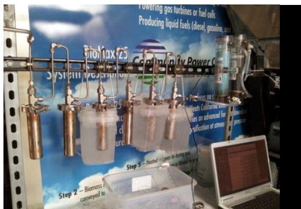
Figure 3.4 Tar collection set up
