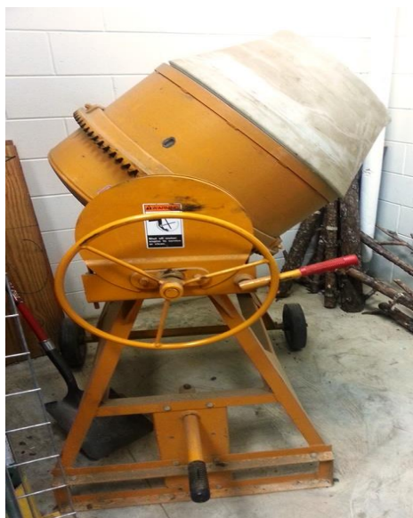
Figure 4.1 Concrete mixer for blending biomass
