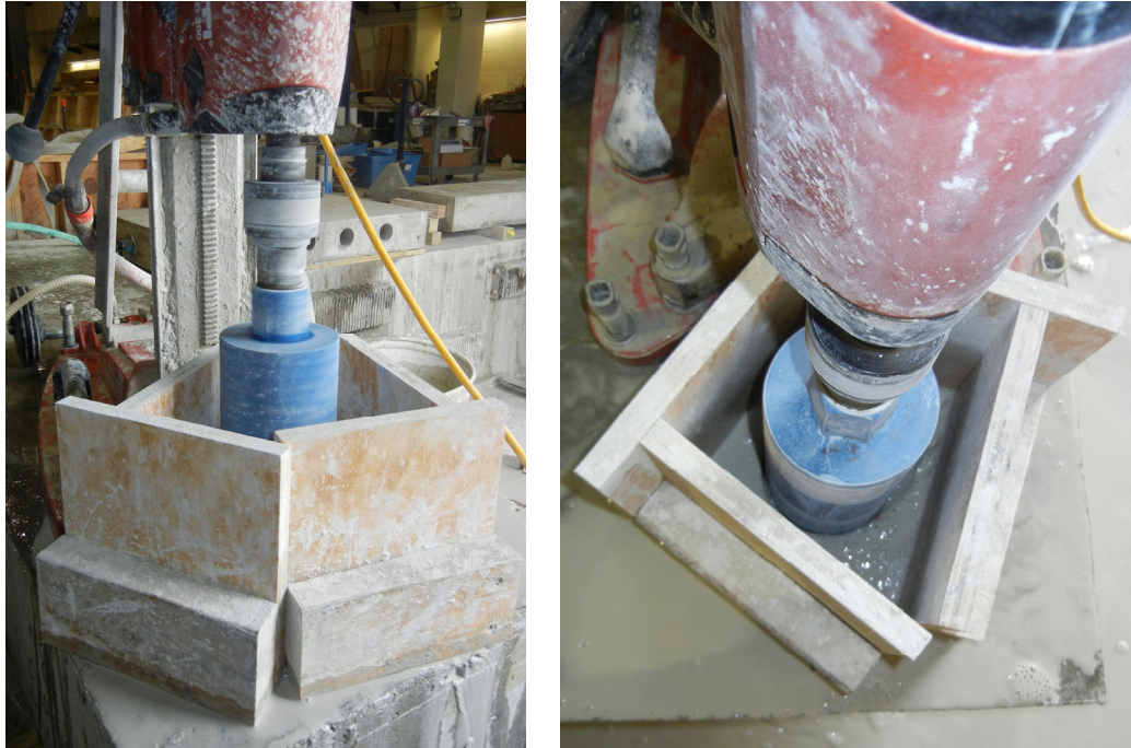
Figure 3-22: Guards used during coring to improve lab cleanliness
