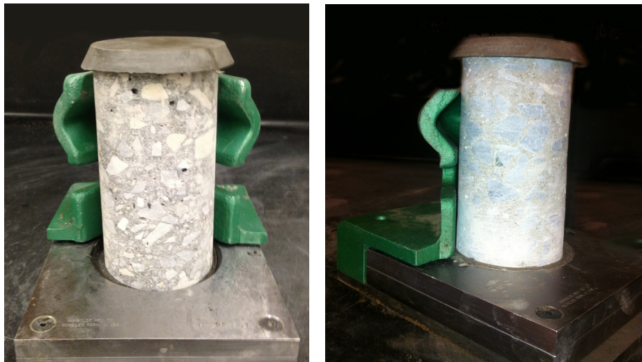
Figure 3-32: Example of sulfur capping
