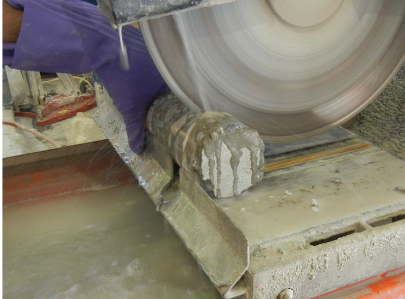
Figure 3-28: Use of wet saw for trimming cores
