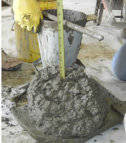
Figure 3-13: Slump for a concrete using HRWRA
