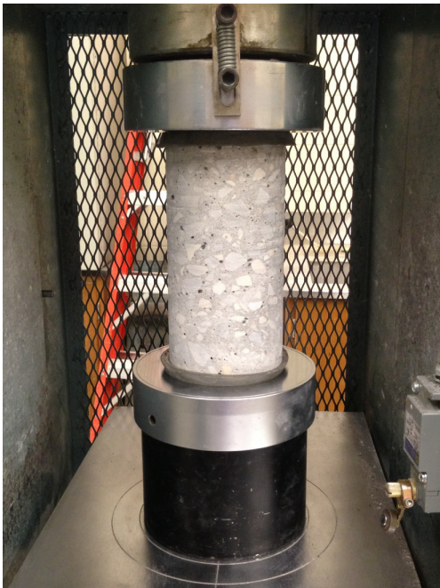
Figure 3-35: Example of 4 x 8 in. core specimen in compression machine
