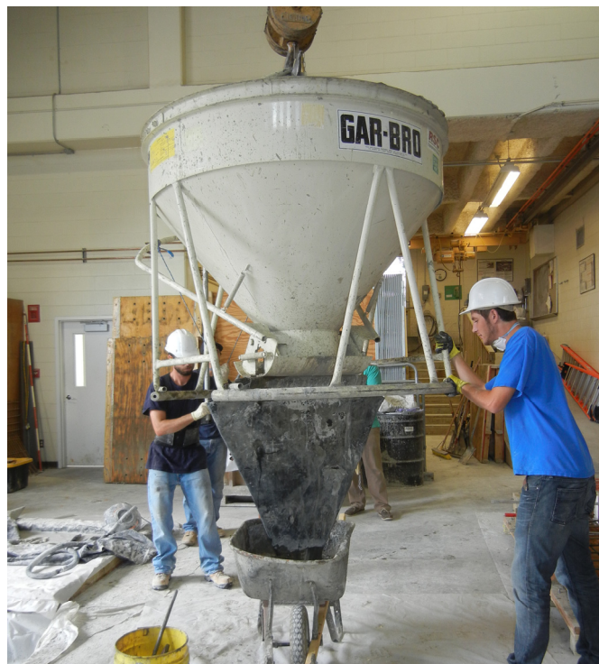
Figure 3-15: Placing concrete into wheelbarrow for sampling
