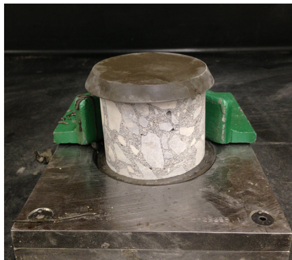
Figure 3-33: Modified capping stand for short cores
