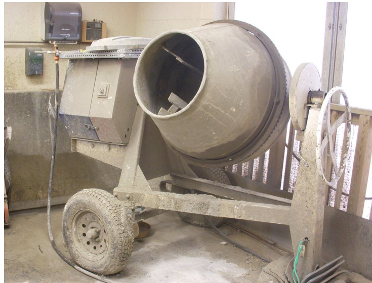
Figure 3-11: Concrete mixer used for in-lab trial batching
