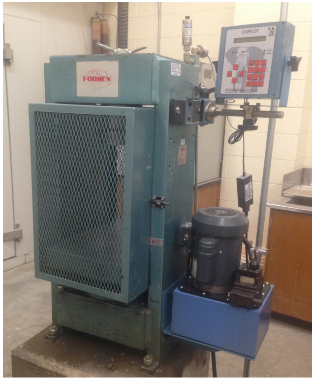
Figure 3-34: Forney compression machine used for testing
