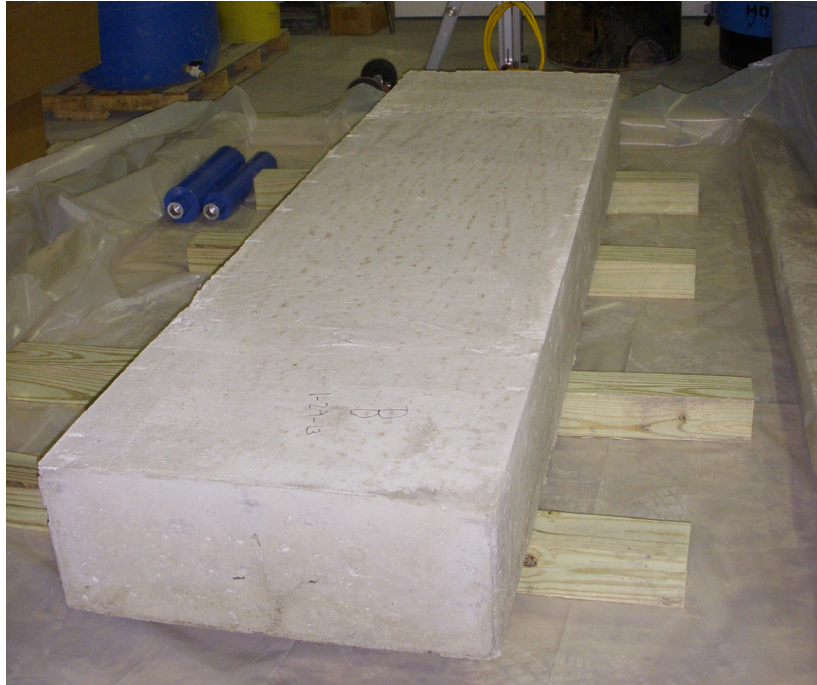
Figure 3-21: Slab setting over coring bath
