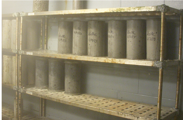
Figure 3-16: Cylinders (6 x 12 in.) in moist-curing room
