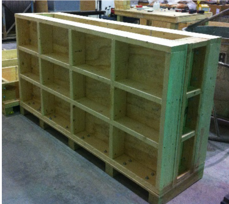
Figure 3-6: Constructed form for wall specimen
