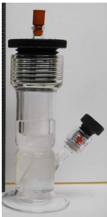
Image 3-2. Illumination vessel for the reduction of Cr(VI) in SPEEK/PVA films.
