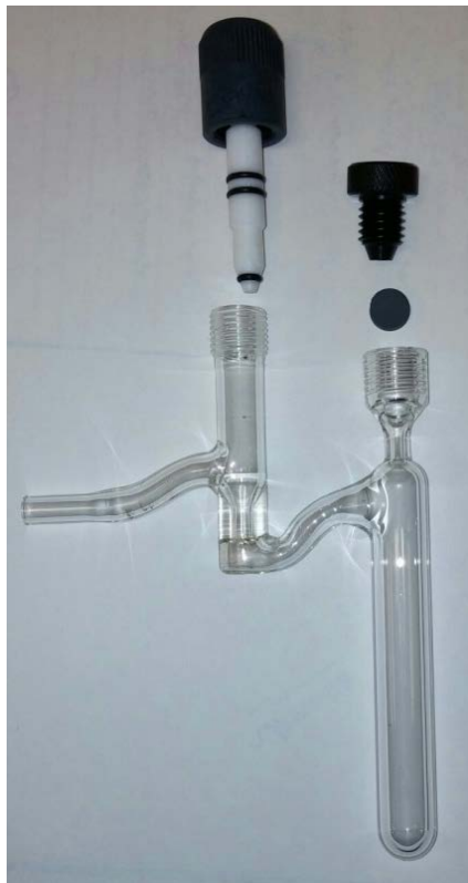
Image 4-2. Illumination vessel used for photolysis of air-free solutions. Degassing was accomplished via freeze-pump-thaw cycles.
