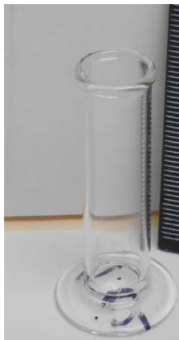
Image 3-1. Illumination vessel used for the reduction of Cr(VI) in polymeric solutions.
