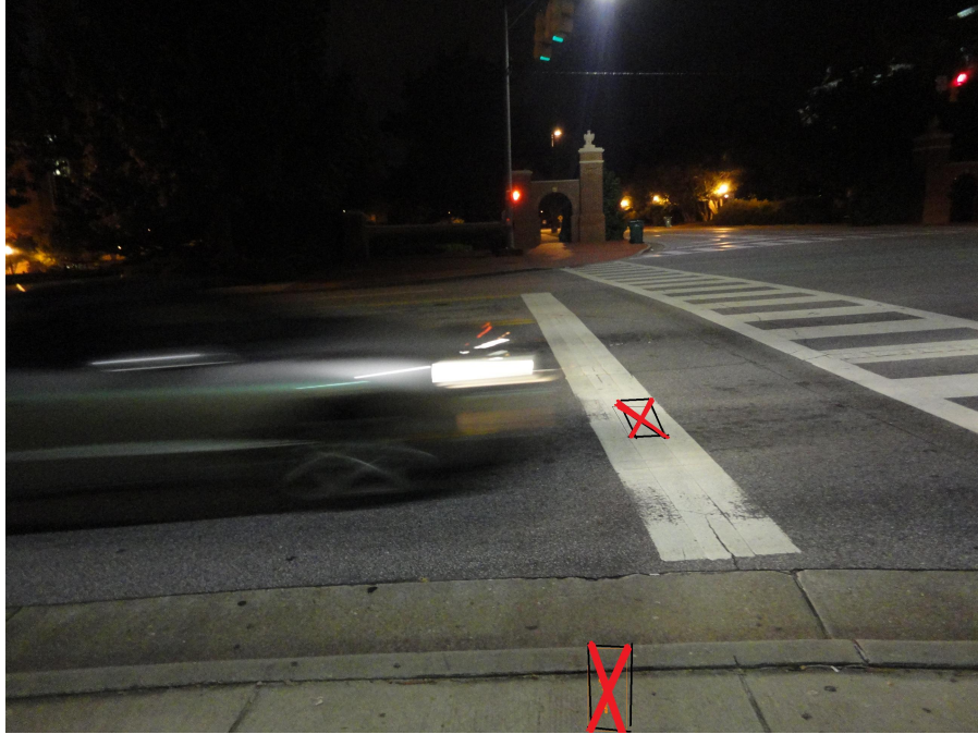
Figure 3.4: Experiment setup positions at traffic light - “X” marks positions the red x-signs. The traffic light measurements provided the opportunity to observe actual situations of slowly-moving or stalled/stopped vehicles.
