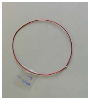
Figure 4.1 Example of a q-coil (5 inch copper loop with 18 AWG copper wire)
