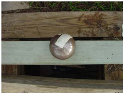
Figure 4.7 Picture of the 4 inch Carbon Steel Sphere from the Pit testing
