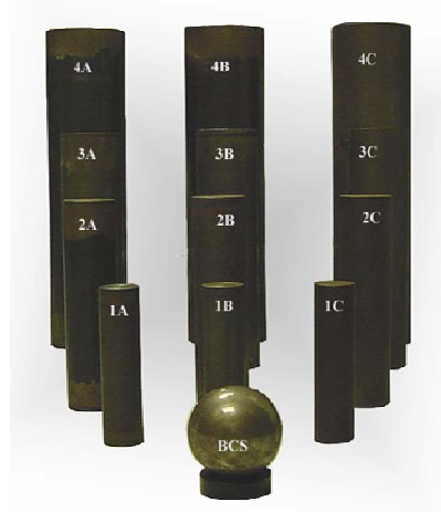
Figure 4.3 UXO test objects consisting of 12 cylinders outlined in Table 4.1
