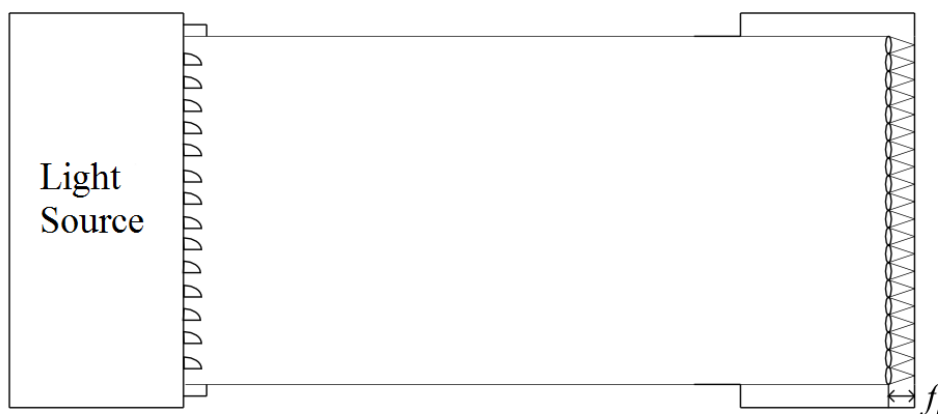
Figure 2.14: The process of aligning the microlens array.
