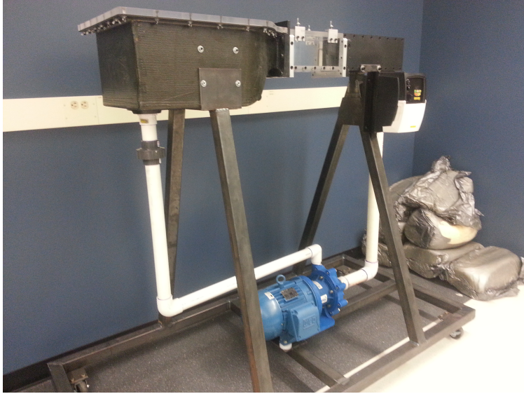
Figure A.2: Current appearance of Auburn University water tunnel
