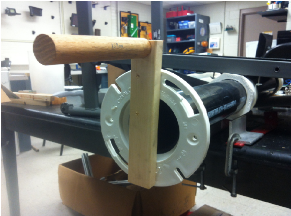
Figure A.5: Manual conveyor belt driver using a ABS pipe
