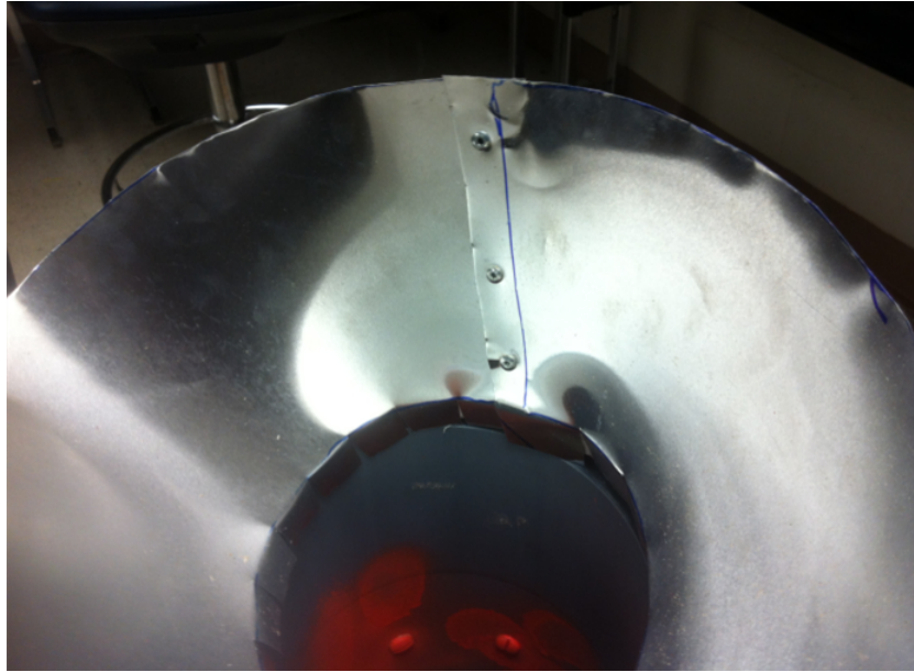
Figure A.10: Aluminium hopper above the ECT
