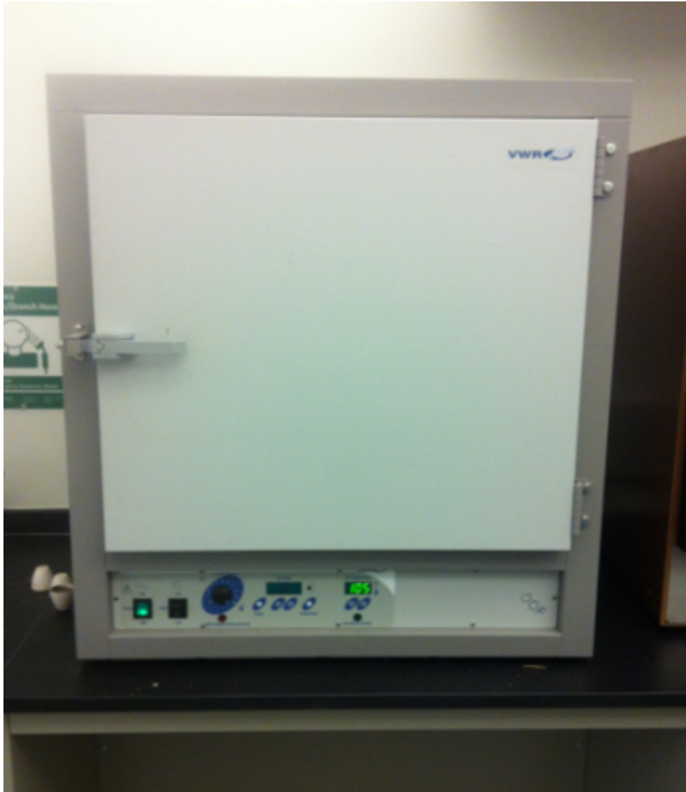
Figure B.4: Oven for woodchips drying
