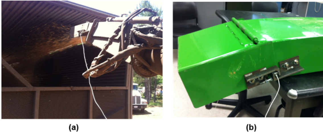
Figure 5.2: Hinged element as used in measuring impact force of chips ejected from a chipper. The left image shows the modified chute in place, and on the right a close-up view of the sensing element.
