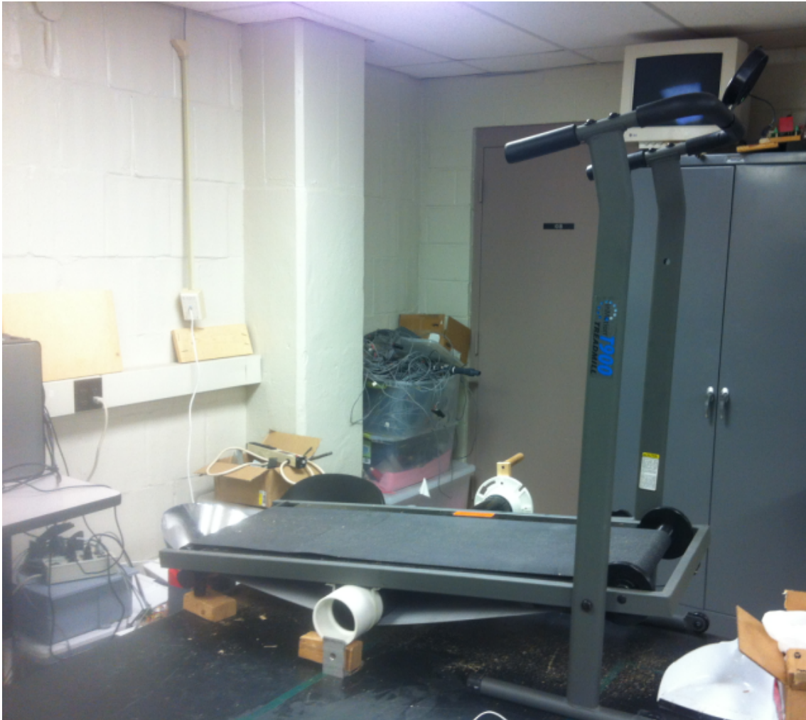
Figure A.6: Mechanical treadmill used as woodchips feeding system
