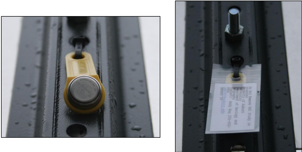
Figure 3. iButton installation on the back of a street sign. The photo on the left is the iButton in the bracket without the id tag. The photo on the right is the iButton in the bracket with the id tag.
