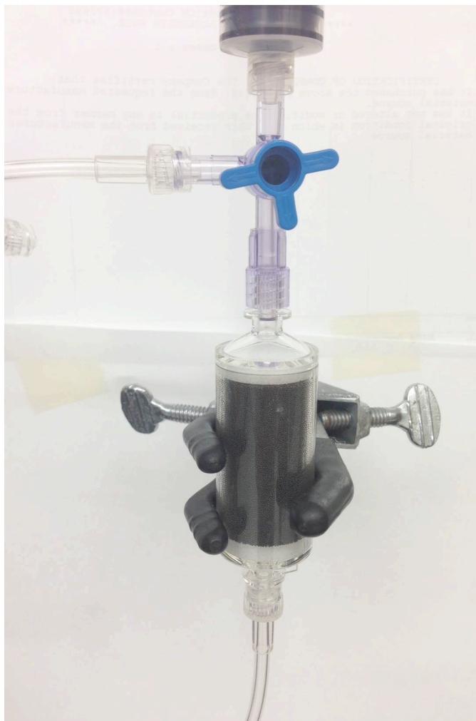
Figure 4.1 Digital image of the proposed magnetic field-flow fractionation device composed of a column packed with magnetic beads.
