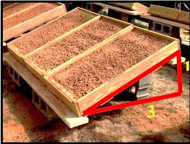
Figure 3.7: Test plots placed on 3:1 slope using concrete blocks and lumber
