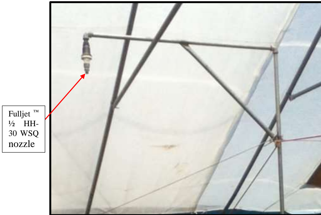
Figure 3.11: Portable galvanized steel rainfall simulator with sprinkler nozzle
