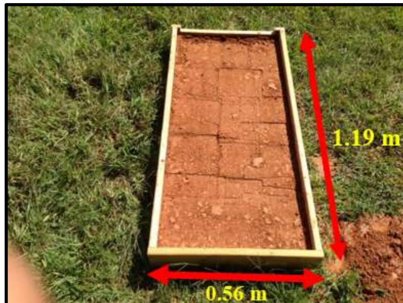
Figure 3.6: Soil filled and compacted small scale test plots
