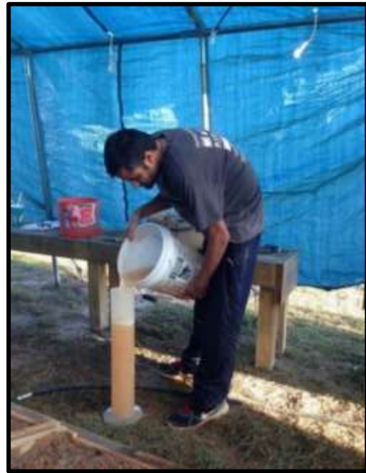
Figure 3.21: Pouring the filtered water into graduated cylinder to measure runoff volume, TGRU, Auburn, AL
