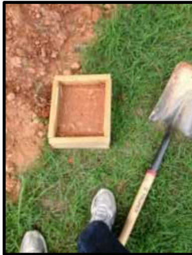
Figure 3.9: Mold box (25.4 cm x 25.4 cm) used to determine required tamps to achieve a field bulk density of 0.9 \text{ g cm}^{-3}
