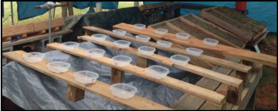
Figure 3.12: Placement of catch cans over test plots during uniformity testing, TGRU, Auburn, AL
