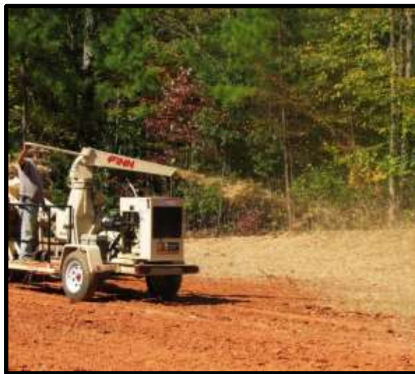
Figure 3.14: Wheat straw application by straw blower as performed in a commercial application
