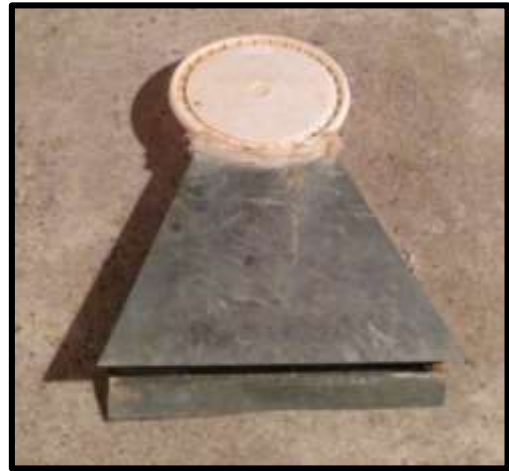
Figure 3.8: Flumes to direct runoff from test plots into collection buckets
