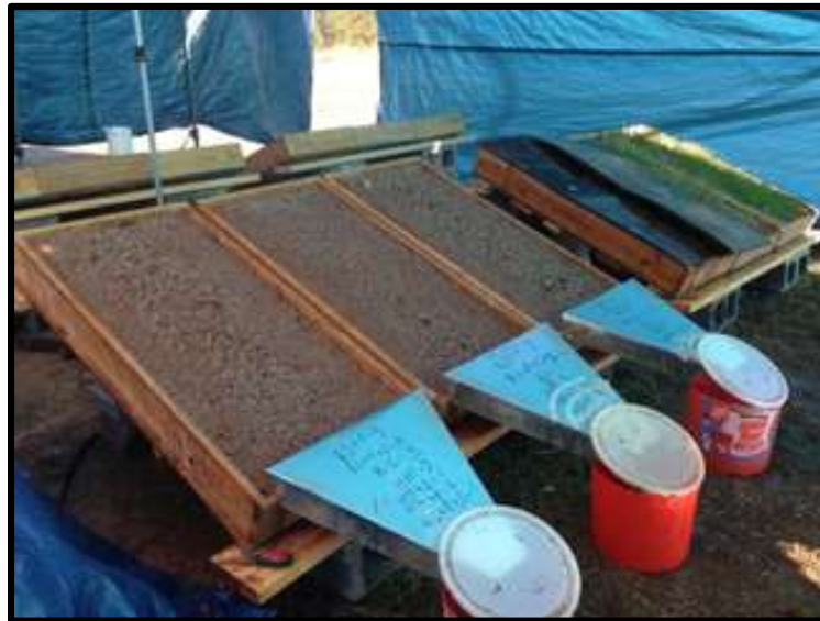
Figure 3.19: Collection of runoff from the test plots, TGRU, Auburn, AL
