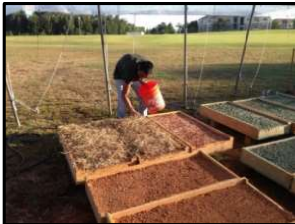
Figure 3.15: Wheat straw application by hand at the ASWCC recommended rate of 4480 kg ha -1 , TGRU, Auburn, AL
