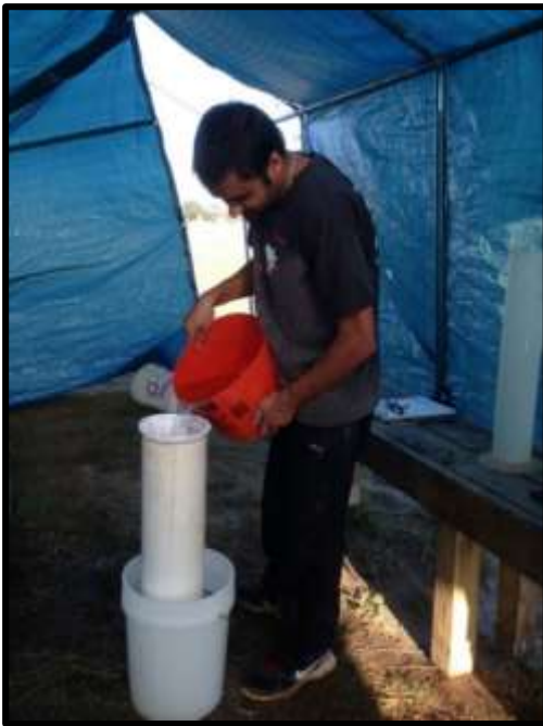
Figure 3.20: Pouring the sediment water into the filter bags, TGRU, Auburn, AL
