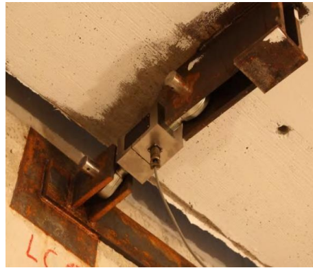
Figure 4-25 Single-Span Top Connection Detail (Naito et al. 2011)
