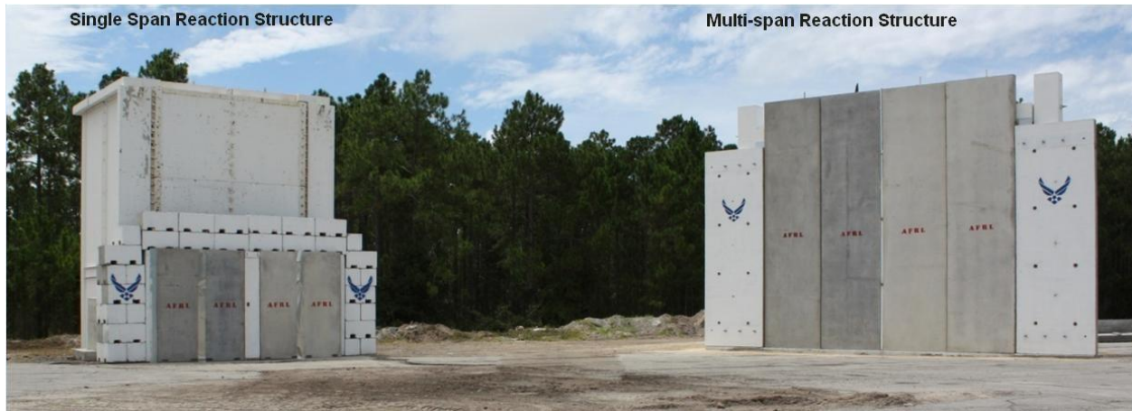
Figure 4-19 Test Set Up for Full-scale dynamic tests with single span reaction structure (left) and multi-span reaction structure (right)
