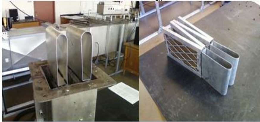
Figure II-31. Picture of two round-top fairings added to the pleat tip of microfibrous media filter; fairings at upstream when running tests
