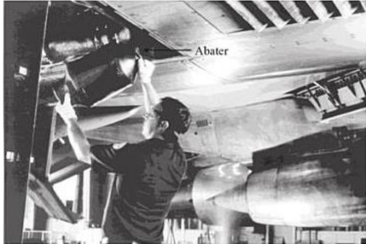
Figure I-4. Installation of ozone converter on a commercial jet aircraft
