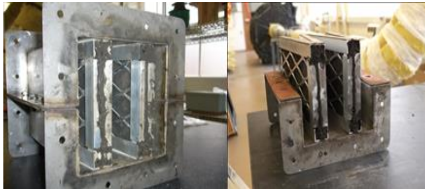
Figure II-25. Picture of no fairings added to the pleat tip of microfibrous media filter; fairings at upstream when running tests
