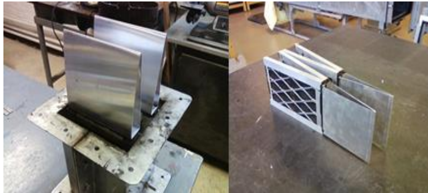
Figure II-37. Picture of two triangle fairings added to the pleat tip of microfibrous media filter; fairings at upstream when running tests
