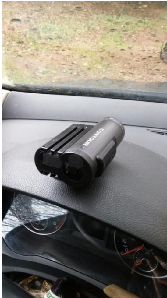
Figure 6: Photo of Contour +2 geospatial video camera mounted to dashboard
