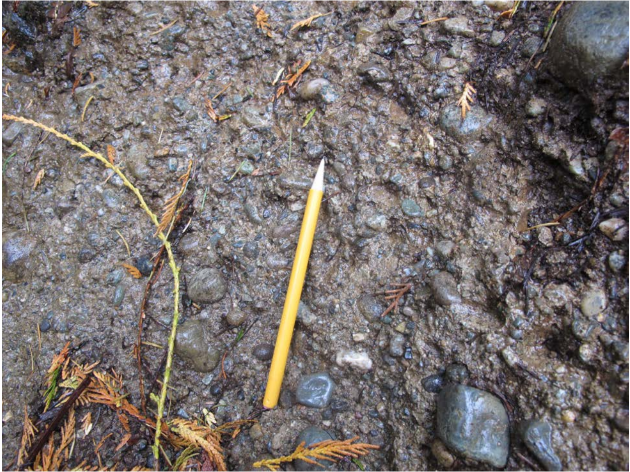
Figure 6. Photograph of semi-cemented rounded cobbles and pebbles typical of a Glacial till deposit within the Muckleshoot basin.
