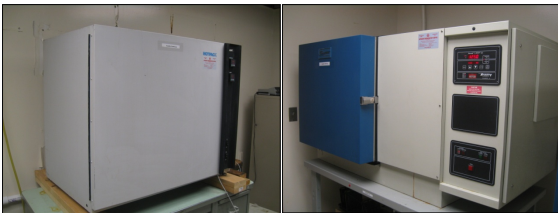
Figure 3.20 Humidity Chambers Used for Moisture Exposure
