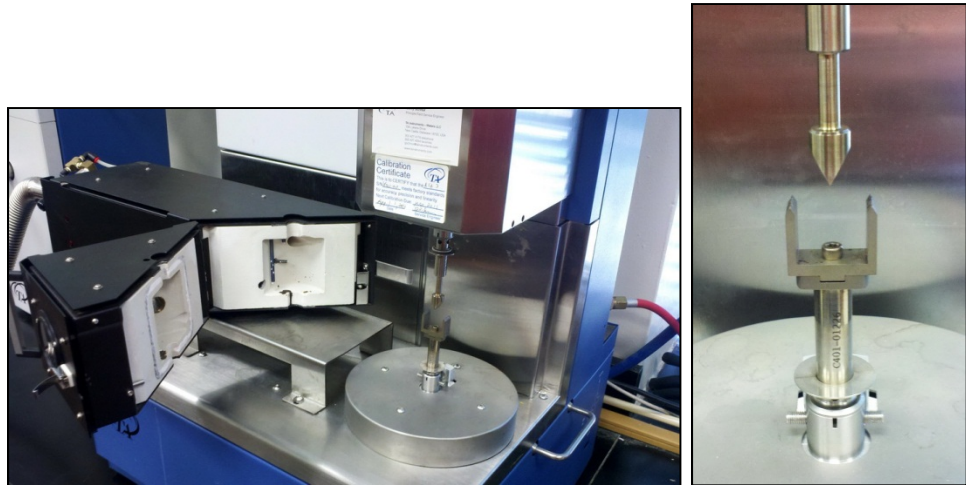
Figure 3.16 TA Instruments RSA3 DMA System
