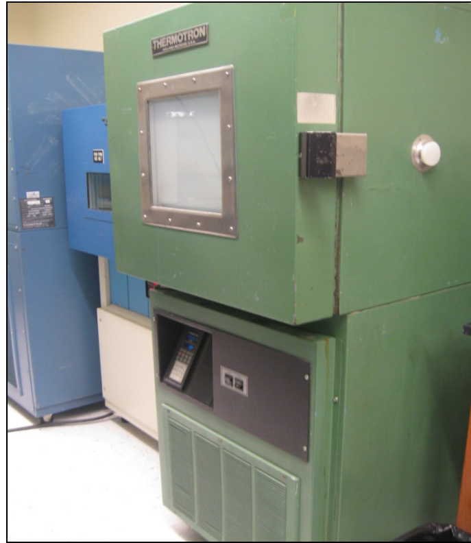
Figure 3.5 Thermal Cycling Chamber
