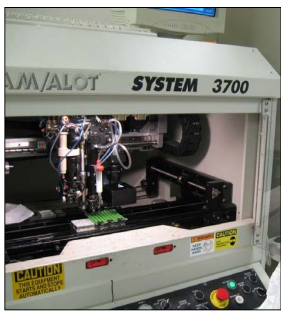
Figure 3.2 Specimen Preparation Machine and Mold Assembly
