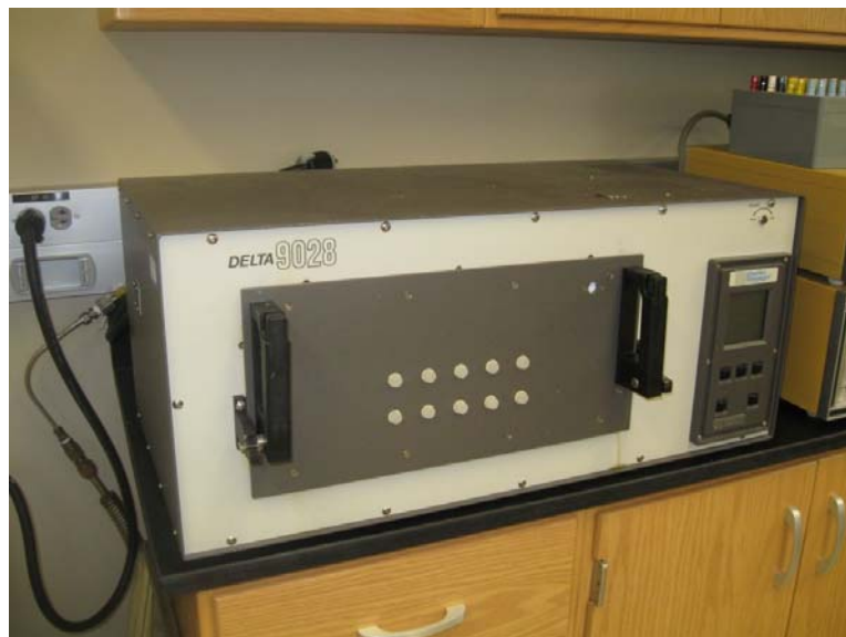
Figure 3.3 Box Oven for Curing
