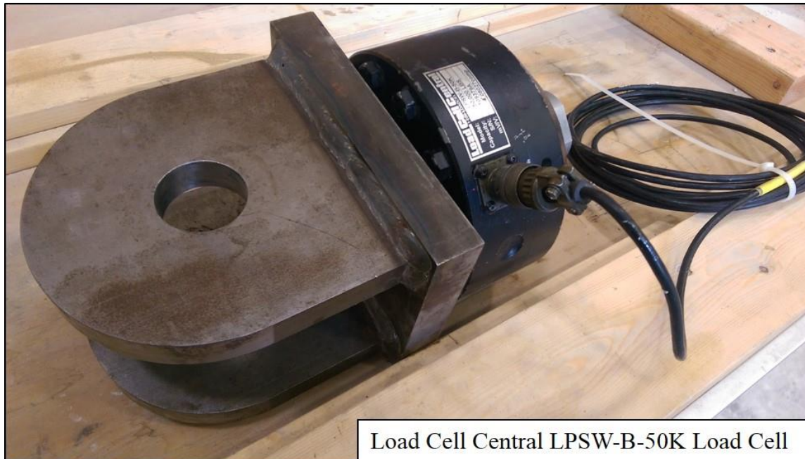
Figure 4-33. Load Cell with Attached Damper Clevis
