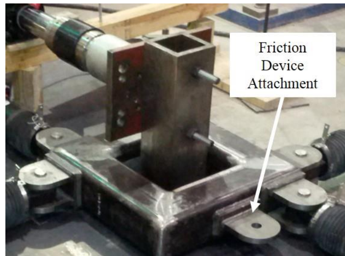
Figure 4-17. Two-Phase Viscoplastic Bumper System
