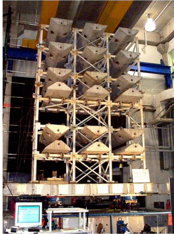
Figure 2-13. Six-Story Base Isolated Model Structure (Wolff & Constantinou, 2004)
