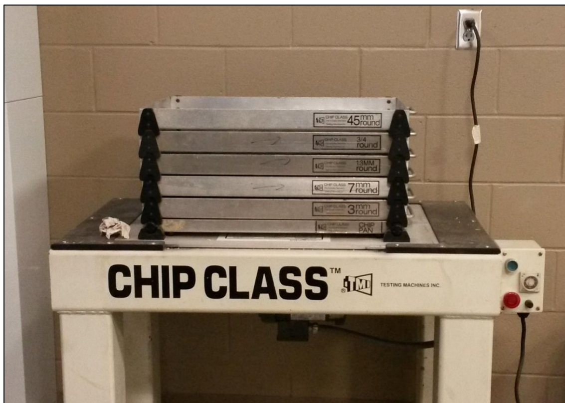
Figure 3.1. TMI woodchips classifier used for woodchips particle size distribution measurement.
