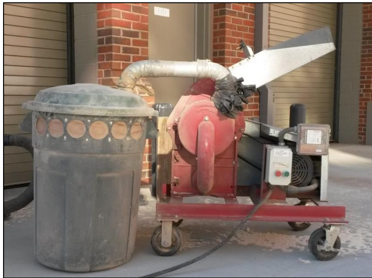
Figure 3.2. C.S. Bell Co. hammer mill used for grinding of woodchips.
