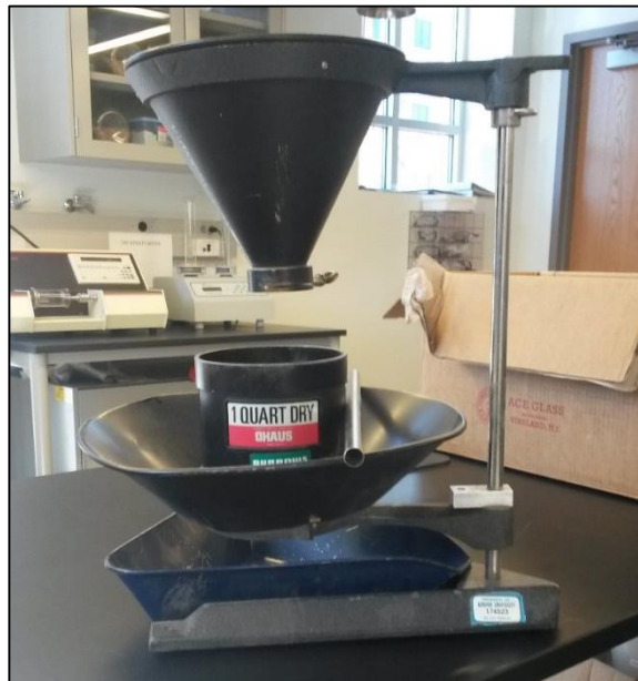
Figure 3.4. Apparatus used for bulk density measurement.
