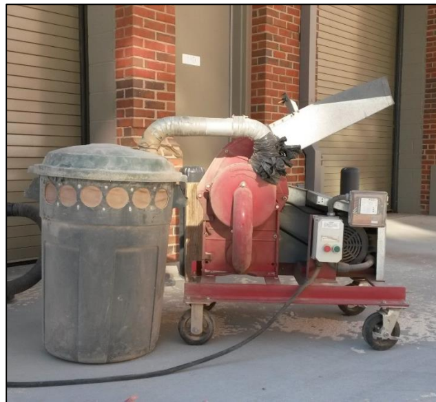
Figure 5.1. C.S. Bell Co. hammer mill used for grinding experiments.
