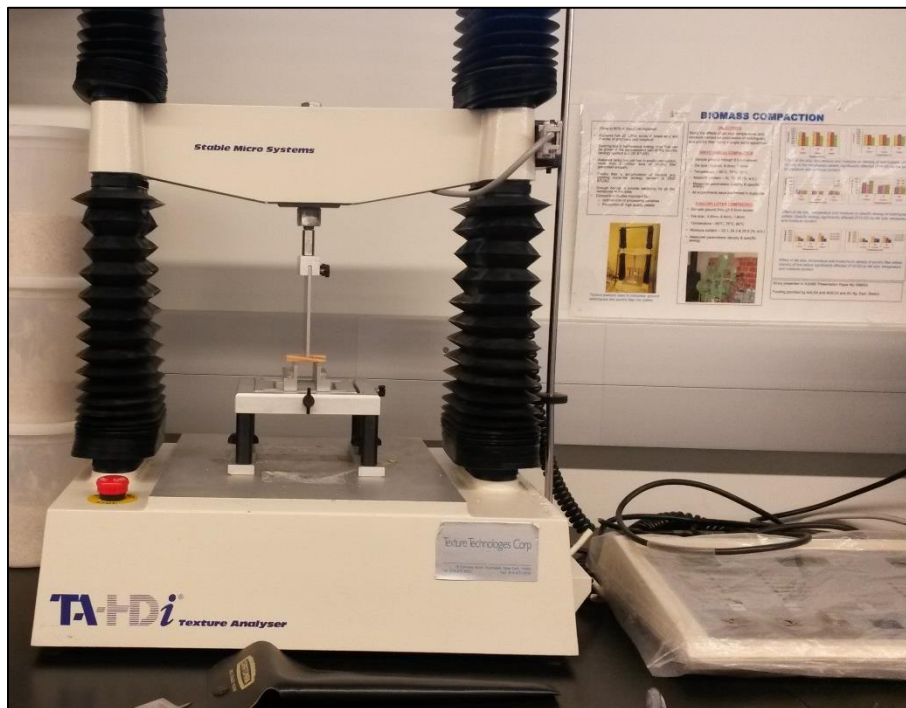
Figure 4.2. Texture analyzer used for three point bending test.
