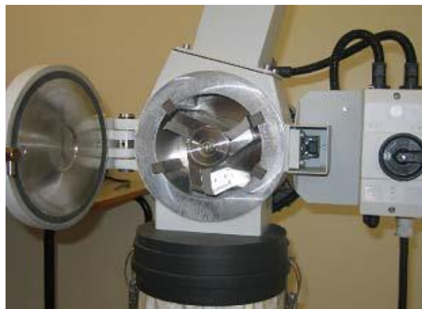
Figure 2.4. A typical knife mill (Naimi, 2008).
