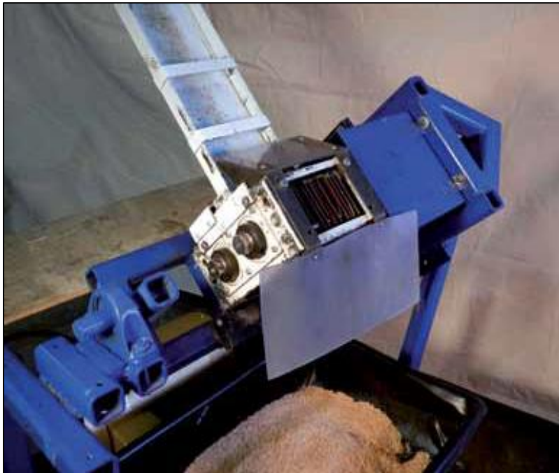
Figure 2.5. Forest Concepts laboratory crumbler (Dooley et al., 2013).
