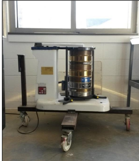
Figure 3.5. W.S. Tyler Ro-Tap sieve shaker used for particle size distribution measurement.
