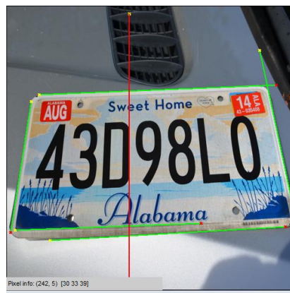
Figure 11. Hough Lines Covering 4 Sides of the Tag
