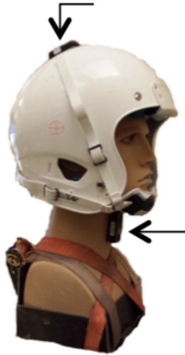
Figure 38 G-Force Tracker mounting locations on headform
