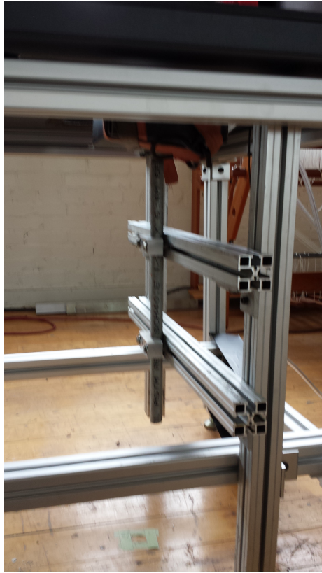
Figure 34 Rod attachments to cannon frame
