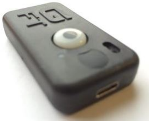
Figure 37 Tri-axial G-force Tracker accelerometer
