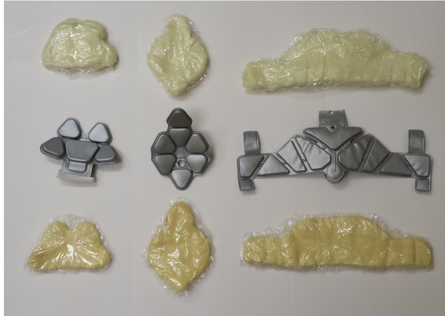
Figure 42 Padding shapes (Top: New ST Trauma Reducing Fabric, Middle: Schutt TPU Padding, Bottom: Old Kevlar Trauma Reducing fabric)
