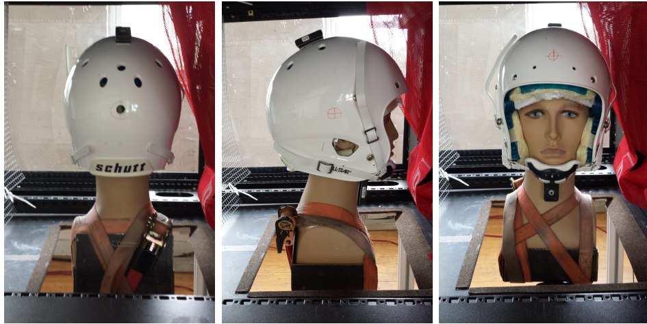
Figure 40 Impact locations (Left: Rear, Middle: Side, Right: Front)
