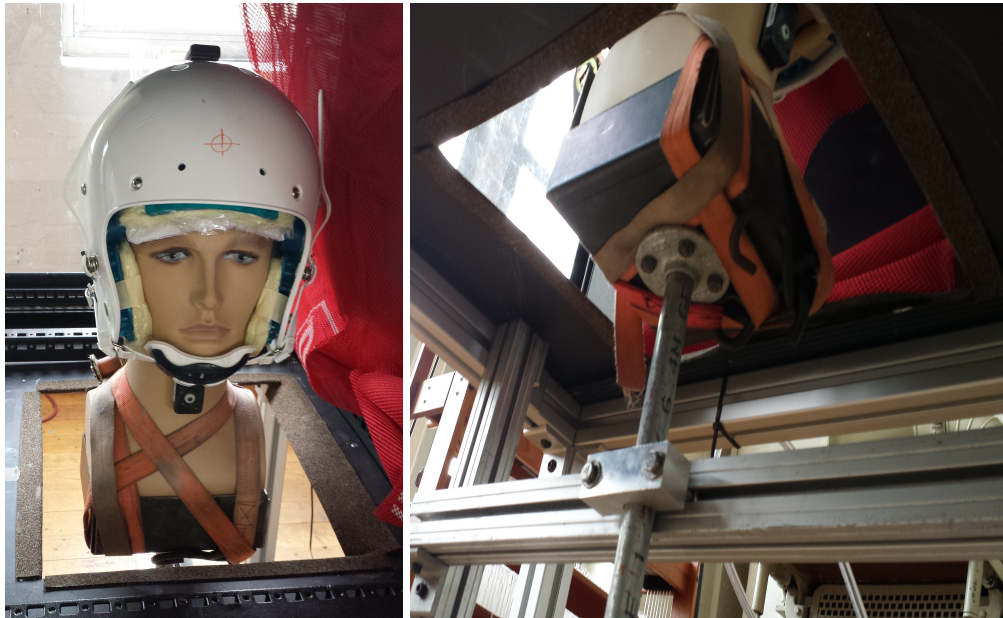
Figure 35 Headform attachment to rod
