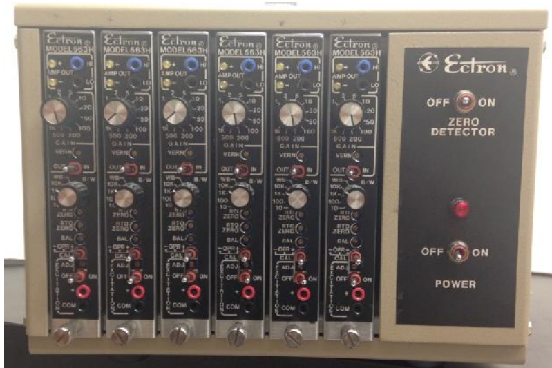
Fig. 2.5: Photograph of the Ectron 563H amplifier used to amplify the strain gage signal on the long-bar.
