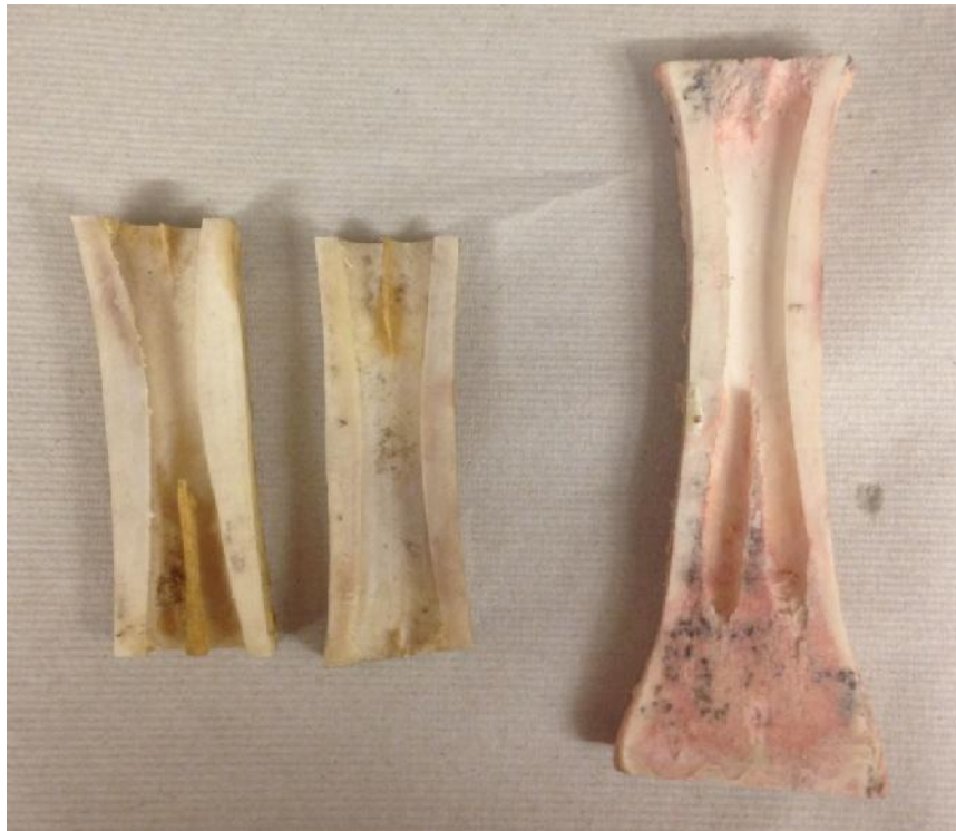
Fig. 4.3: Posterior portion of bovine cortical bone after axial slicing. Dynamic fracture specimens (Fig. 4.4) were milled from the central region.
