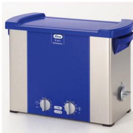
Fig. 5.23: Elmasonic E60H ultrasonic cleaner from Elma Ultrasonics used for simultaneous bath sonication and mechanical stirring. 25
