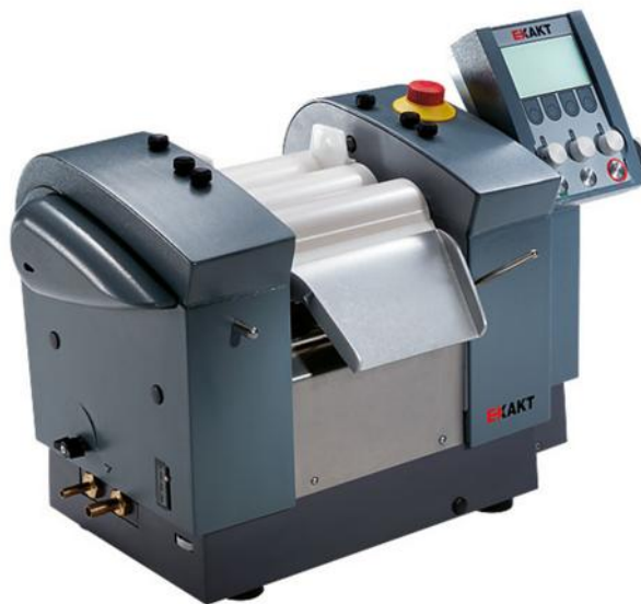
Fig. 5.21: Exakt 80E calender used to disperse relatively large quantities of nanomaterials. 23
