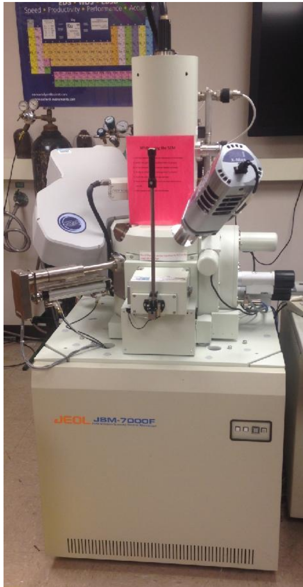
Fig. 3.19: JEOL JSM-7000F used to generate SEM images.
