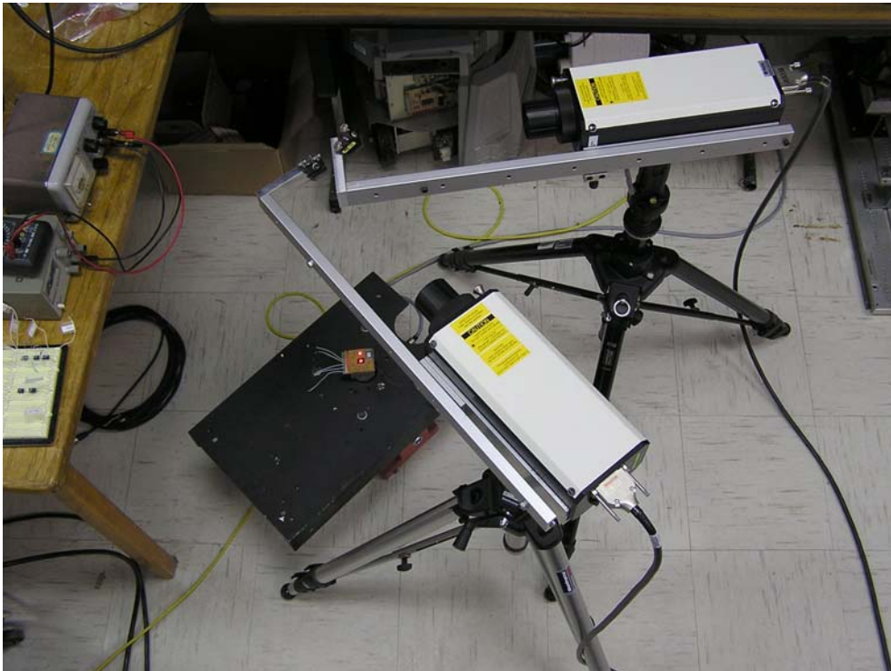
Figure 5.4. A photograph of the shaker and the two Polytec laser systems.
