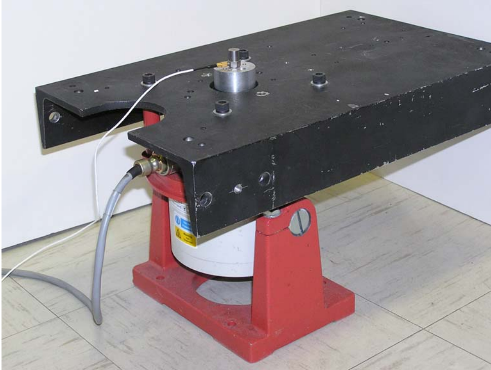
Figure 5.2. A photograph of the electromechanical shaker used in evaluating the prototype relative velocity sensor.
