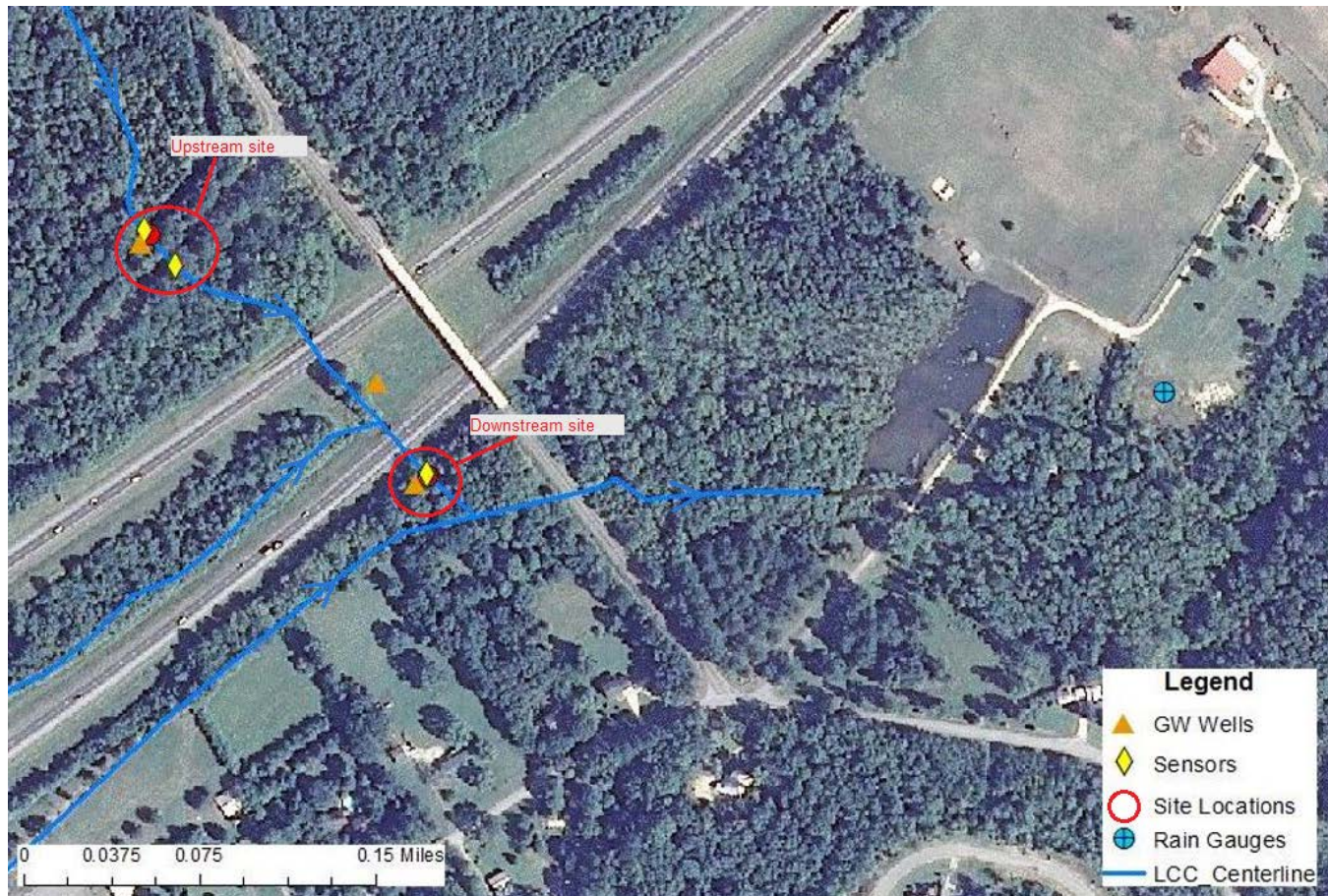
Figure 3.3: LCC Upstream and Downstream Sensor Locations for Area Velocity Sensors, Auto-Samplers, Water Quality Sondes, Hobo level Loggers (used in groundwater wells); Rain Gages.
