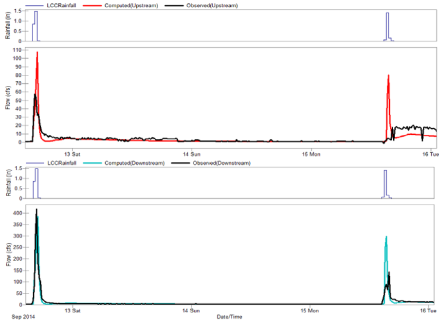
Figure 4.13: Flow hydrograph comparison for upstream (top) and downstream (bottom) simulated and respective measurements (9/12/2014).
