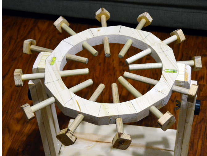
Figure 15: Capturing the stump cross-section contours
