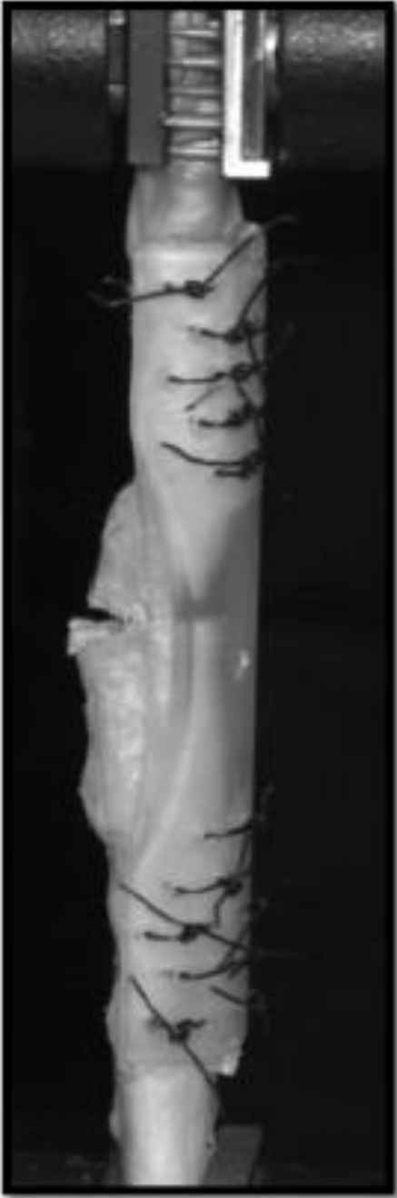
Figure 38: Bioabsorbable Poly-L-Lactic acid tendon plate (Jenson 2005). Figure used under Fair Use guidelines.
