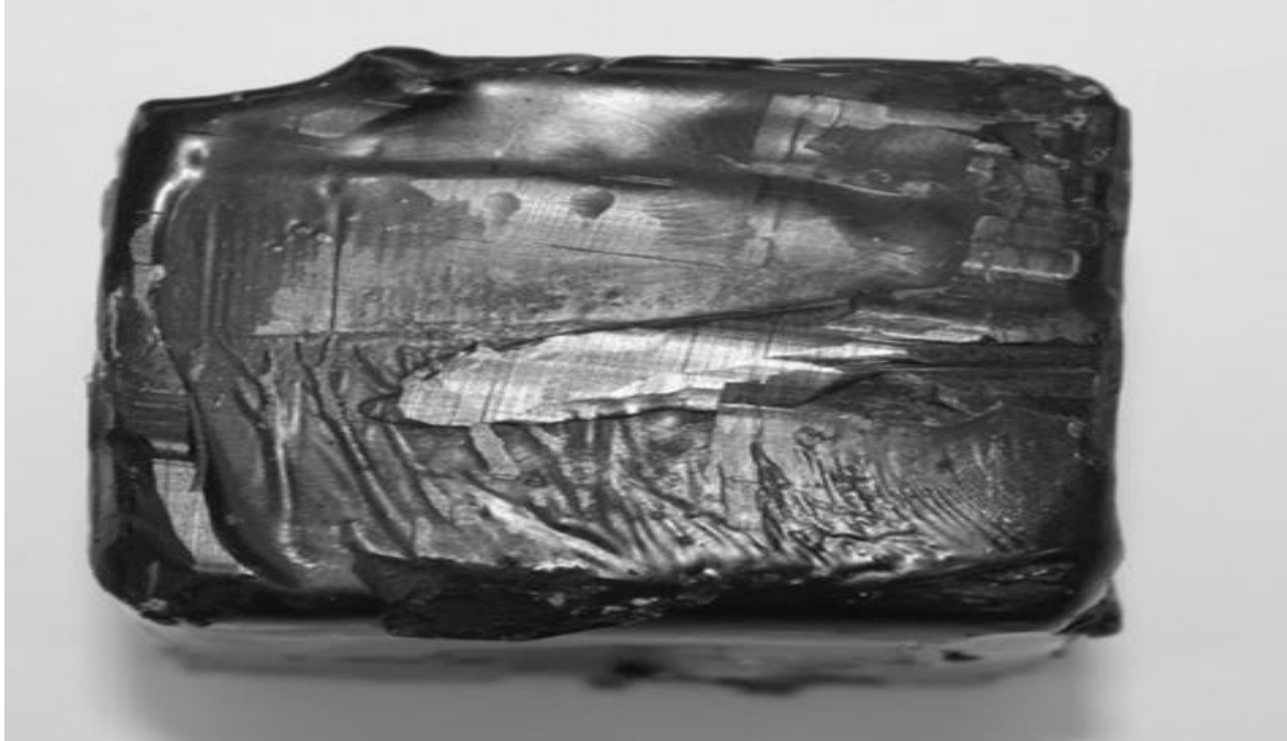
Figure 2.8 Image of a 5 wt% GNF/PCM sample with 30% added HDPE after 10 thermal cycles (Ehid et al., 2012)
