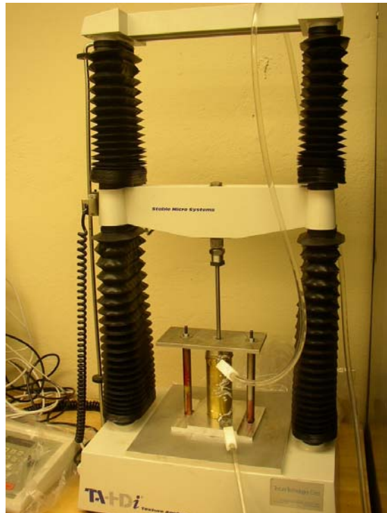
Figure 3.1- Single pellet compaction test set up
