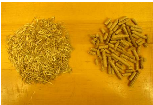
Figure 2.3 – Ground (3.18 mm screen) and pelleted switchgrass (4.76 mm diameter)
