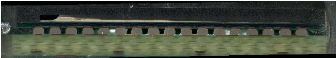
Figure 56: K6H-series SEM solder ball image (100X)
