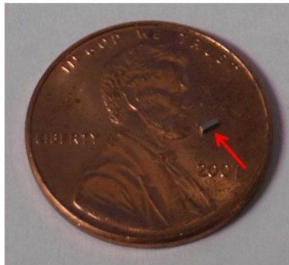
Figure 2.7: A 1500 \mu\text{m} X 500 \mu\text{m} X 500 \mu\text{m} NdFeB magnet like the ones used in the second MEMS current sensor prototype and the final MEMS current sensor design.
