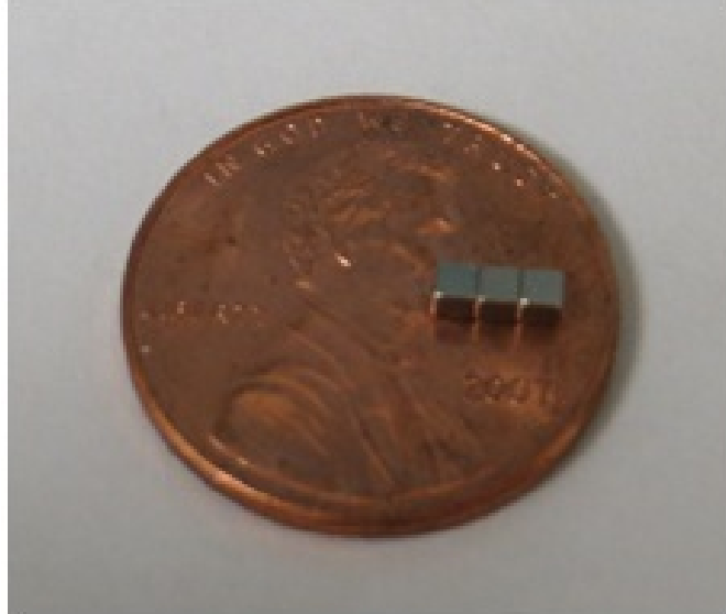
Figure 2.3: The assemblage of three NdFeB magnets used in the prototype current sensor as compared to a U.S. penny. The magnets each measure 1.6 mm X 1.6 mm X 1.6 mm, with three of them stuck together forming an effective 4.8 mm X 1.6 mm X 1.6 mm magnet magnetized in the long dimension.
