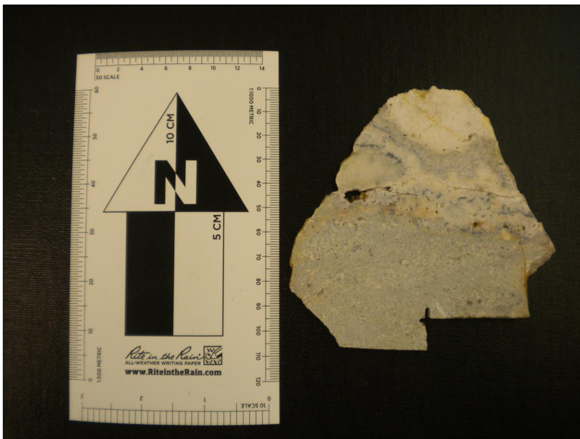
Figure 12: Photograph of an ore sample from the Trade Dollar Mine showing the gold-poor altered granite sample (chip was cut off the bottom of the sample) and the gold-rich mineralized vein less than 5 cm away.
