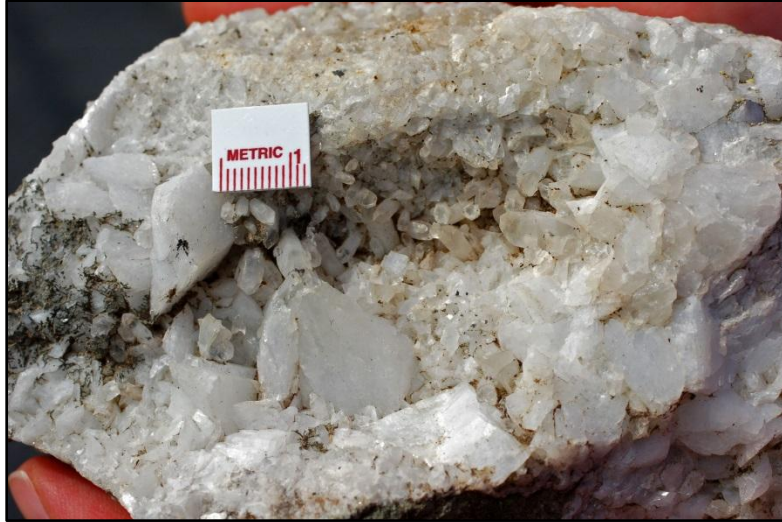
Figure 28: Photograph of a hand sample showing several large crystals of adularia with much smaller quartz grains surrounding them.
