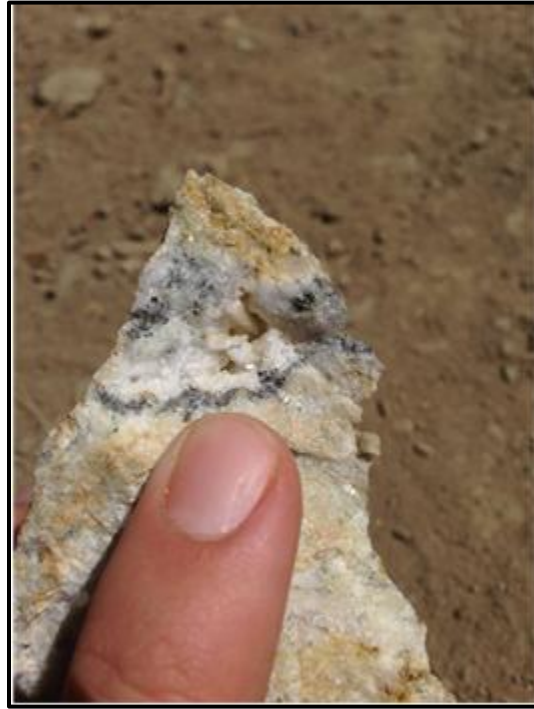
Figure 11: Field photograph showing a finger pointing to the dark ore minerals marking the typical banding present in highest-grade ore samples collected for this study.
