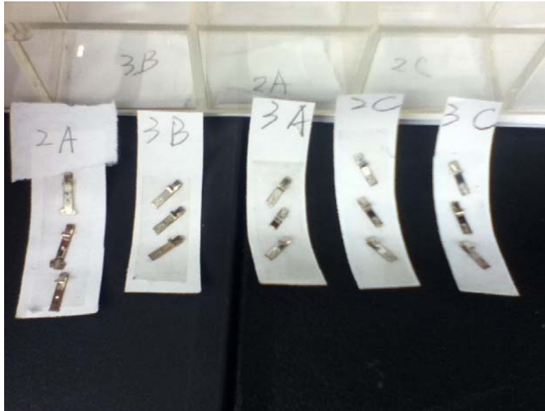
Figure 2-4. Photograph of samples with cut-away to expose receptacle springs
