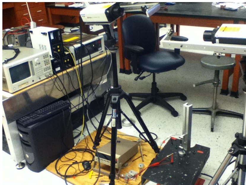
Figure 3-11 Photograph of equipment setup for transfer function test
