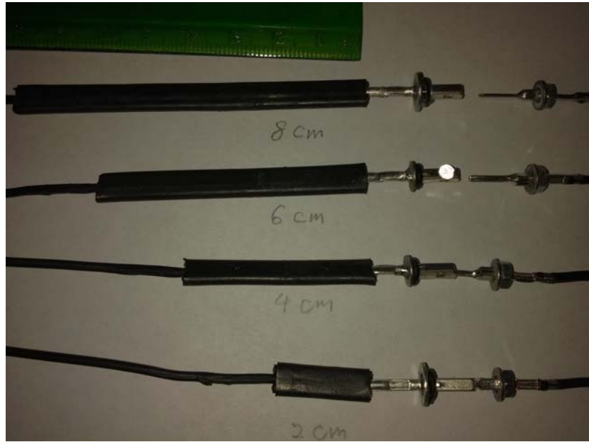
Figure 3-4 Receptacle samples with modified wires joined by thermal shrink tubing
