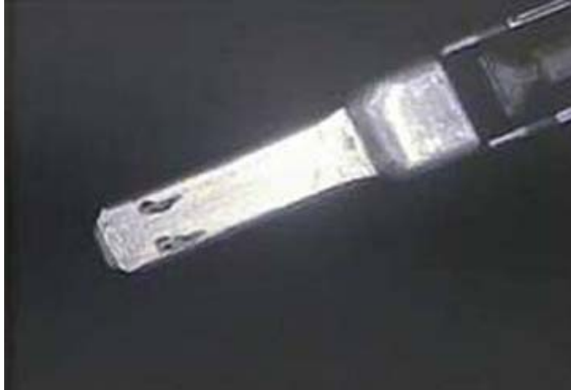
Figure 2-1. Fretting corrosion spot on sample connector blade
