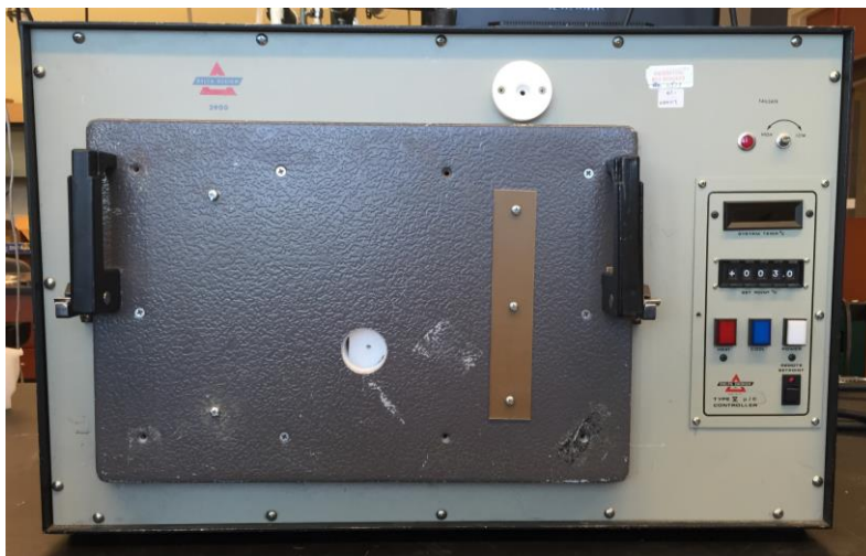
Figure 1 – Temperature controlled oven used for calibration
