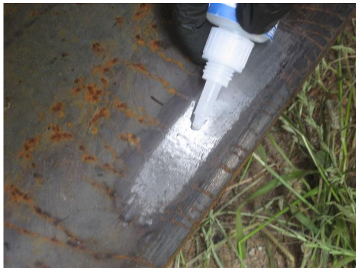
Figure 3-10 Treated Steel Surface Prior to M-Bond Application
