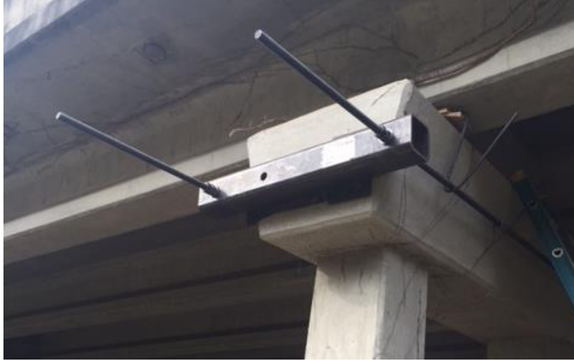
Figure 5-11 End Anchorage at Reaction Bent
