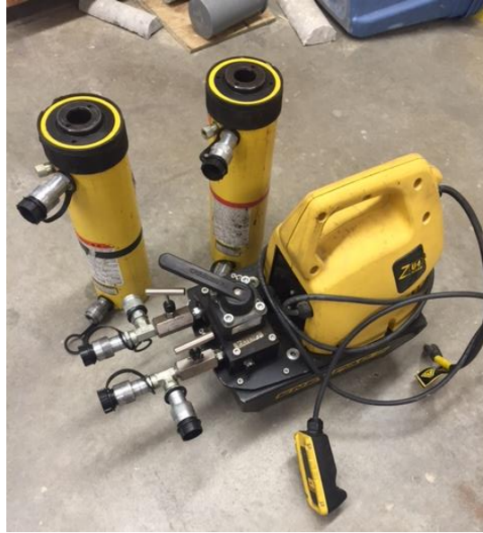
Figure 3-19 Enerpac Center-Hole Hydraulic Cylinders and Pump
