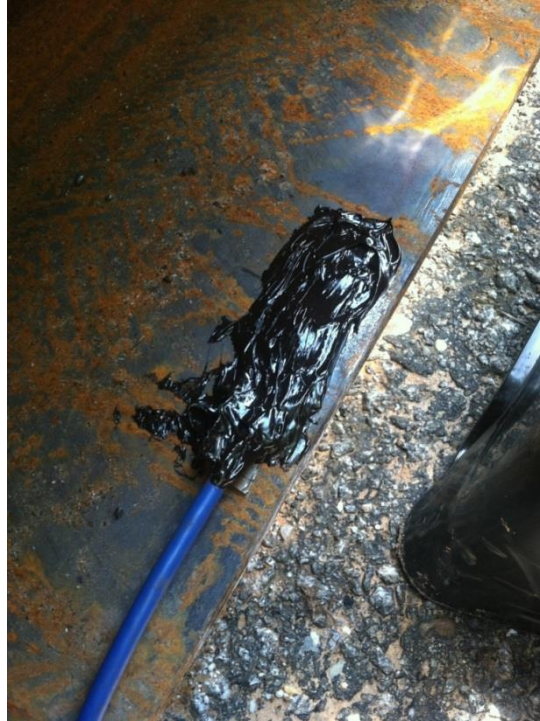
Figure 3-13 Electrical Resistance Gage with M-Coat J Surface Protection
