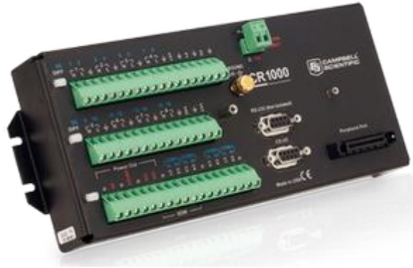
Figure 3-25 Campbell Scientific CR1000 Datalogger (Campbell Scientific 2015)
