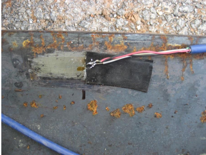
Figure 3-12 Strain Gage with Soldered Connection to Three-Wire Cable
