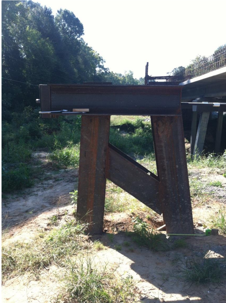
Figure 3-17 Reaction Frame Configuration
