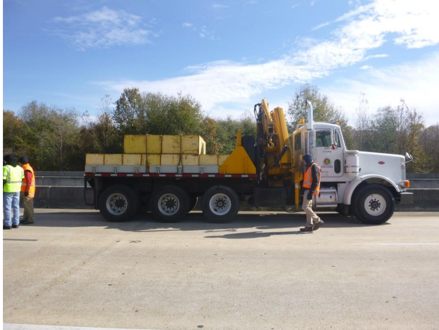
Figure 5-9 ALDOT Load Truck in Configuration LC-5
