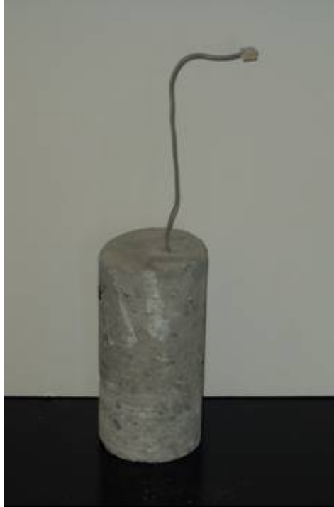
Figure B-94: Core with iButton installed
