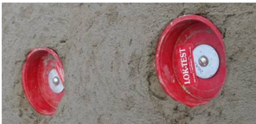
Figure 2-31: Floating pullout inserts
