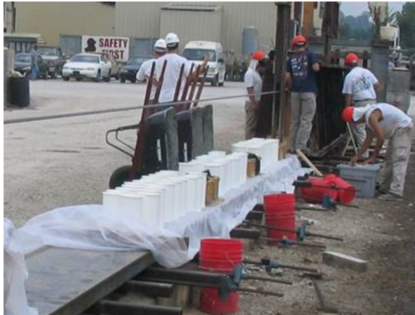
Figure 4-9: Casting of concrete specimens
