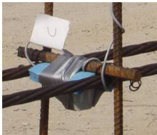
Figure 4-17: iButton attached to a stirrup
