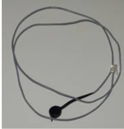
Figure 4-15: Cylinder and cube temperature-recording device
