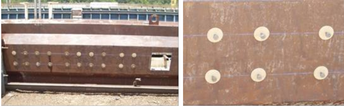
Figure 4-20: Side-mounted pullout inserts on mock girder forms
