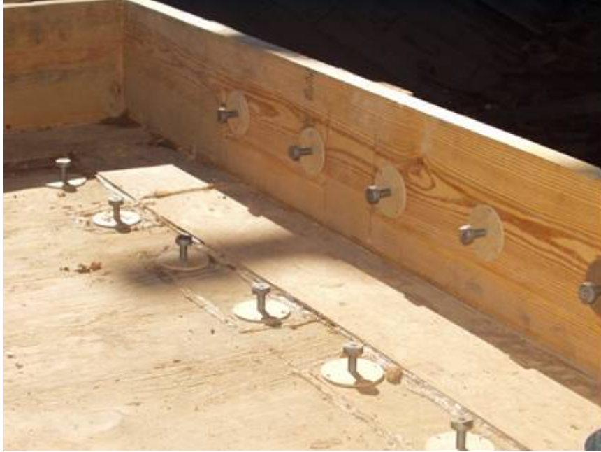
Figure 5-13: Side and bottom pullout inserts
