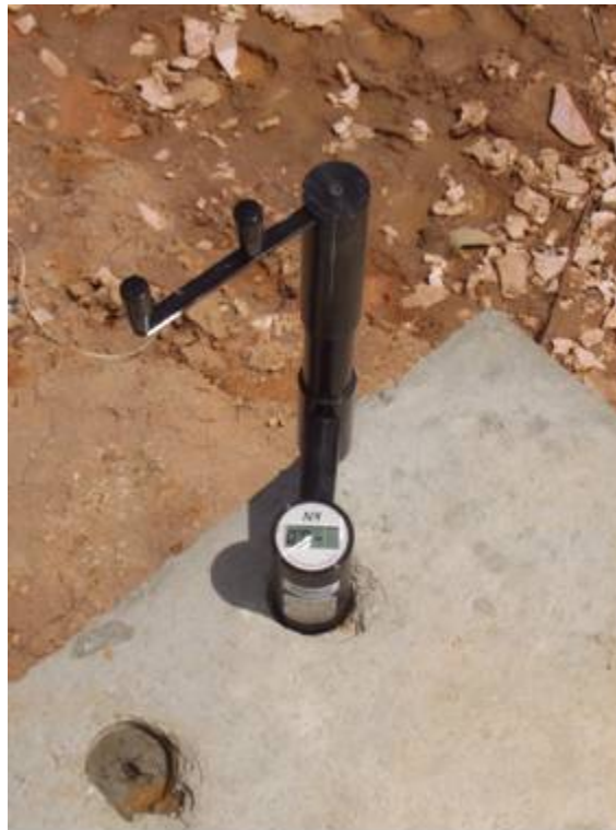
Figure C-111: Pullout testing of top inserts on mock bridge deck
