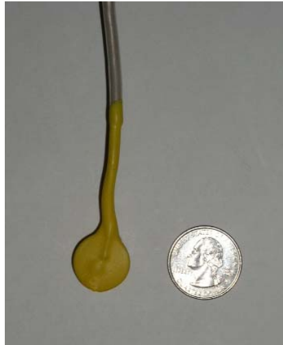
Figure 2-17: The COMMAND Center temperature sensor
