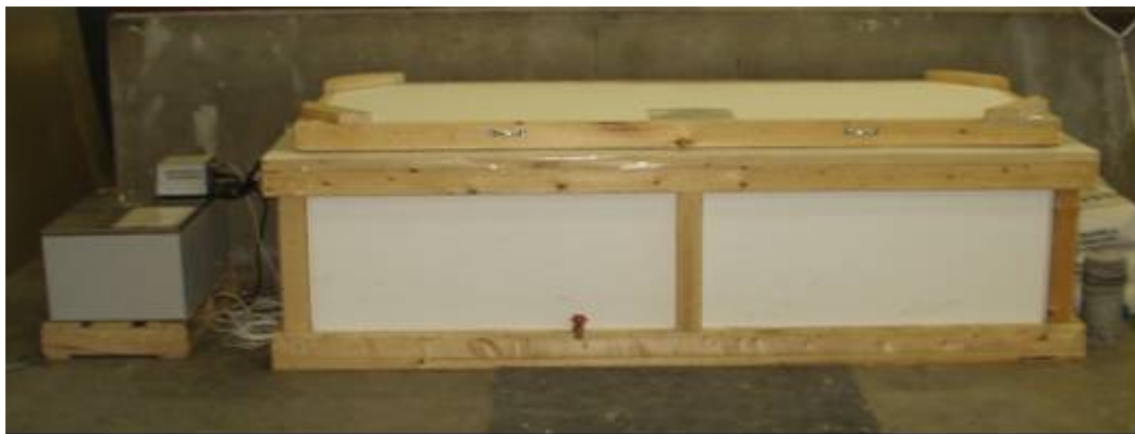
Figure 3-2: Curing tank and programmable heating/cooling circulator
