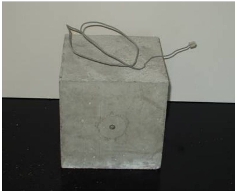
Figure B-95: Pullout cube with iButton installed
