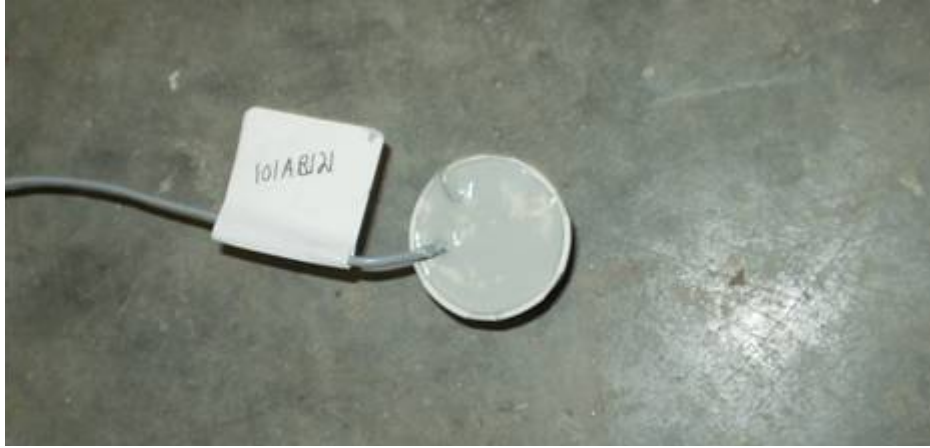
Figure B-96: iButton installed in mock girder
