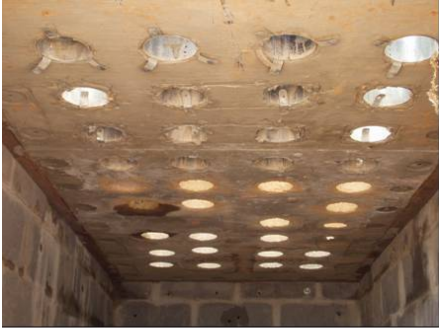
Figure C-112: Bottom view of cast-in-place cylinder and cores for mock bridge deck
