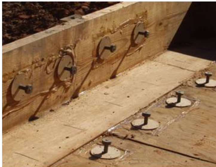
Figure 2-30: Form-mounted pullout inserts
