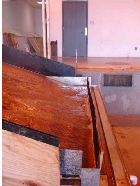
Figure 6.23 Configuration No. 1: Flow Pattern Along the Toe.
