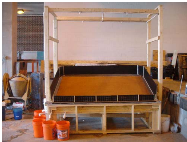
Figure 4.28 Finalized Small-Scale Erosion Control Model.
