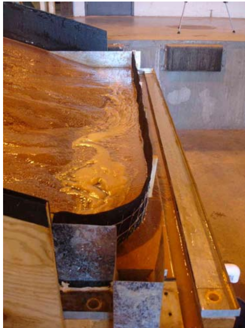
Figure 6.24 Configuration No. 2: Flow Pattern Along the Toe.
