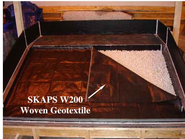
Figure 4.22 Model With SKAPS W200 Woven Geotextile Fabric.
