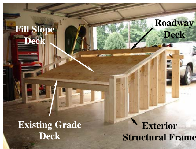
Figure 4.8 Structural Frames and Decking.
