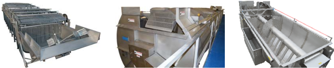
Figure 1. Immersion chillers: drag chiller (left), auger chiller (middle), rocker chiller (right). Photos courtesy of Morris and Associates, Inc. Garner, NC.
