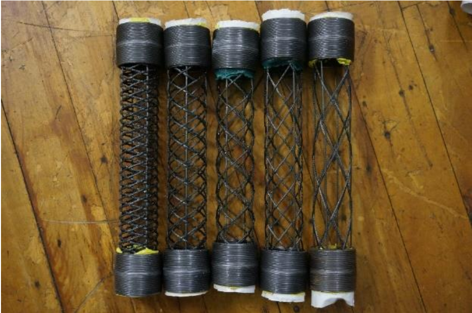
Figure 70 O-ACS samples for compression tests
