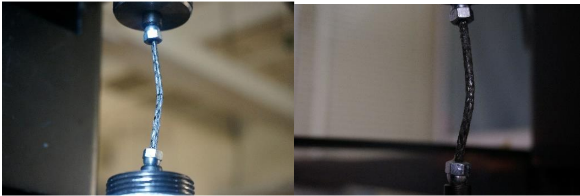
Figure 29 Failure due to the buckling under compression
