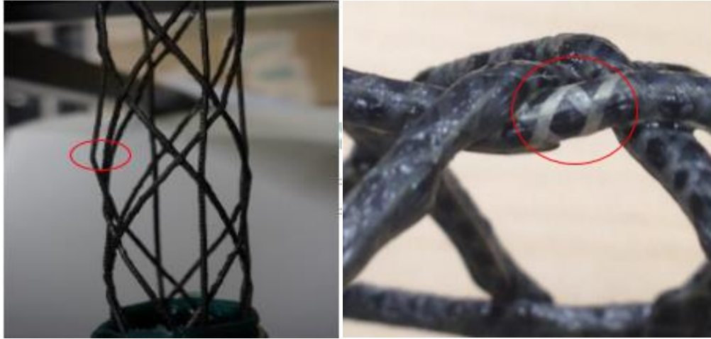
Figure 73 Buckling failure triggered by joint de-bonding (left) and yarn failure (right)
