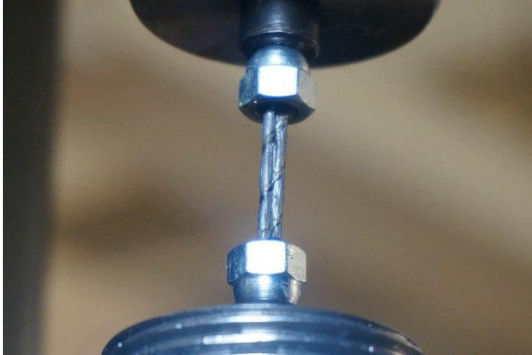
Figure 27 Compression test of cord-pregs
