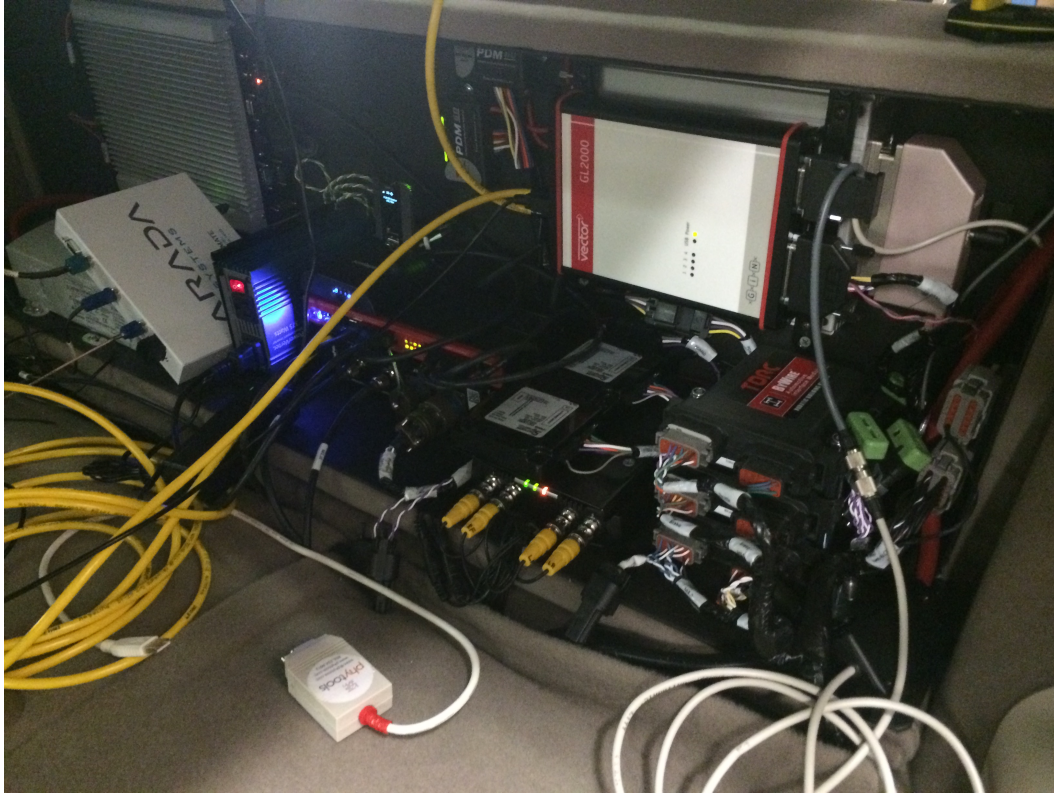
Figure 4.2: Experimental setup in the vehicle which includes MicroAutoBox, DSRC and PinPoint
