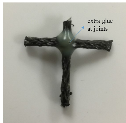
Figure 4.4: A joint with extra glue applied on it
