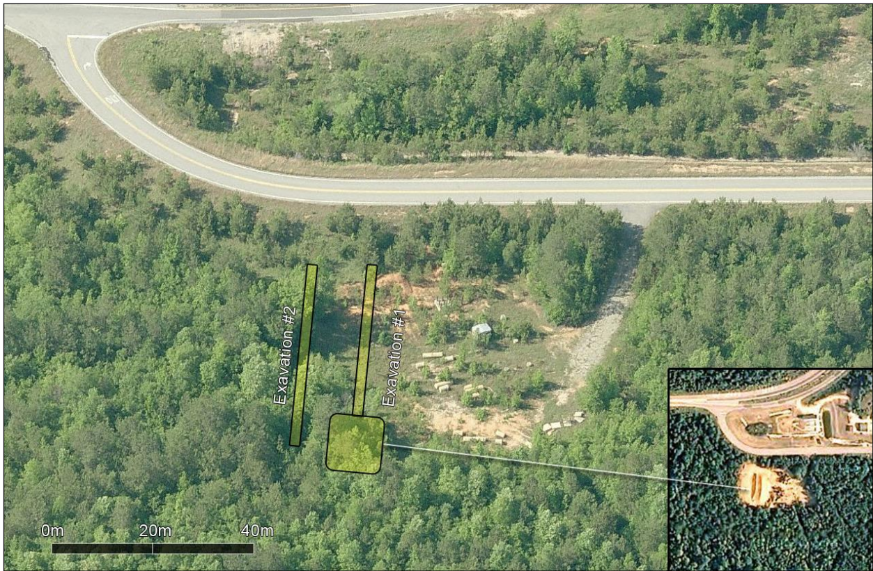
Figure 12 - NGES aerial with approximate excavation locations overlaid (Pictometry, 2012).
