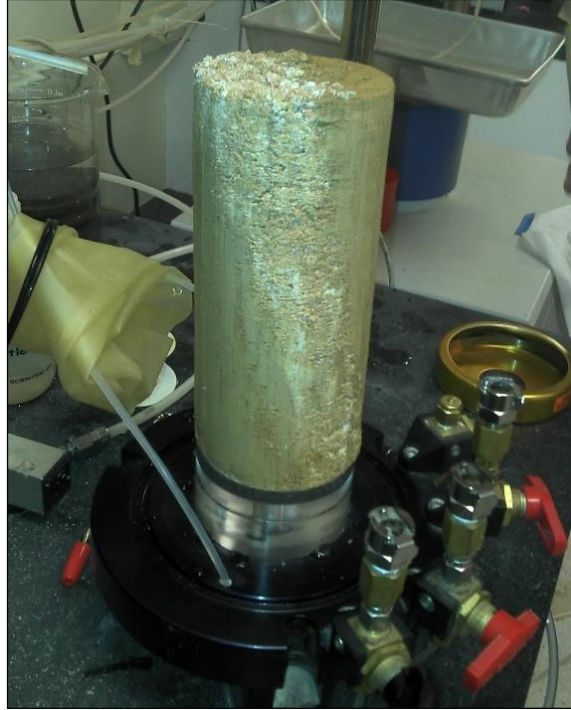
Figure 52 - Thin layers present in undisturbed soil samples.
