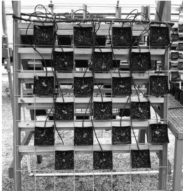
Figure 4.10. A full view of one side of the vertical structure shows how the irrigation system is installed. The main irrigation line is placed on the upper edge of each cattle-fencing panel. Spaghetti tubing is connected to the main irrigation line by two gallon per hour irrigation emitters. Each line of spaghetti tubing is inserted through a pre-drilled hole in the rim of each pot. A 15/64-inch Turbomax drill bit was used to create the hole for the spaghetti tubing.
