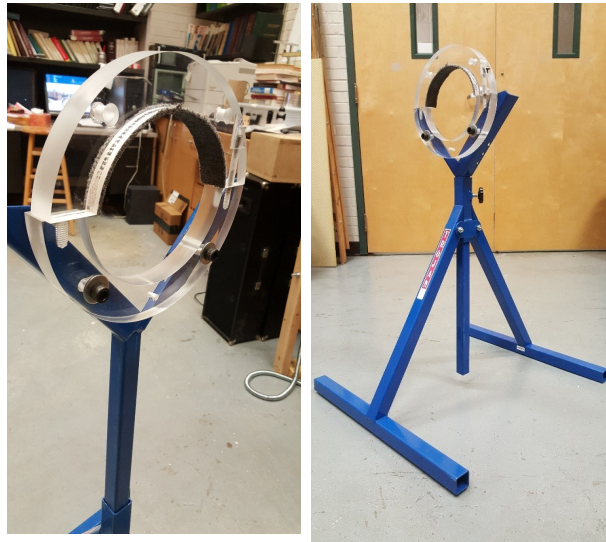
Figure 1.12: Pictures of the jack stand with the fixture to hold the tube
