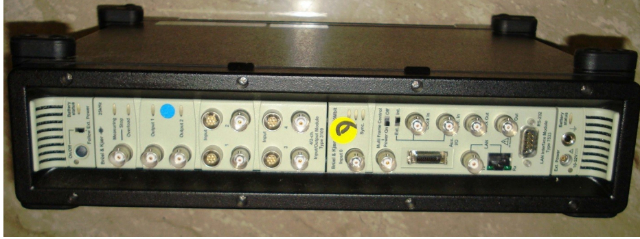
Figure 1.2: Bruel&Kjaer Pulse Multi-Analyzer System Type 3560C
