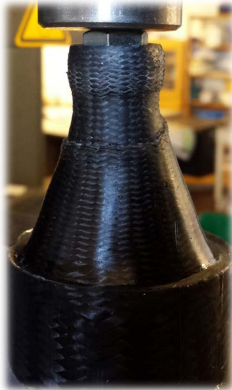
Figure 48 – Failure of Over-Braided Joint #2
