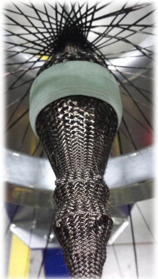
Figure 29 – Layer 1 Complete and Insertion of Silicone Tooling
