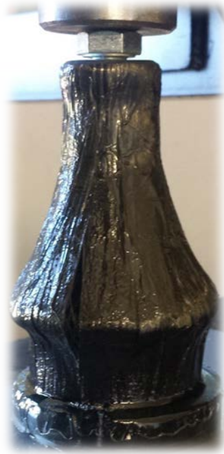
Figure 41 – Failure of Filament Wound Joint #2
