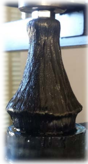
Figure 43 – Failure of Filament Wound Joint #3
