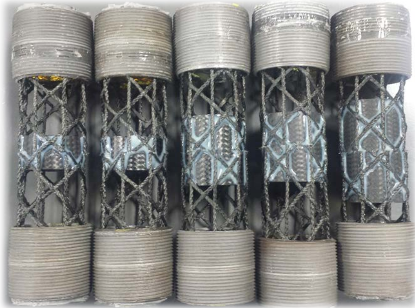
Figure 63 – Potted Splice Joints
