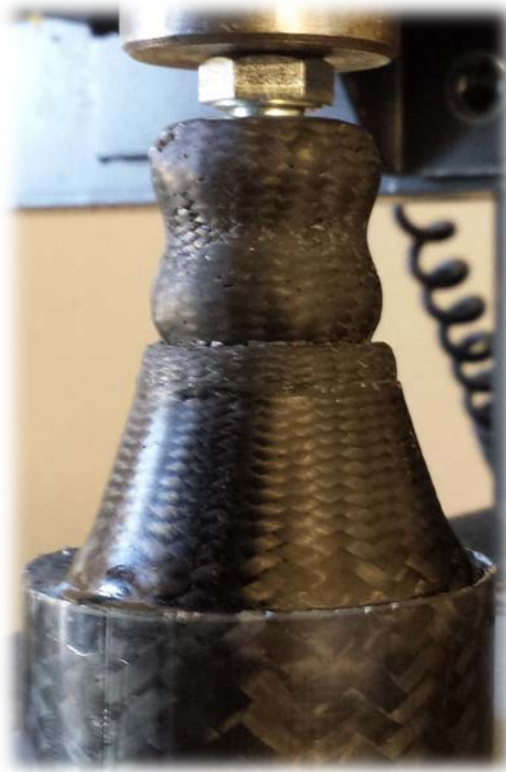
Figure 52 – Failure of Over-Braided Joint #4
