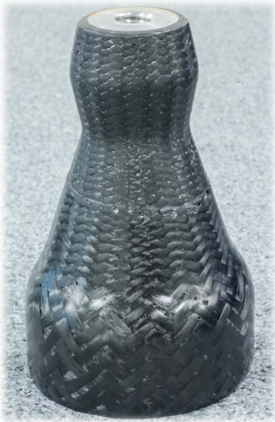
Figure 35 – Joint with Double Taper-Out Insert
