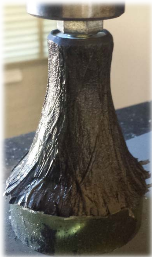
Figure 39 – Failure of Filament Wound Joint #1
