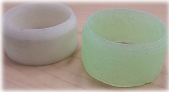
Figure 57 – 3D Printed Master and Silicone Tooling
