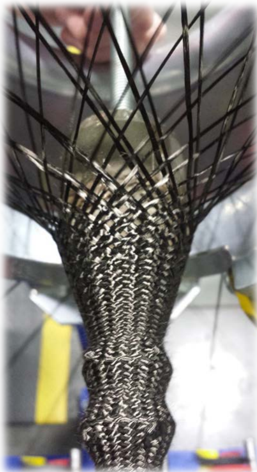
Figure 28 – Over-braiding of First Layer
