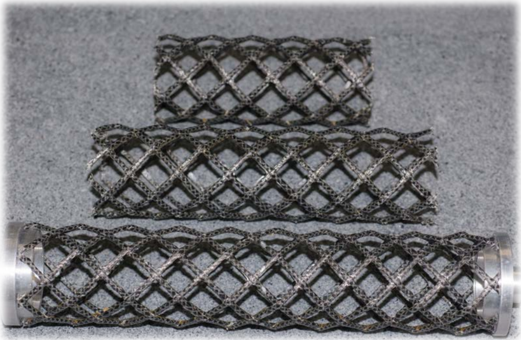
Figure 74 – Varying Lengths of Bi-axial Springs Used for Testing
