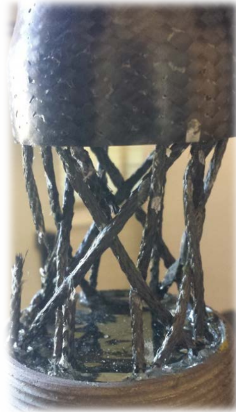
Figure 69 – Detail of Joined O-ACS Failure
