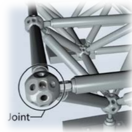
Figure 17 – Truss Structure with Spherical Node Joints
