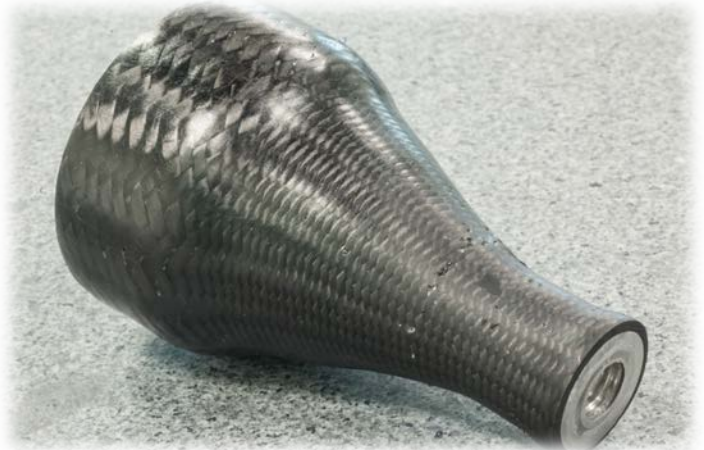
Figure 34 – Joint with V-Groove Insert
