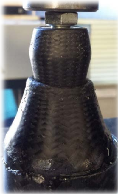
Figure 50 – Failure of Over-Braided Joint #3
