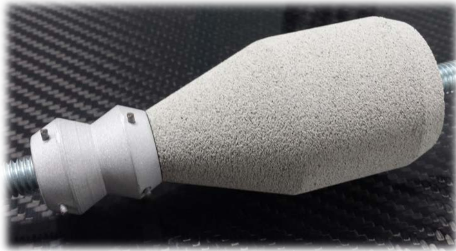
Figure 26 – Wash-out Mandrel and Metal Insert Assembled
