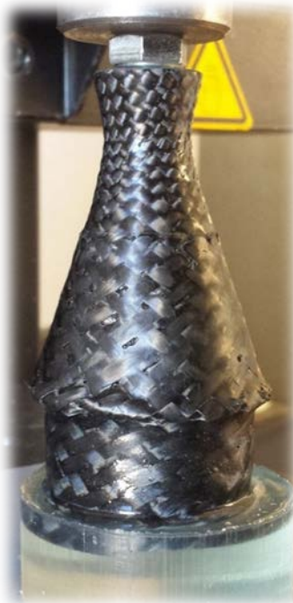
Figure 46 – Failure of Over-Braided Joint #1
