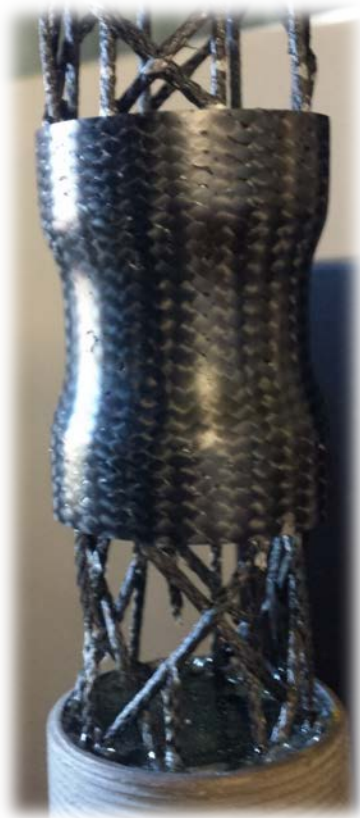
Figure 68 – Coupler Joint Post-Failure
