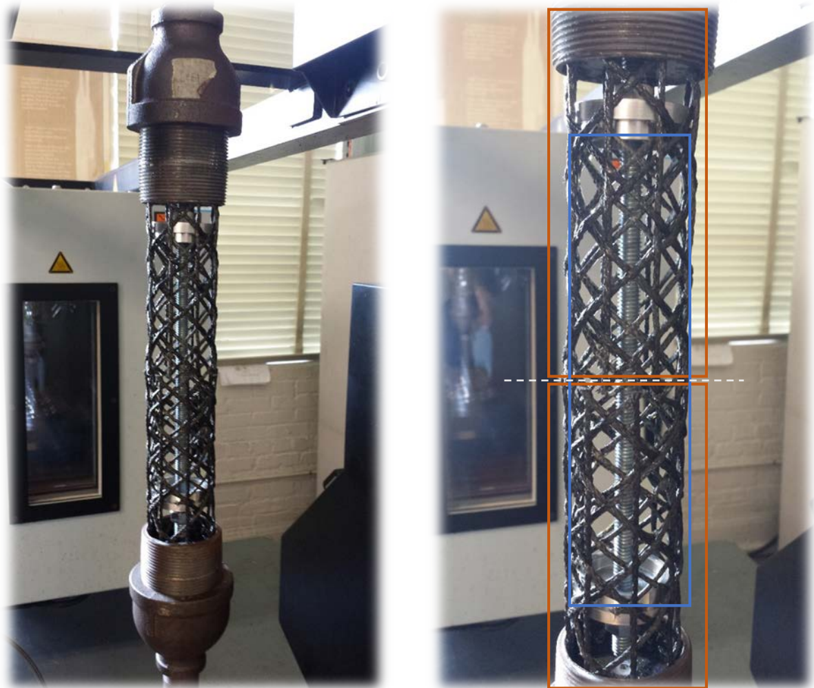
Figure 75 – Specimen Fixtured for Tensile Testing
