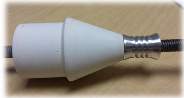
Figure 20 – Gypsum Plaster Mandrel and Insert
