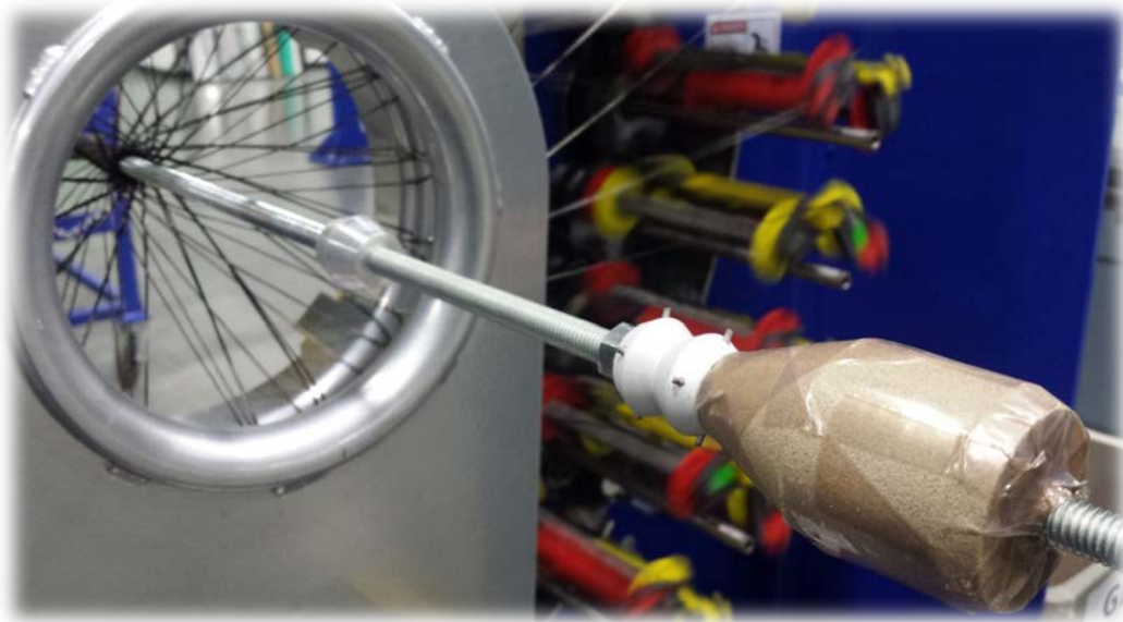
Figure 27 – Mandrel mounted for over-braiding
