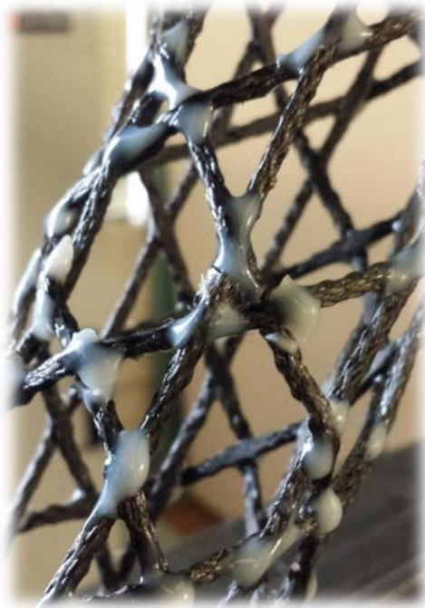
Figure 8 – O-ACS with Epoxy Reinforced Micro-joints
