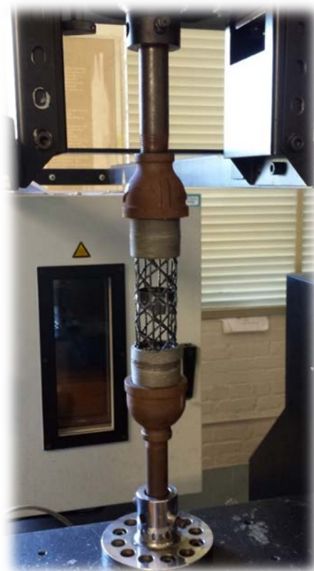
Figure 62 – Fixturing of Potted O-ACS
