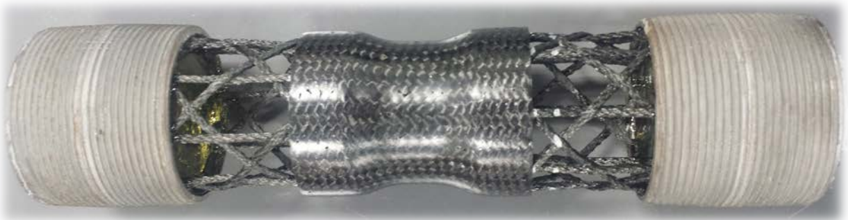
Figure 66 – Coupler Joint Potted for Testing
