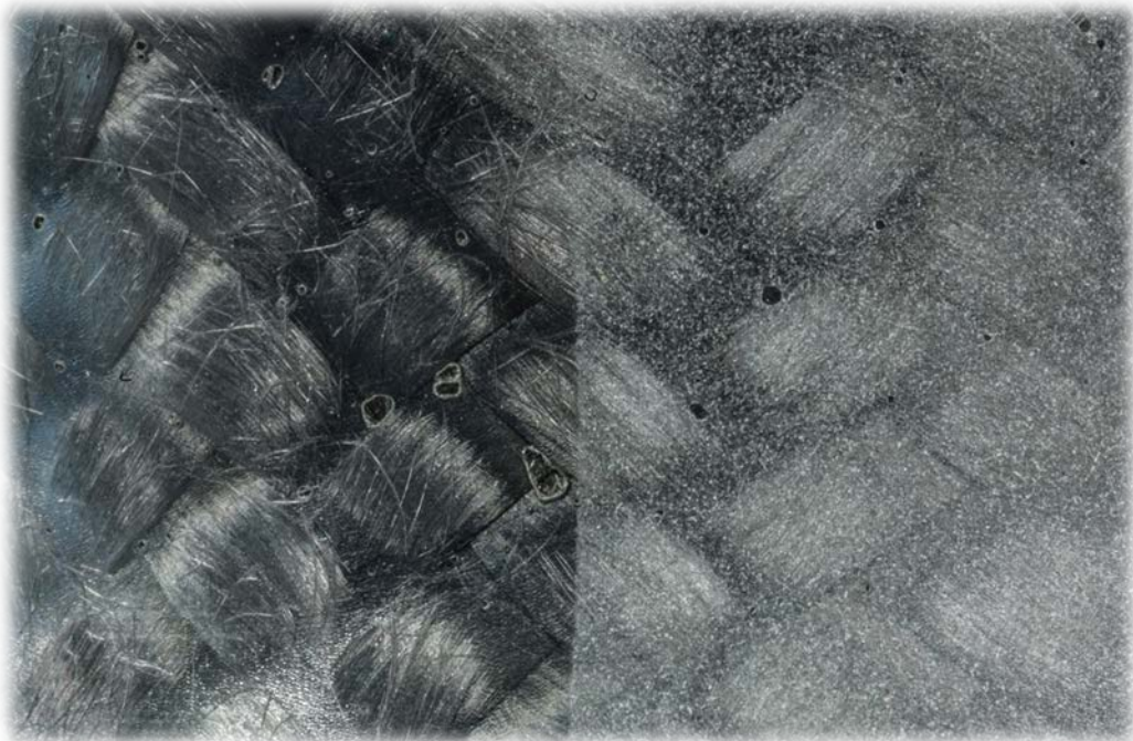
Figure 56 – Un-prepped Composite vs. Media Blasted
