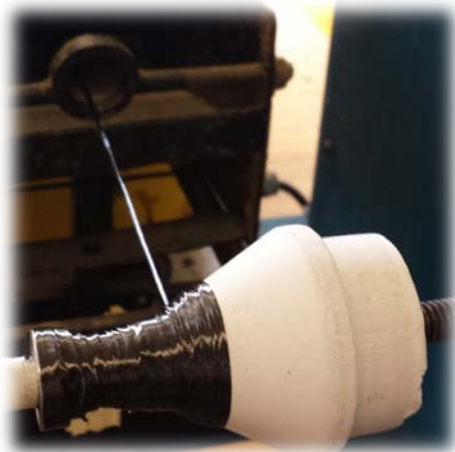
Figure 21 – Filament Winding of 90° Ply #1
