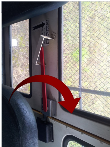
Figure 3.8: Motion Required to Unlatch Rear Emergency Door on a Rolled-Over School Bus
