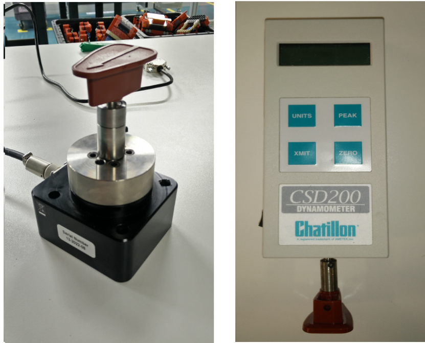
Figure 4.10: Torque and Push Force Measurement Devices
