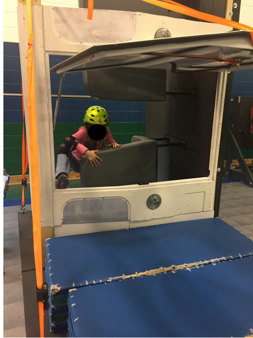
Figure 3.11: Self-Extrication With Rear Seat Obstruction
