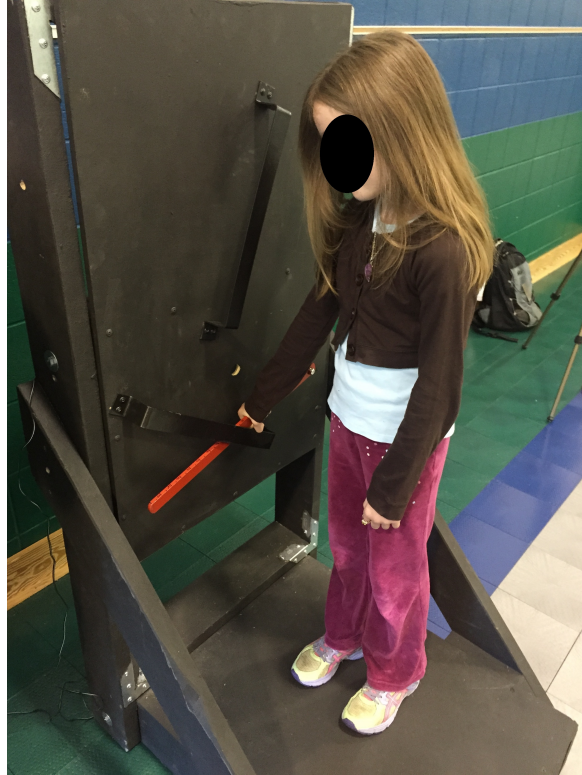
Figure 3.5: Door Handle Force Measurement in the Upright Orientation
