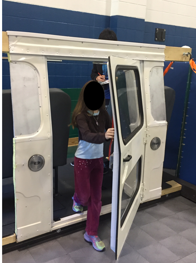
Figure 3.4: Unlatching Rear Emergency Door in the Upright Orientation
