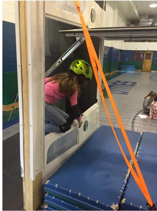
Figure 3.10: Self-Extrication Without Rear Seat Obstruction
