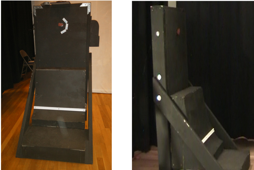
Figure 4.9: Torque and Push Force Measurement Stand
