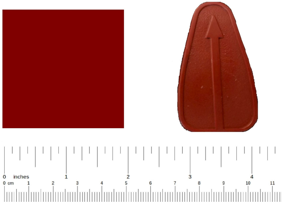
Figure 4.5: Surface Area Comparison of Roof Hatch Knob to Plastic Cube (50 mm x 50 mm)
