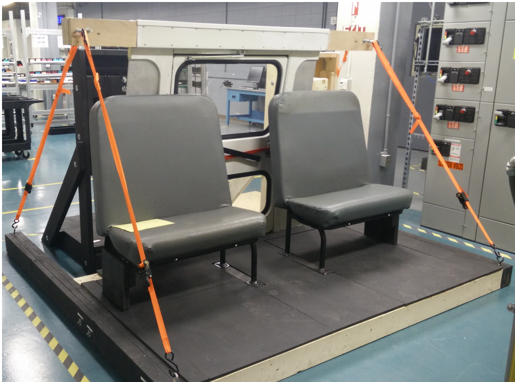
Figure 3.3: Rear Emergency Door Evacuation Test Apparatus
