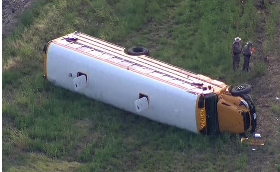
Figure 1.1: Rolled Over School Bus with Roof Hatches Opened [Associated Press, 2014]
