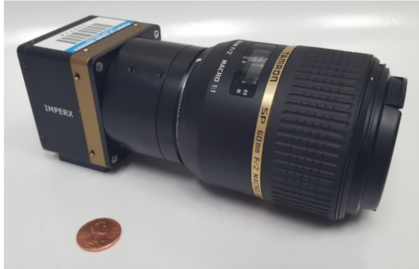
Figure 4: Plenoptic camera currently in use at Auburn University equipped with a 60 mm Tamron main lens
