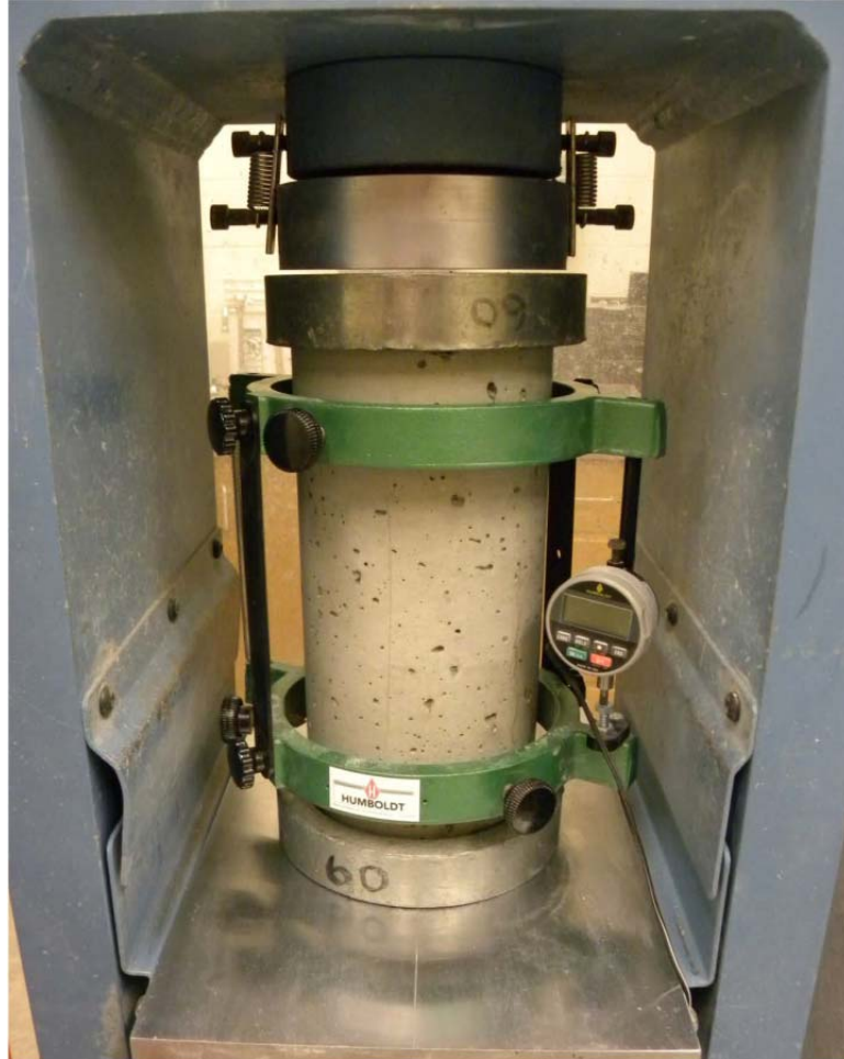
Figure 6-5: Cylinder Prepared for Elastic Modulus Testing
