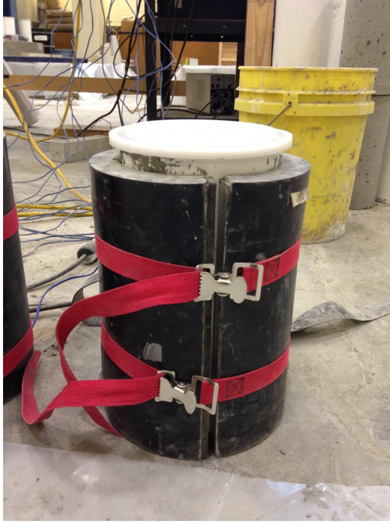
Figure 6-4: SURECURE Jacket for Accelerated Curing
