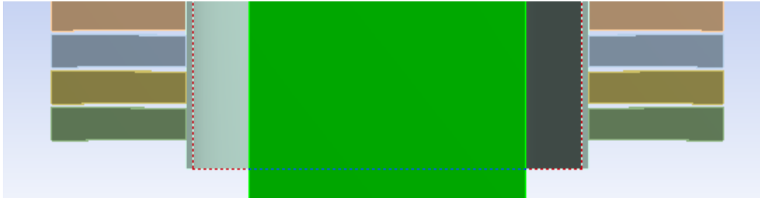
Figure 72: Sectioned view of annular comb, showing solid backbone and interrupted, annular teeth. (The green cylinder in the middle is a placeholder for the human leg)
