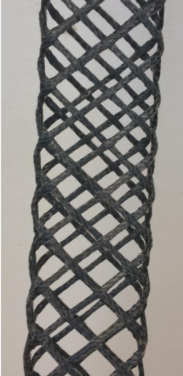
Figure 26: Generic biaxial braid of cured carbon-fiber prepreg. This particular braid was formed over a mandrel with rectangular cross-section, although most studied had circular cross-sections.
