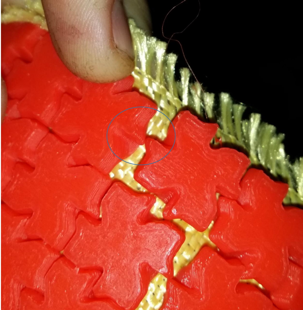
Figure 216: Tooth protrusions catching on each other as the array returns to standard shape after significant local shearing or bending (circled).
