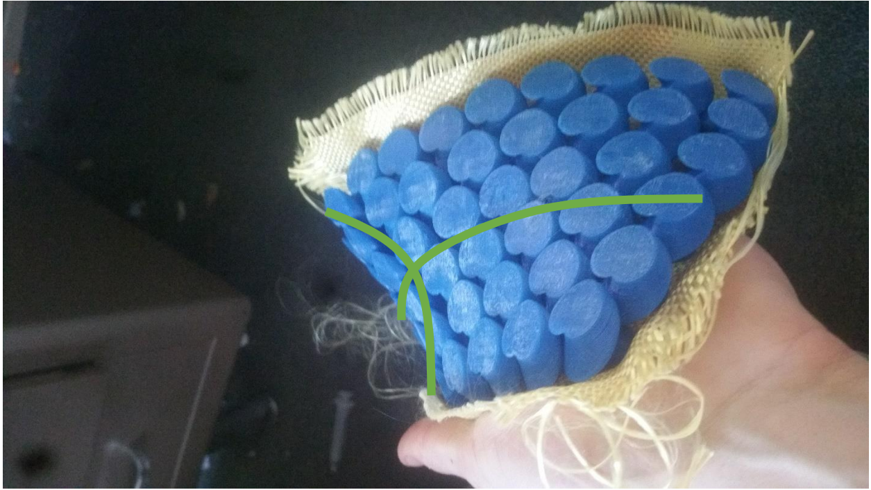
Figure 235: Compressing the square-packed array along either diagonal produces sympathetic deformation into a saddle shape (anti-clastic curvature).
