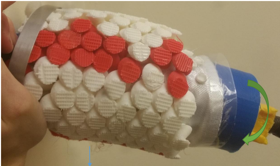
Figure 367: Side view of test fixture fitted with pre-curved array, bent until lockup. The green arrow shows the direction of bending, and the blue arrow shows the vertical direction (the plane of the base of the test fixture contains this vector).
