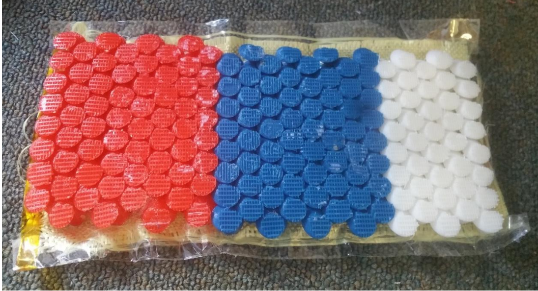
Figure 307: Long array ready to be wrapped into a cylinder, consisting of three separate prints (conveniently produced in different colors).
