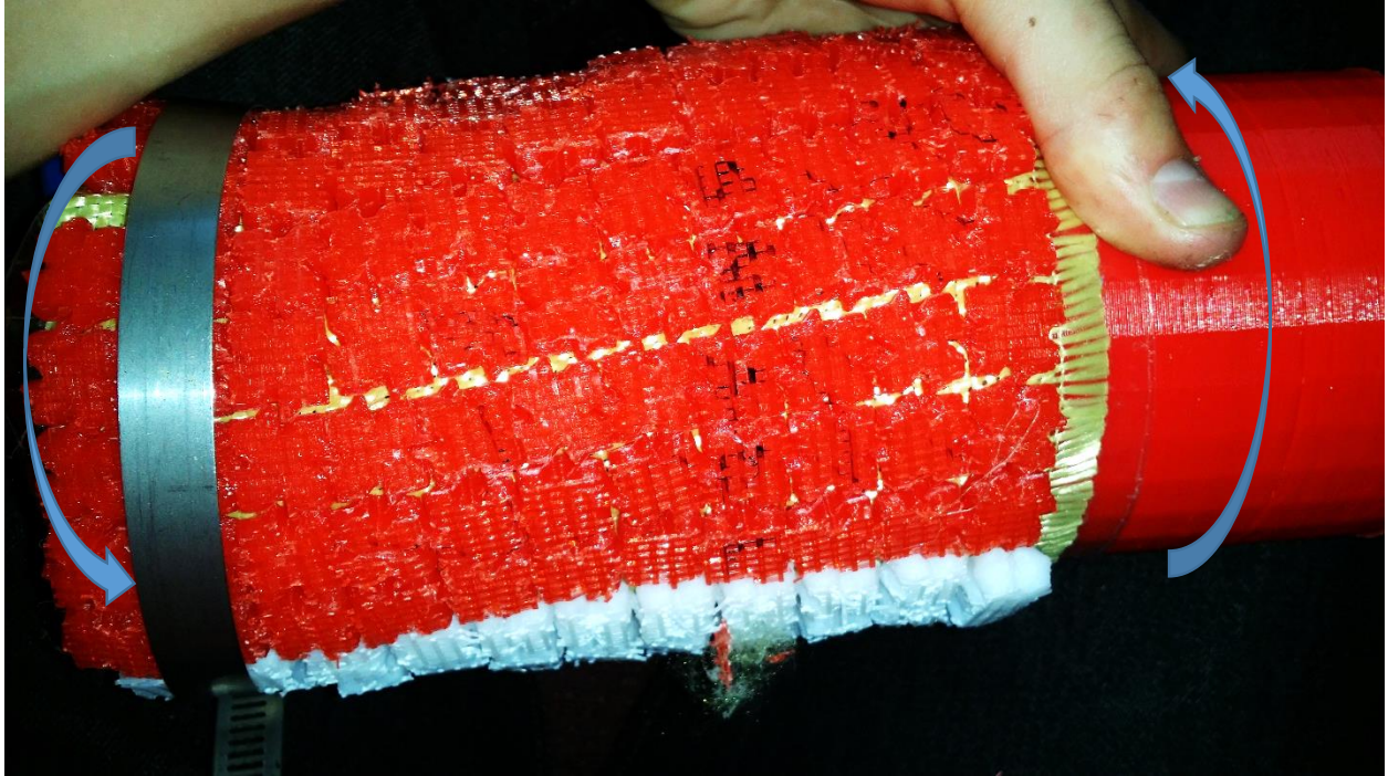
Figure 319: Torsional lockup of the array after being rotated clockwise (viewing from the top) thanks to tooth contacts. The direction of the torsion is also indicated with blue arrows.
