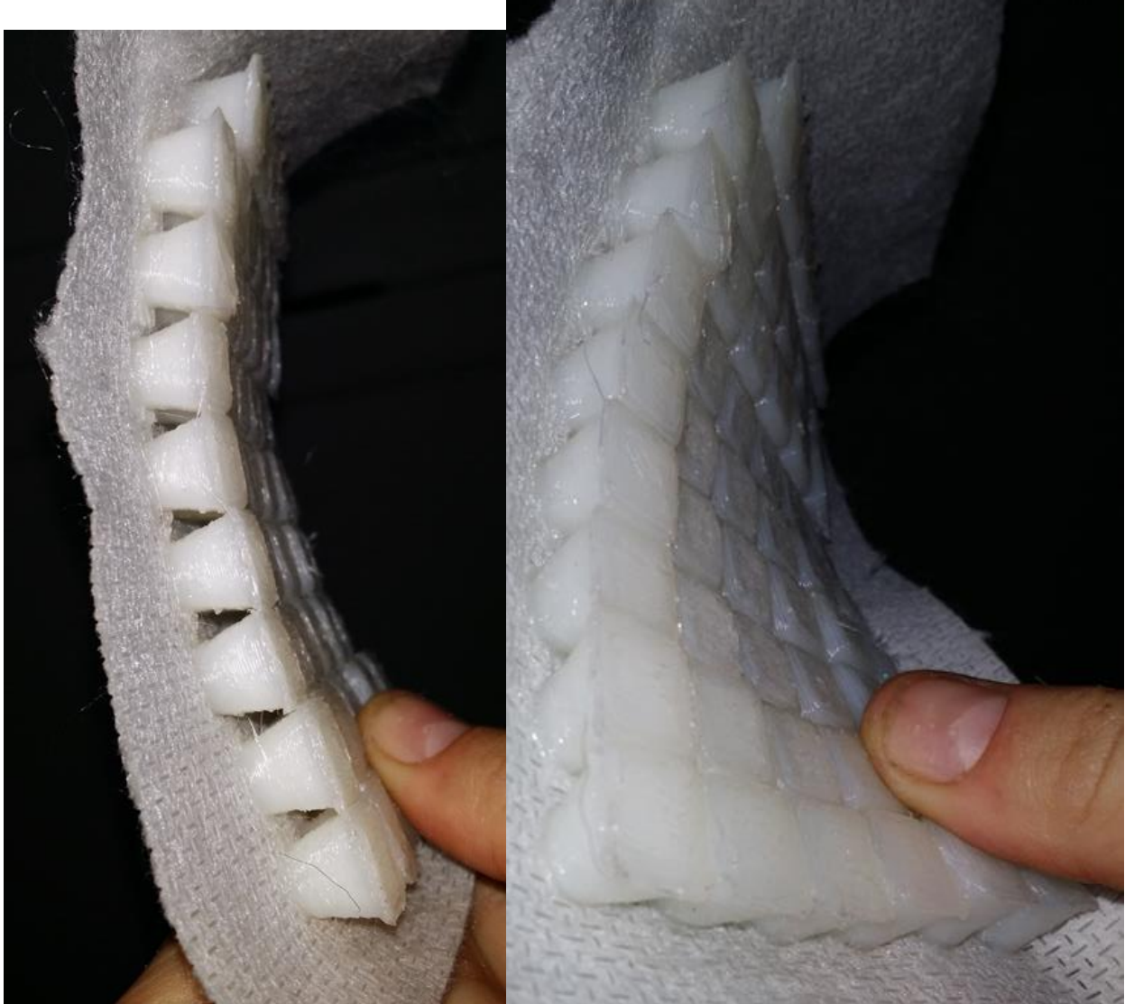
Figure 207: Bending the square array about an angle that is an integer multiple of 90^\circ (left) produces less curvature than bending about a different angle (right).
