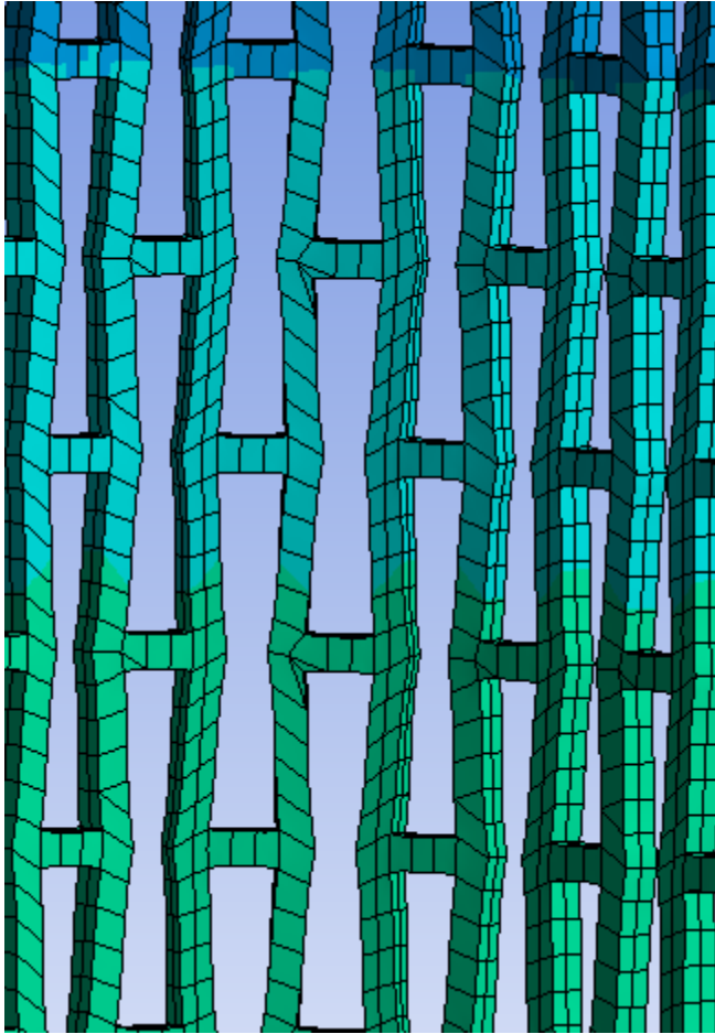
Figure 112: The maximum stretch achieved by the simulation. Subjecting the reentrant backbone alone to vertical tension did indeed straighten out the reentrant hexagon cells into near-rectangular shape as anticipated. However, there was some vestigial bowtie-like shape to the cells even after significant tension, suggesting that some aspect of the cantilevered joints between cells was behaving improperly.
