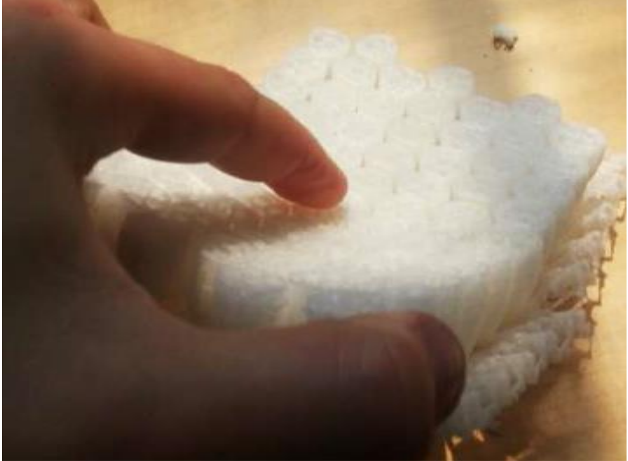
Figure 180: Overall view of the printed structure in bending. Note the synclastic curvature. Unfortunately, it was fairly compliant after “lockup”.
