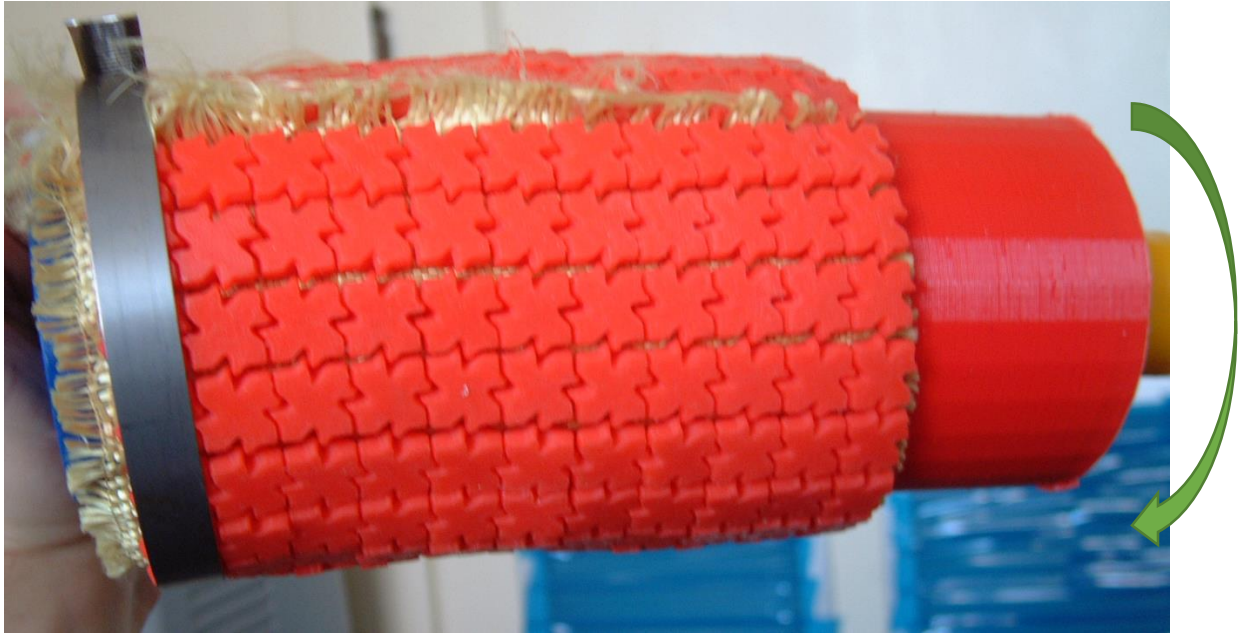
Figure 311: Side view of array mounted on test fixture; the direction of “leg” rotation is shown with the green arrow.
