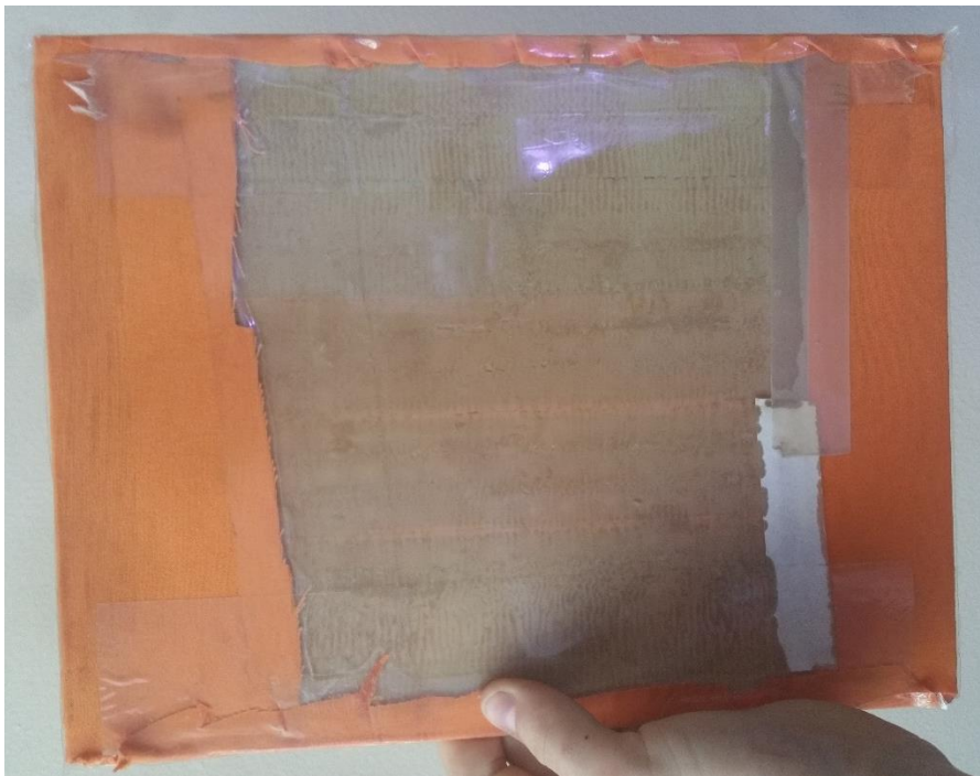
Figure 374: Underside of glass plate: the edges of the fabric have been secured with tape to the glass.
