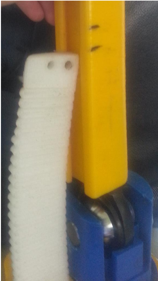
Figure 50: Deformation of comb when sole attachment to leg is low-friction contact. Right: unattached comb stands up roughly straight under its own weight.
