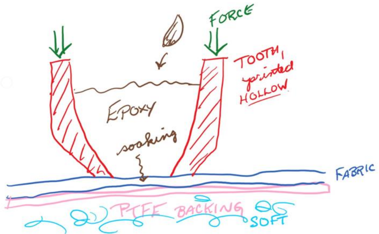
Figure 298: Sketch of tooth-filling process that should also see a strong bond between the filling epoxy and fabric.
