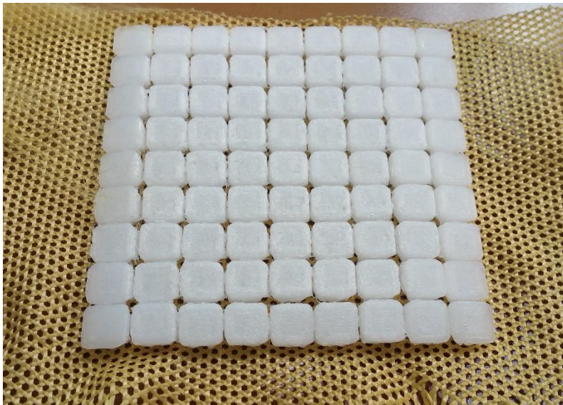
Figure 187: Tooth array on triaxial-weave Kevlar fabric (neutral).
