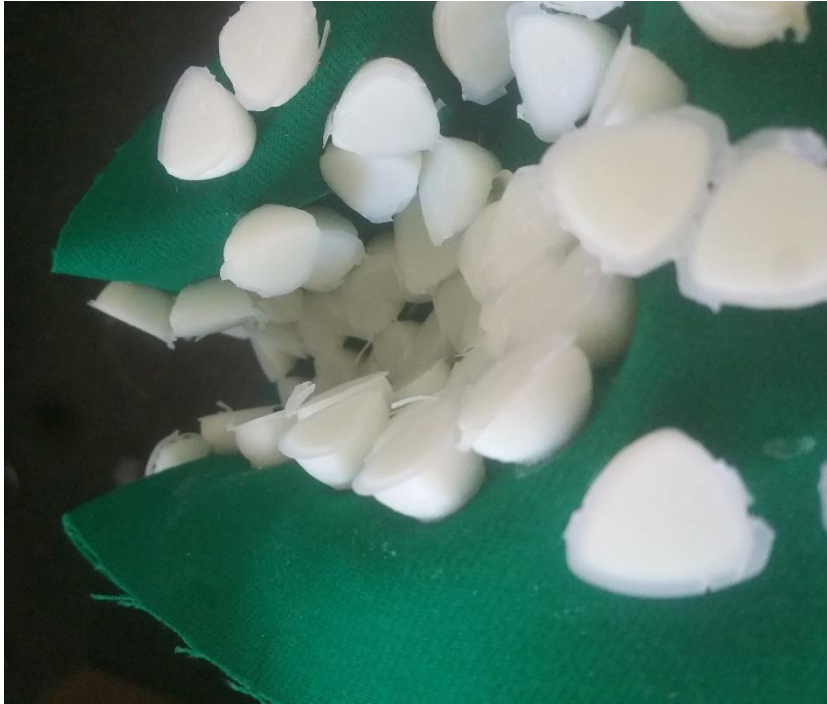
Figure 275: The array based on Reuleaux triangles did not lock up effectively in bending.
