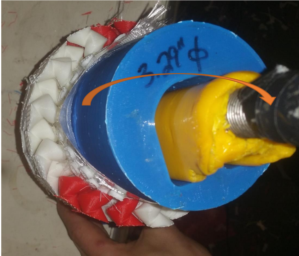
Figure 368: Top view of test fixture fitted with pre-curved array, bent until lockup. The orange arrow shows the direction of bending.
