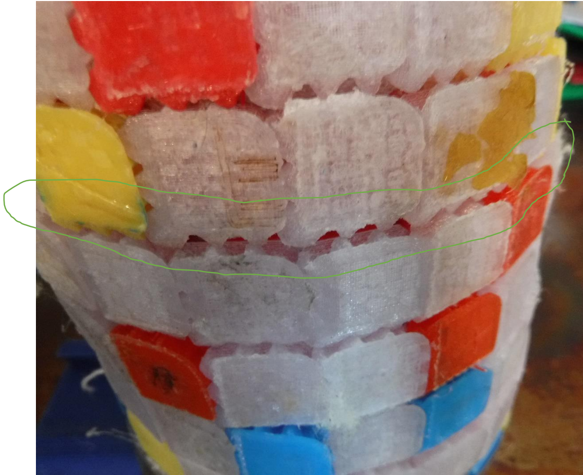
Figure 350: Close-up view of area offset 90° from the direction of leg rotation. The teeth in this portion of the array do not lock up in vertical contact from leg bending, but they do lock up in shear once they cannot slide past each other any further. In fact, the tooth design seems to cam the teeth apart vertically, leaving them further separated vertically than they were at the neutral position. This view most clearly shows the contact that produces shear lockup in the row that has been circled in green.
