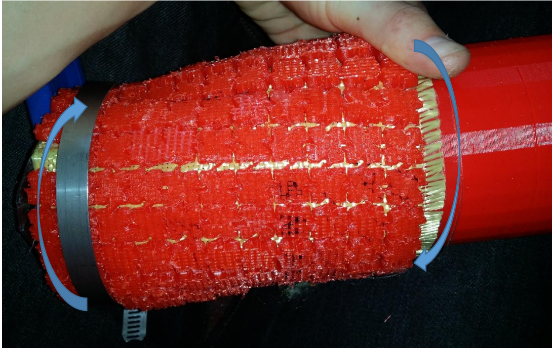
Figure 320: Torsional lockup of the array after being rotated counterclockwise (viewing from the top) thanks to tooth contacts. The direction of the torsion is also indicated with blue arrows. Note that this is the opposite direction of torsion from that of Figure 319.
