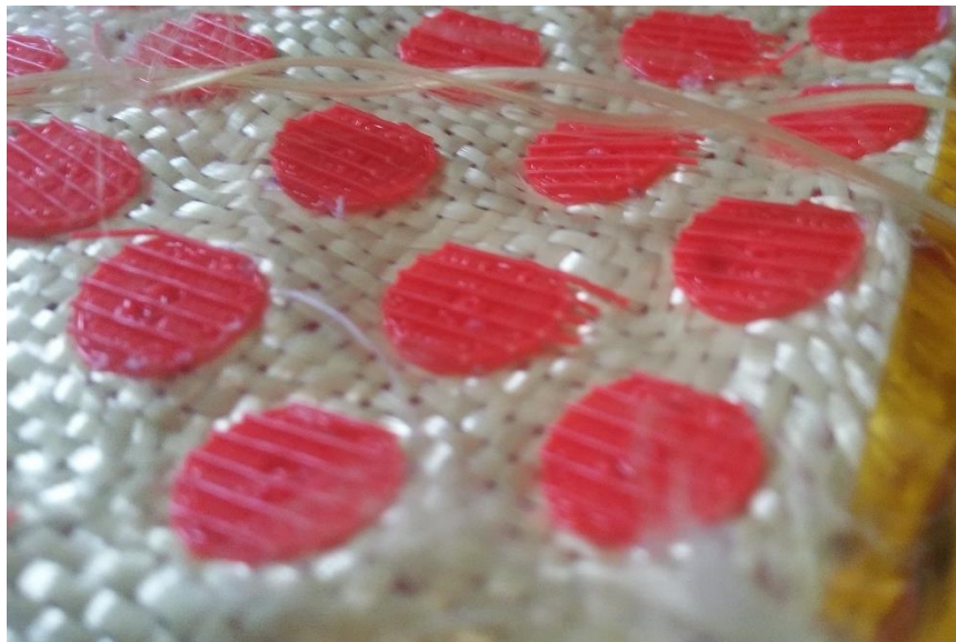
Figure 303: The underside of a fabric-backed array, showing rivets used to improve bonding between the teeth and the fabric.
