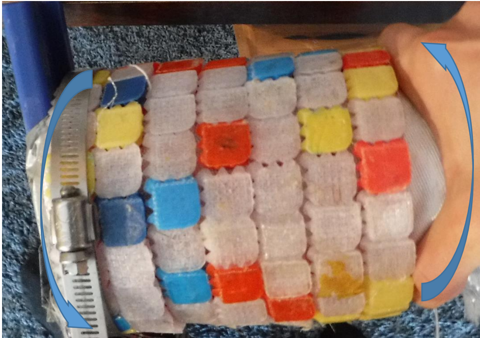
Figure 355: Maximum extent of torsional freedom at lockup, torsion in one direction (indicated with blue arrows).
