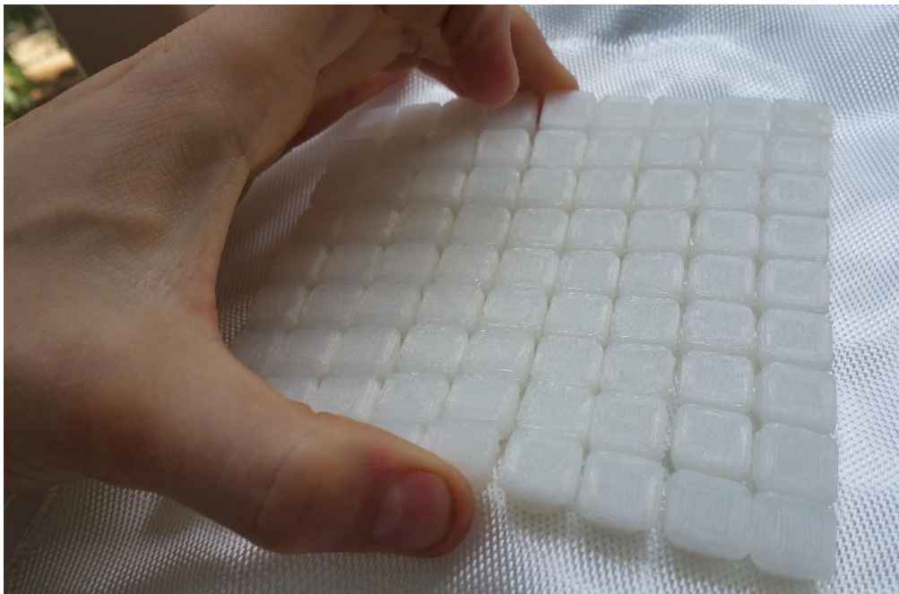
Figure 185: Showing bending lockup of fiberglass with tooth array.
