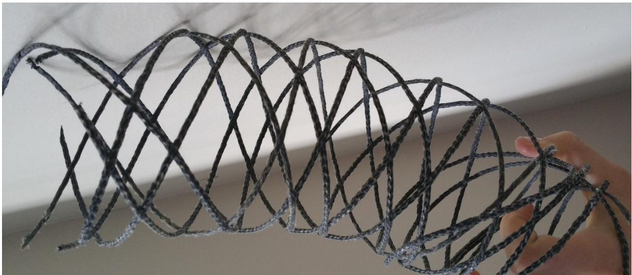
Figure 29: Open-structure braids also have significant bending compliance.
