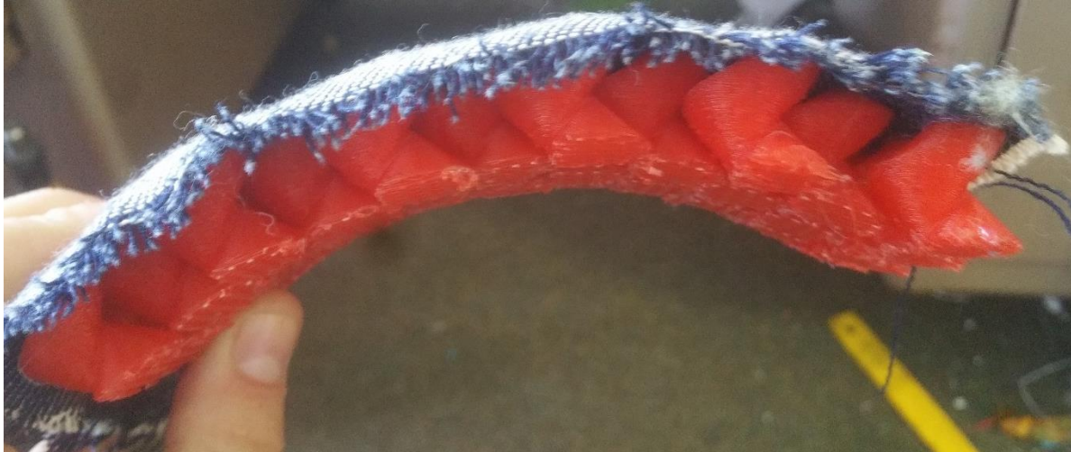
Figure 230: Post-lockup bending curvature of the array. Note that its curvature seems somewhat higher than that for the unscaled array (shown in bending in Figure 225), despite having the same nominal tolerances in the direction shown in green in Figure 227. This indicates that initial diagonal clearances between teeth also affect post-lockup position.
