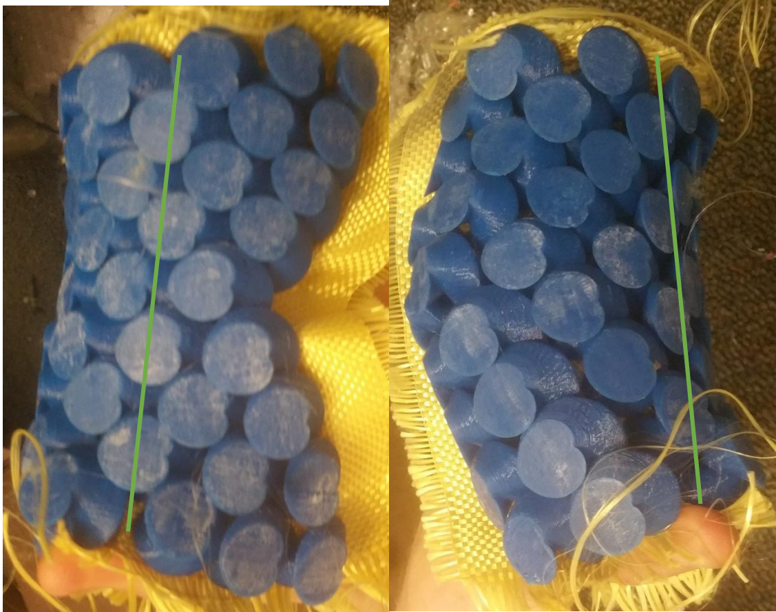
Figure 238: “Double-chevron” instability mode with compression along the axis shown in green, 2 views.
