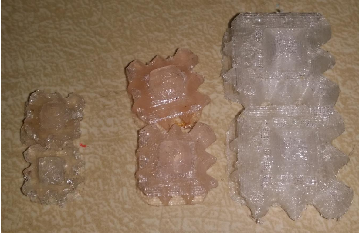
Figure 376: Right to left: original teeth, teeth reduced to 70% of initial size, teeth scaled to 50% of initial size.\
