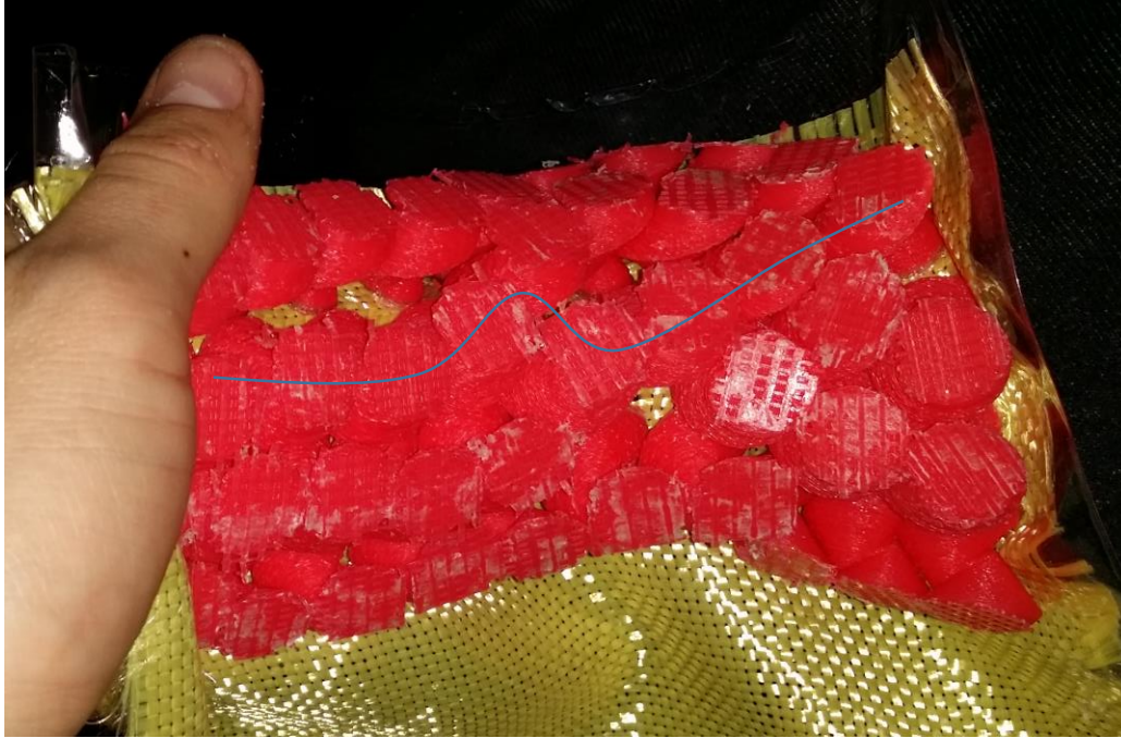
Figure 322: Compressing the paradoxical array with 0.050" clearances between teeth does produce cylindrical conformation, but it seems to be governed by instability. What was once a straight "zig-zagged" row of teeth is traced in blue to illustrate the irregular behavior.
