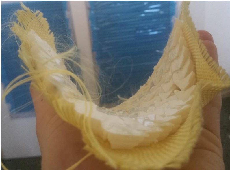
Figure 288: Lockup curvature in bending about a different axis from the one shown in Figure 287.
