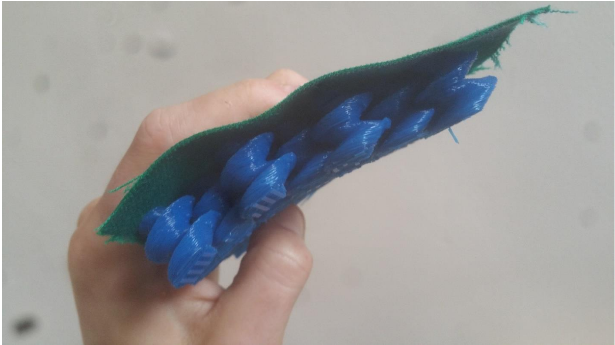
Figure 241: Slight curvature of the double-rotated array at lockup.
