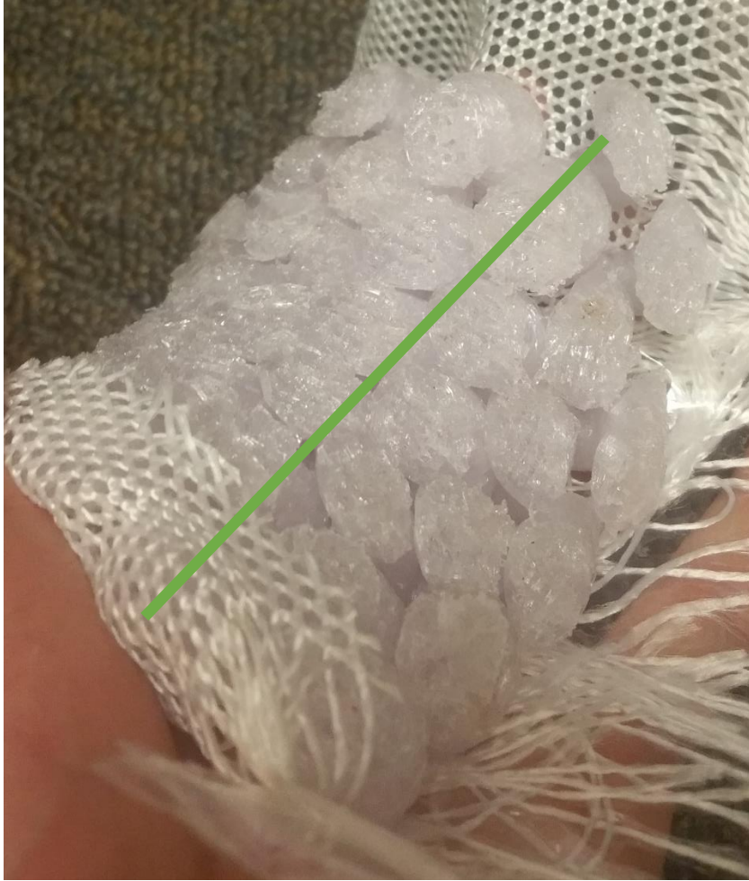
Figure 226: Sympathetic cylindrical deformation of paradoxical-gear-based array with .040" clearances in compression along the axis shown in green (plus a small amount of bending).
