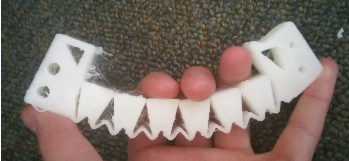
Figure 57: Wavy-backbone linear comb bent just until teeth touched lightly. Note that the wavy backbone is not significantly, visibly elongated.
