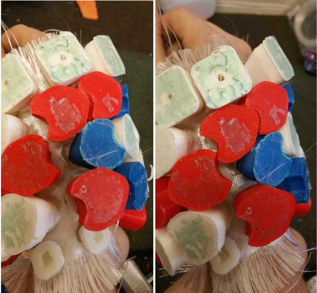
Figure 334: Cylindrical array tested on a human wrist. In the left picture, the wrist is in neutral position, with negligible bending along the neutral axis of the cylindrical axis. A few teeth are touching lightly. In the right picture, many teeth have come to touch, both vertically and tangentially, and the structure is effectively locked up.
