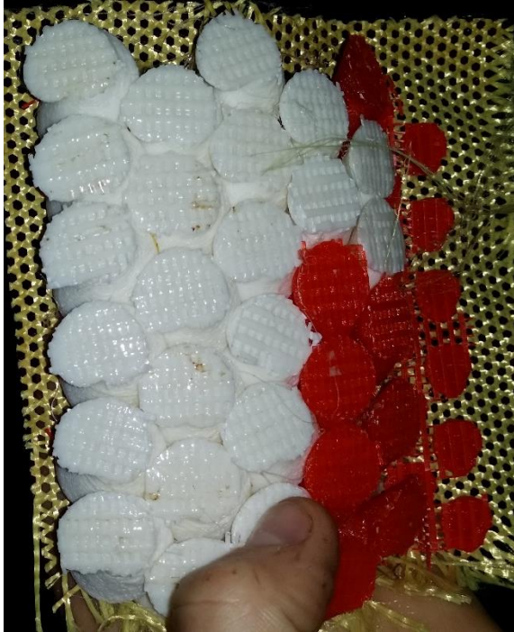
Figure 371: Undeformed view of the array. Note the irregularity in the rotations of teeth; this is due to poor accuracy in assembly (likely the result of thin walls in the base feature that cannot exert a strong hold on the corresponding feature on the tooth inserts).
