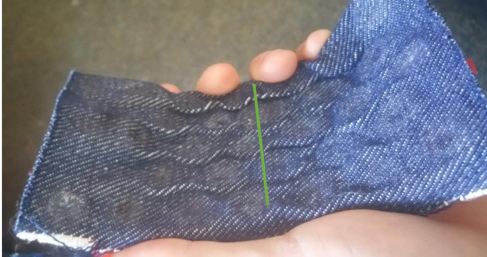
Figure 233: Underside view of 125%-width-scaled HCP paradoxical-gear array in compression along the axis drawn in green (with coupled cylindrical deformation). Note that this curvature is softer than that for the unscaled HCP paradoxical-gear array.
