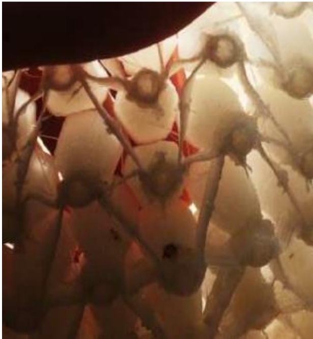
Figure 179: Shell buckling of beams (with their long axes oriented to produce the highest second moment of area when the sheet is in bending) and snap-through of the kite shapes after bending, both of which inhibit post-lockup stiffness.
