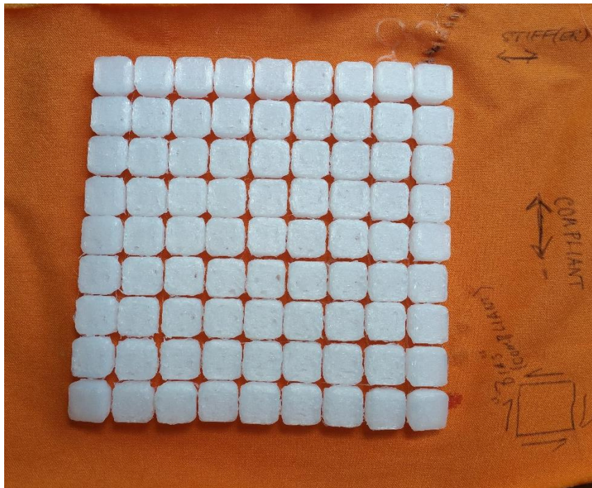
Figure 194: Cotton-polyester-elastomer fabric with significant anisotropy (compliance in one axial direction much higher than in the other) with tooth array printed thereon. As shown by the drawings on the fabric, the single orthogonal compliant axis also renders the cloth compliant in shear, even though it does not have a weave that itself gives a lot of bias compliance.
