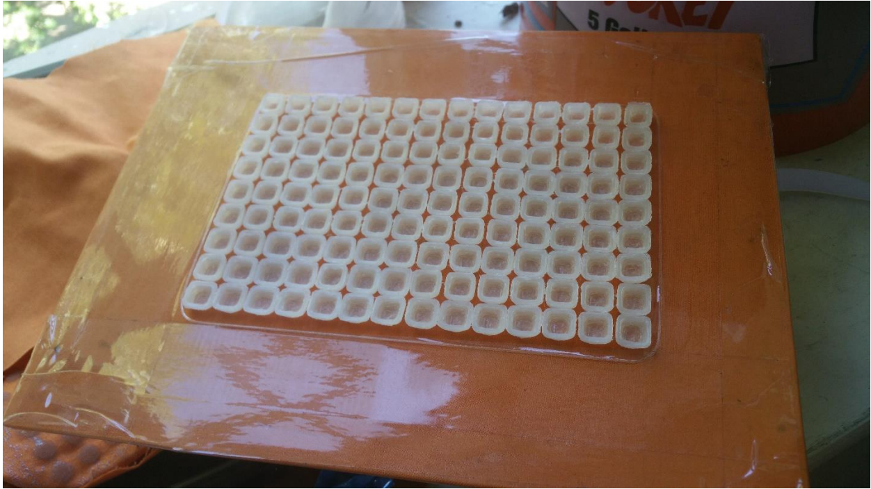
Figure 373: Top view of glass plate with fabric securely attached (note packing tape around print area to further protect against warping.
