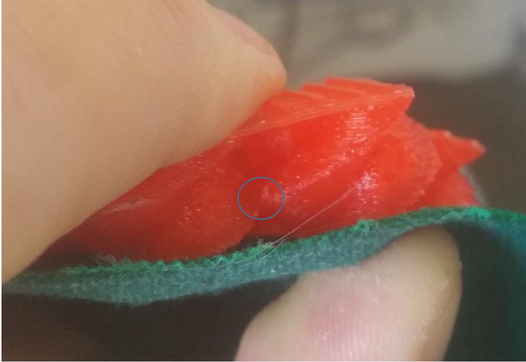
Figure 252: Close-up view of two teeth in contact over a very small area (circled) in bending.
