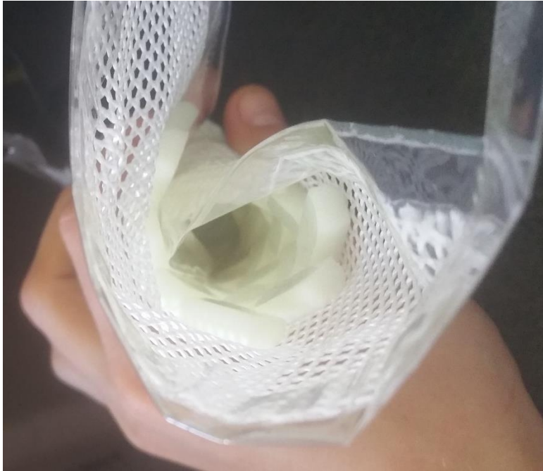
Figure 280: Curvature of the array at lockup after bending along the axis associated with highest curvature (shown in blue in Figure 279)
