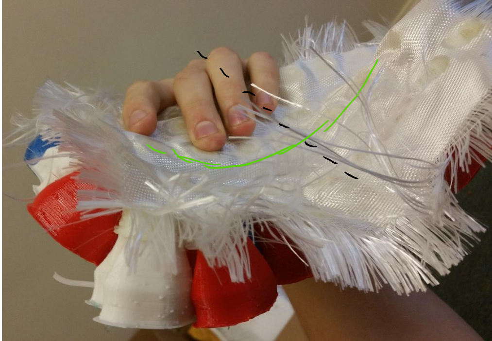
Figure 330: Precurved array in the undeformed position. Its cylindrical curvature is traced in green; the vertical axis of its cylindrical face is drawn with a black dashed line.
