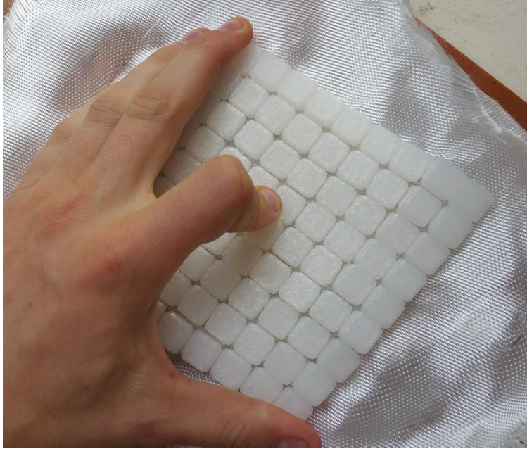
Figure 186: Showing lockup after some planar shear strain.
