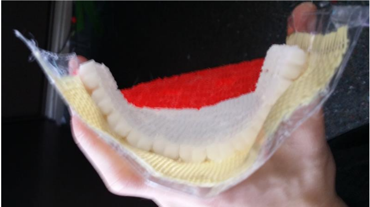
Figure 313: Curvature at planar-bending lockup of the high-clearance (0.036") portion of the array.
