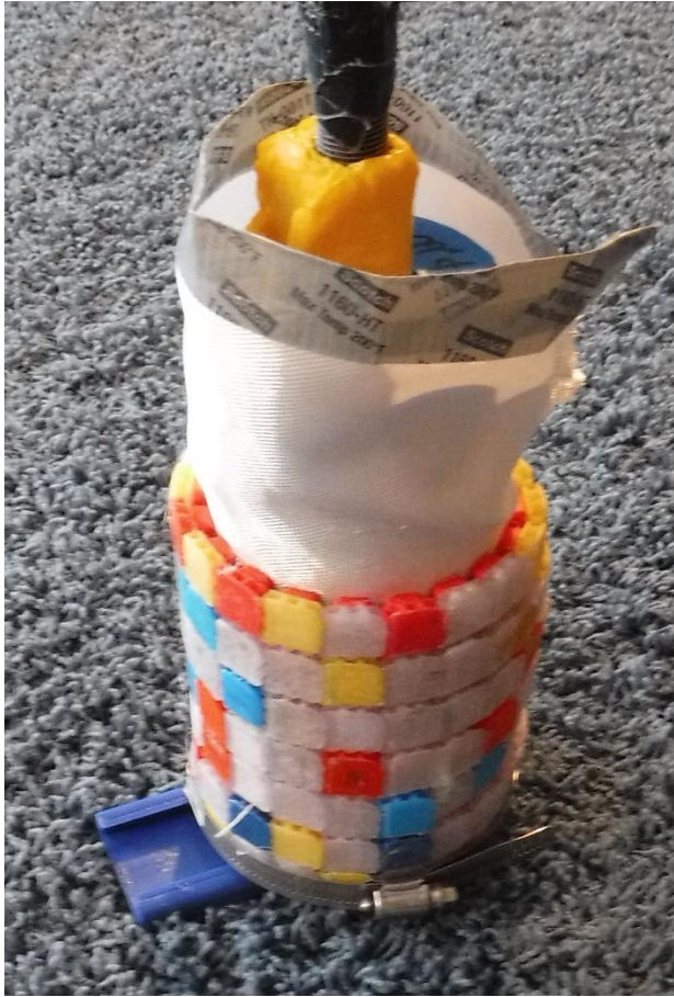
Figure 347: Fabric array with FTASF teeth, mounted on the test fixture, with the joint in the neutral position.
