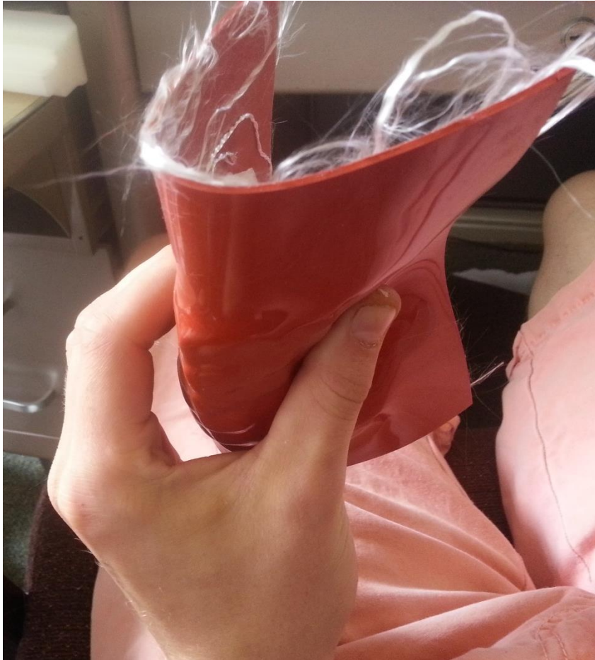
Figure 190: Unsatisfactory post-lockup stiffness of the silicone-backbone tooth array.
