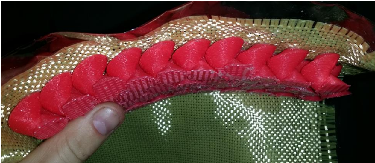
Figure 321: Planar bending lockup curvature of the paradoxical-gear-based array with 0.050" offset between teeth.
