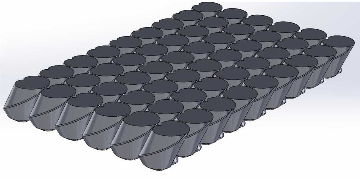
Figure 218: Array of teeth based on the Mercier paradoxical gear.
