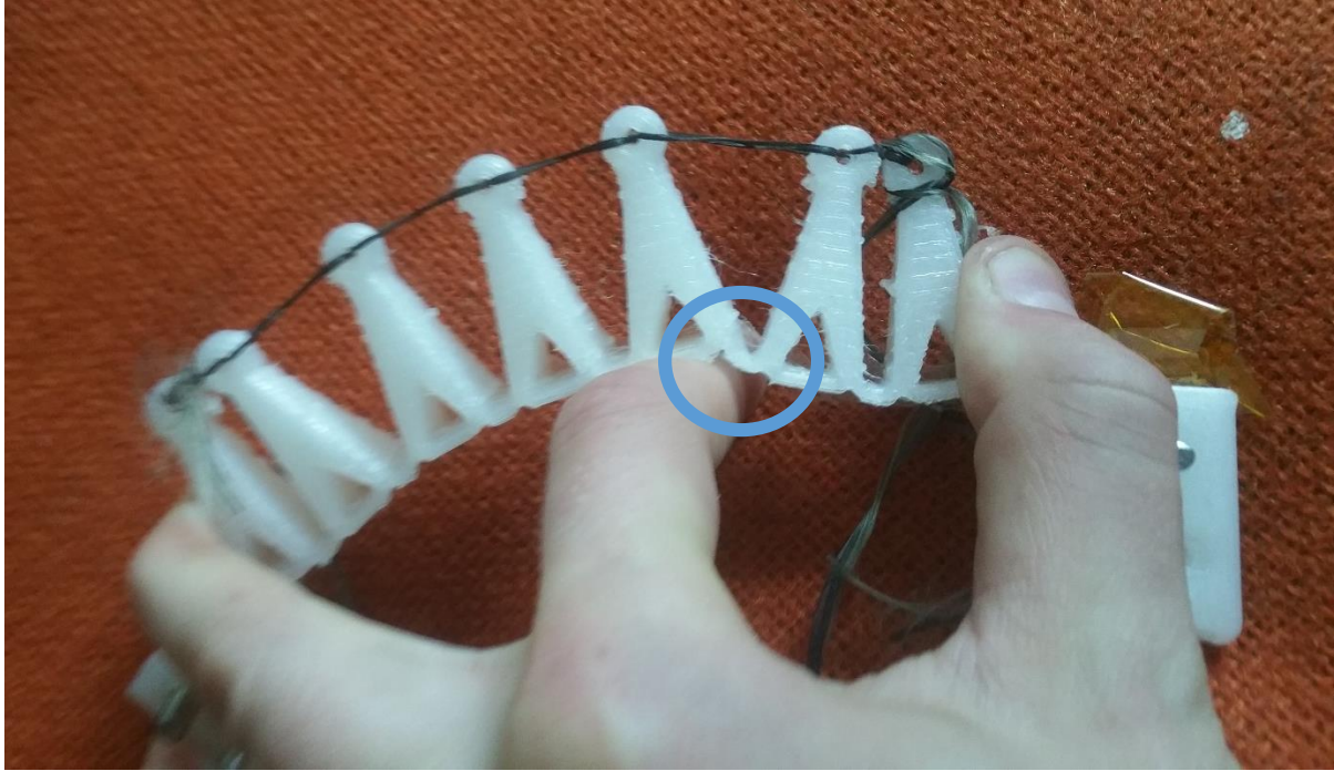
Figure 60: Local buckling of the backbone of the cable-based stiffener (circled in blue) after most cables have become taut. The backbone may have been especially vulnerable to buckling at this point because of local damage it sustained. The backbone also saw some deformation in shear normal to its curvature.
