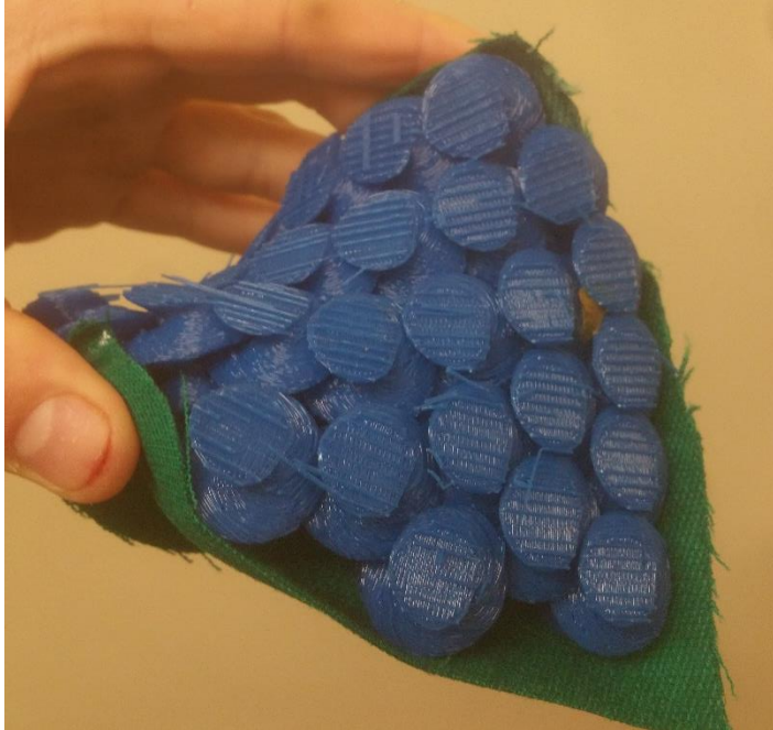
Figure 244: Compressing the array along a different axis from the one shown in the previous figure also produces sympathetic curvature in two directions, but this time the profile is anticlastic, as seen in most other paradoxical-gear arrays.
