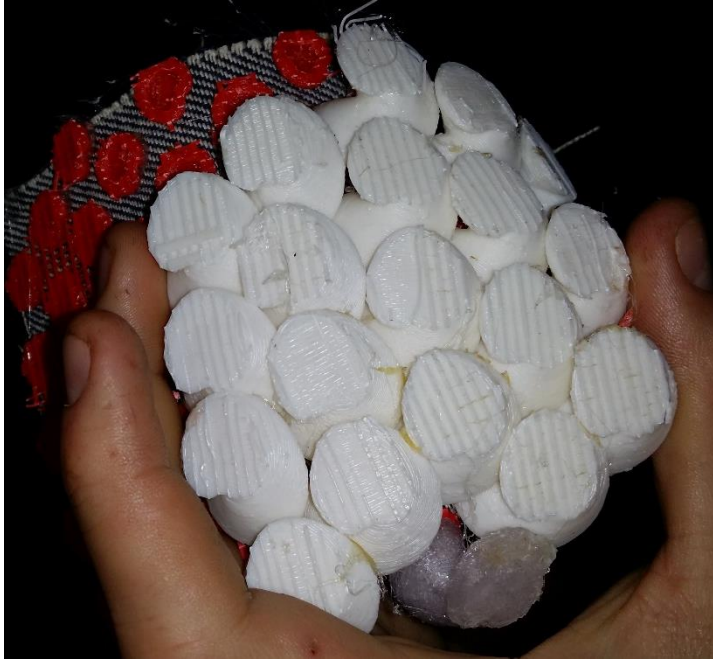
Figure 363: Uncompressed flared paradoxical-gear array (note its undesirable lack of initial freedom and initial synclastic curvature).
