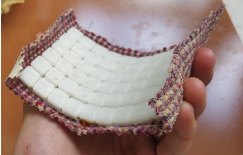
Figure 188: Tooth array on felted Nylon (at lockup point).
