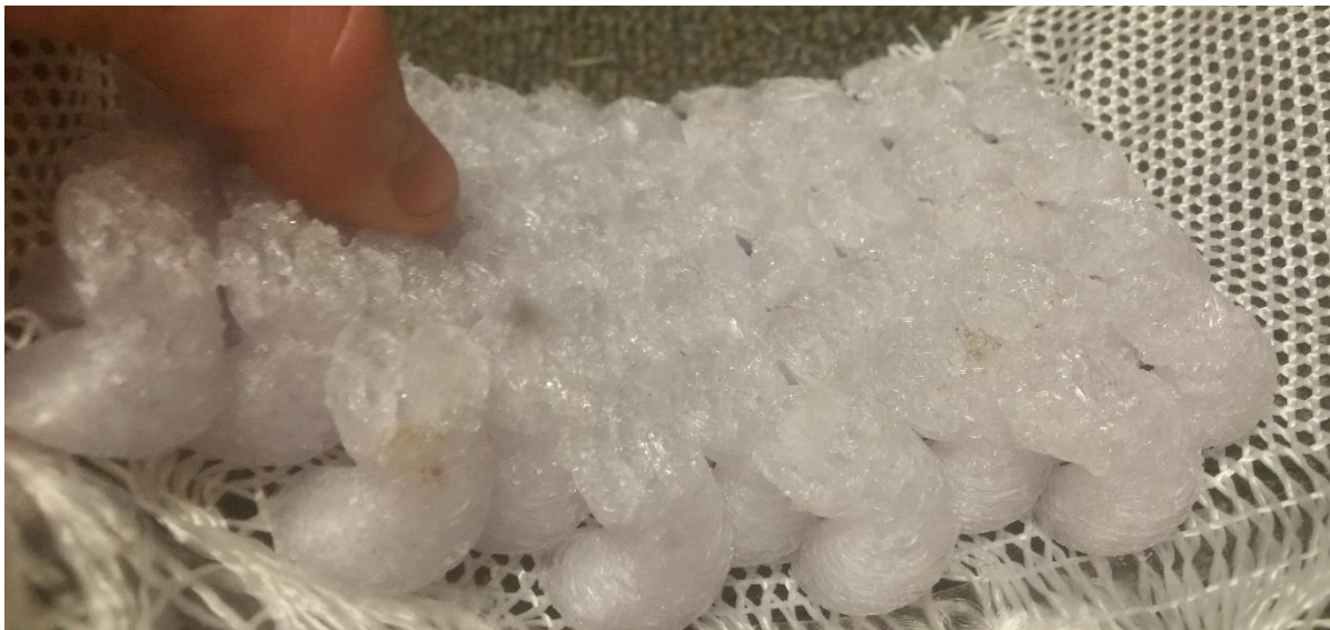
Figure 225: Lockup curvature in pure bending for paradoxical-gear-based array with .040" clearances (much higher than that seen with the 0.012"-clearance array).
