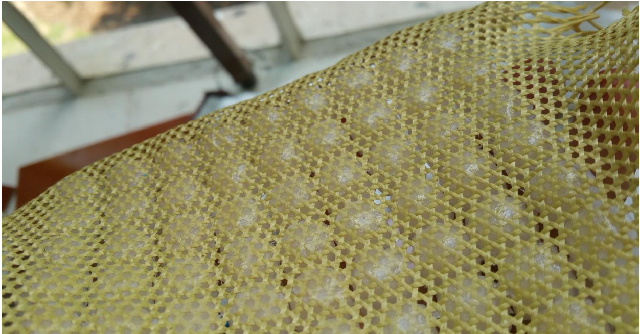
Figure 183: Tech-Bond structural cyanoacrylate (capable of bonding to nylons) was applied to the underside of this open weave at the bases of teeth, then activated for a more-secure bond than that offered by melting nylon to the fabric alone.
