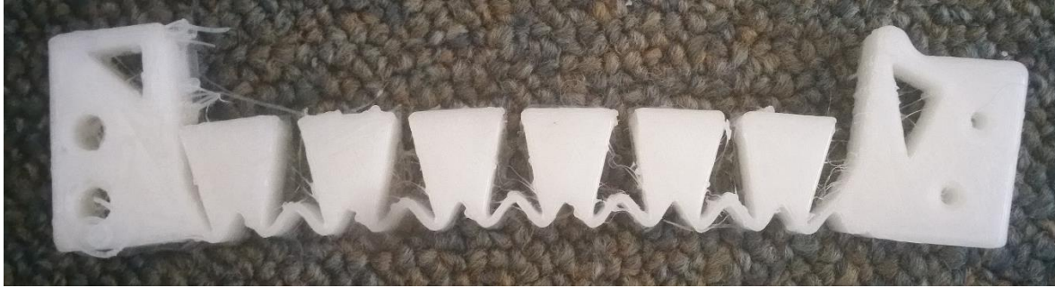
Figure 56: Undeformed comb with wavy backbone printed in elastomer-nylon alloy.
