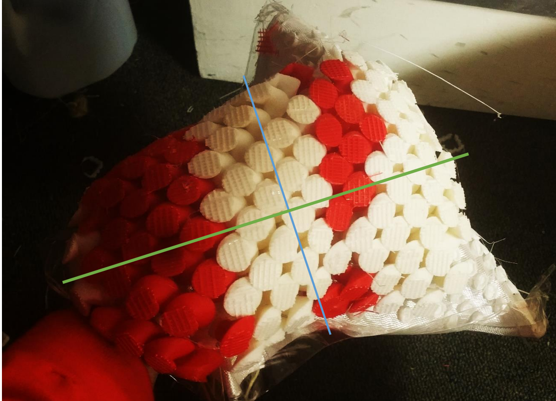
Figure 366: Bending the cylindrically pre-curved array to open up the initial curvature freely transforms the array into a cylindrically-curved array with the new cylindrical axis (shown in green) perpendicular to the original one (shown in blue). This transformation does not engage the backbone in tension and is thus very easy to accomplish.
