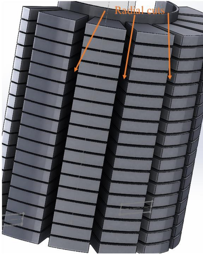
Figure 80: Reducing the pre-lockup bending stiffness of the annular comb teeth by radial interruptions.
