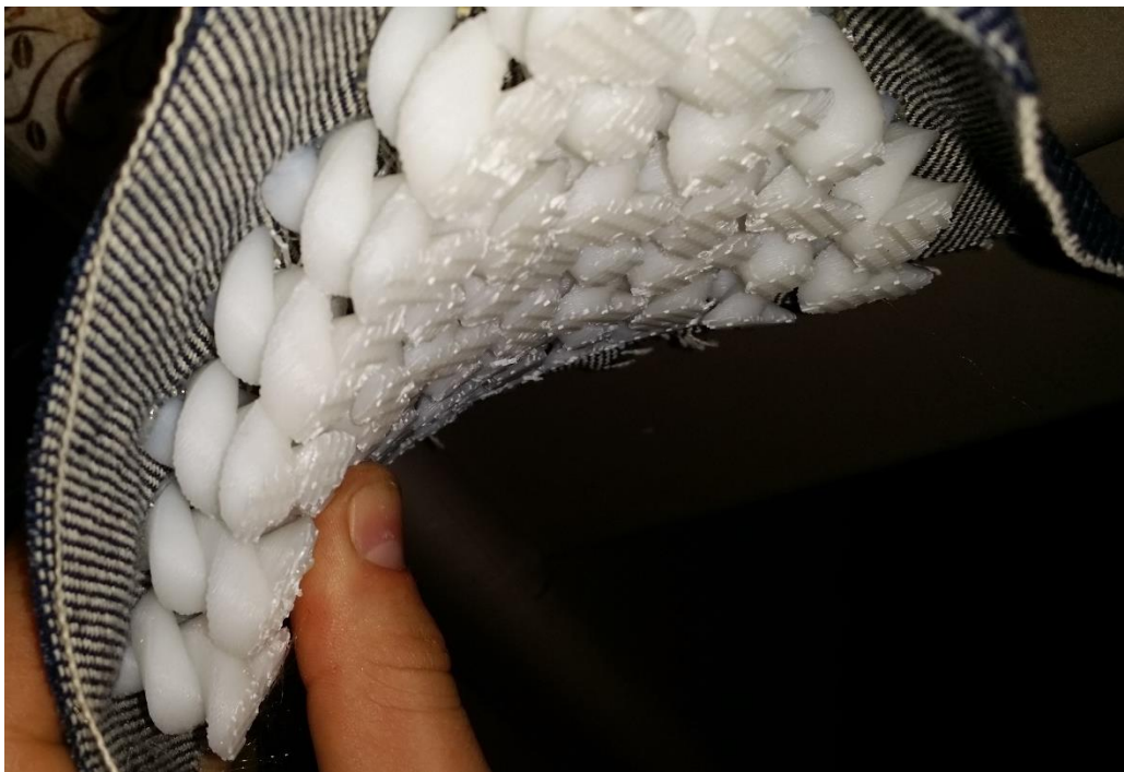
Figure 259: Lockup curvature for bending along a diagonal axis.
