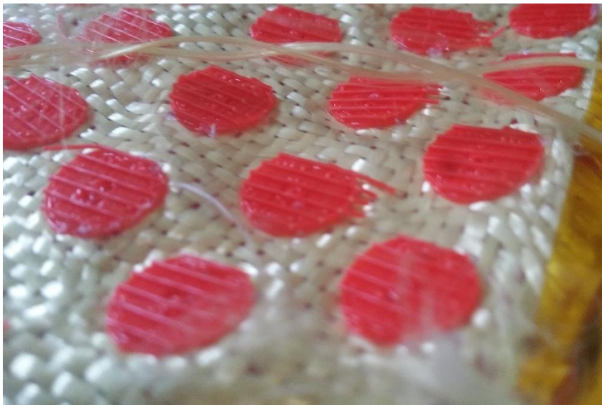
Figure 306: Plastic "rivets" (used to improve glue wetting of the Kevlar fabric) add some roughness to the back of the protective "sock".
