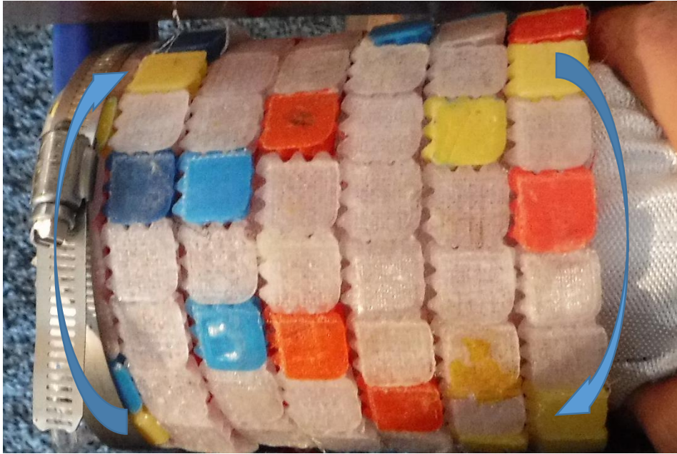
Figure 356: Maximum extent of torsional freedom at lockup, torsion in opposite direction (indicated with blue arrows).
