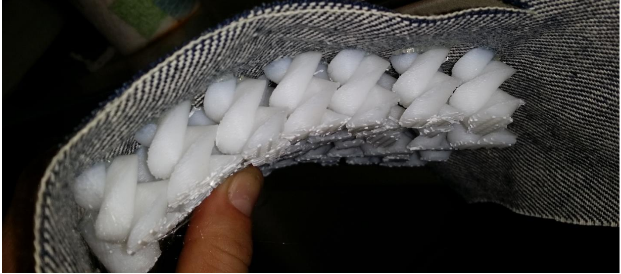
Figure 258: Lockup curvature for bending about a horizontal axis.
