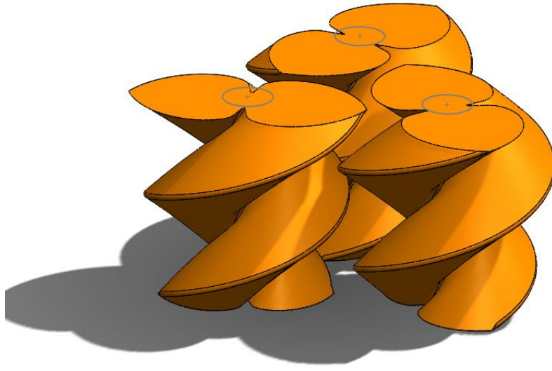
Figure 257: Two-toothed paradoxical gears in triangular/hexagonal packing.
