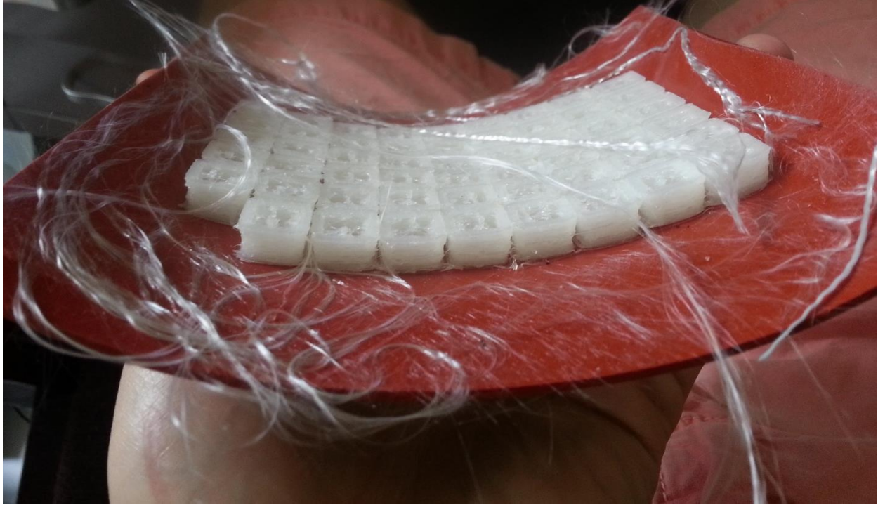
Figure 189: Silicone-backbone comb array. At the subjective beginning of lockup (but the stiffening-up effect was so small as to make this difficult to detect).
