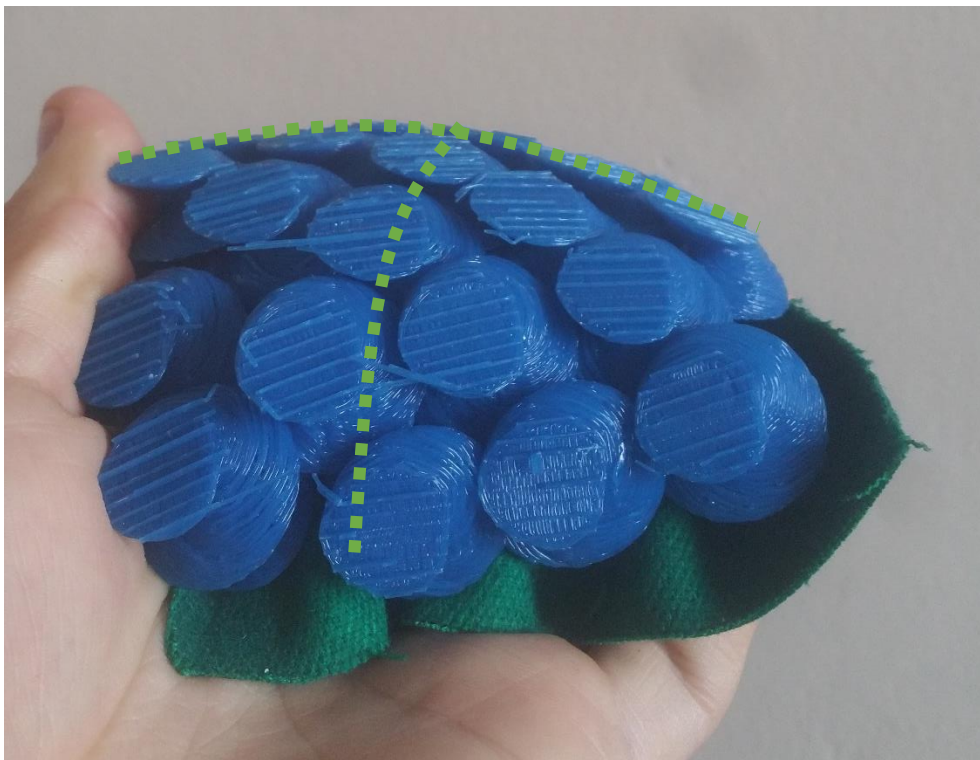
Figure 243: Compressing the array along a specific axis produces sympathetic curvature in two directions, yielding a synclastic or spherical double curvature. Compare this curvature to the merely cylindrical sympathetic deformation of the array based on the single-rotated paradoxical-gear tooth.
