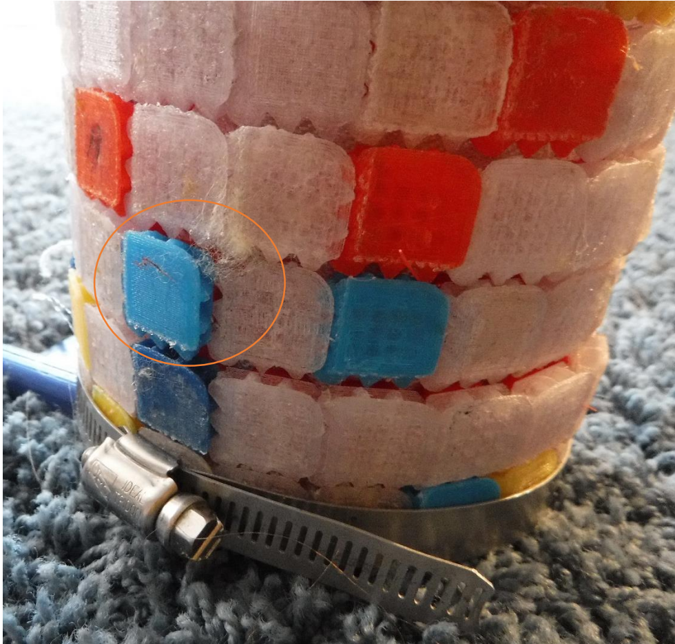
Figure 354: The light blue tooth circled in orange has slid past its neighbors to the right and above it, preventing it from normal engagement with these two teeth.
