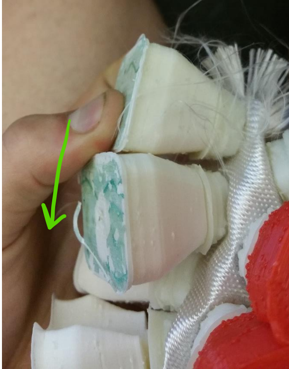
Figure 333: Drooping behavior of long and heavy teeth (note how their normals tend to be angled somewhat downwards from the average normal direction of the fabric). The direction of gravity is drawn in green.
