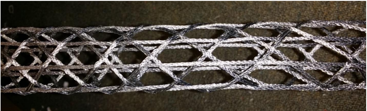
Figure 27: A true-triaxial weave that is quite stiff in bending thanks to its axial yarns.
