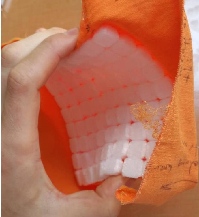
Figure 195: Lockup curvature of the CPE-backbone array when bent along the compliant direction.
