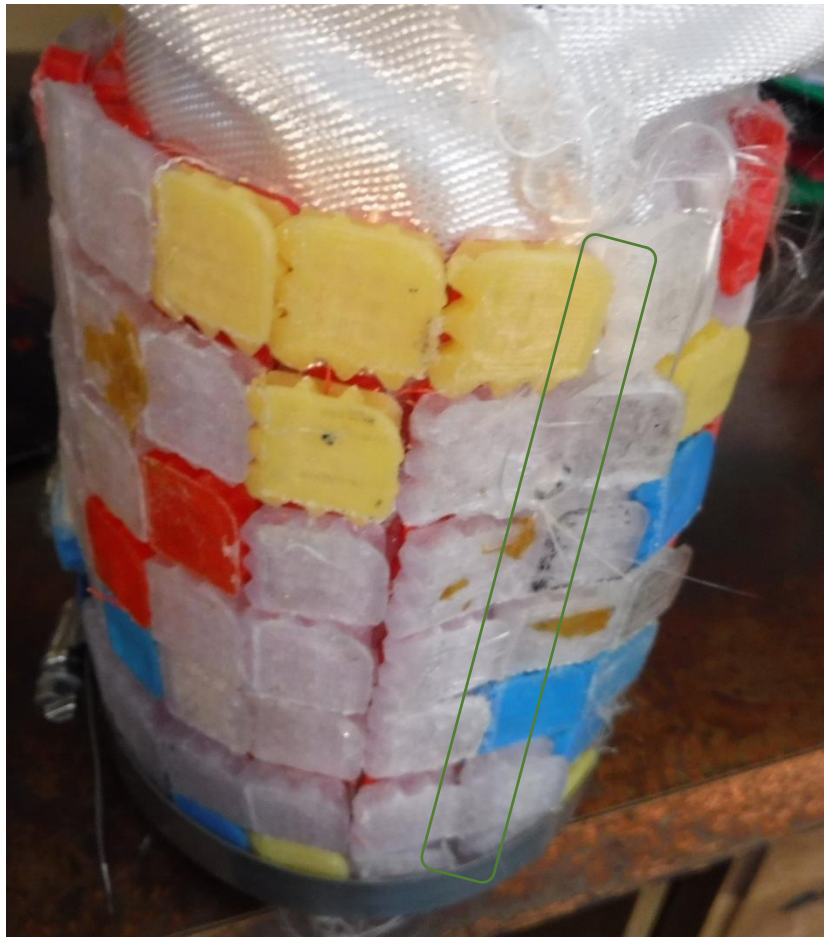
Figure 348: The region indicated with the green rectangle is the imperfect seam in the array. It did not seem to impair the overall function of the array, even though it saw teeth angled improperly thanks to improper spacing.
