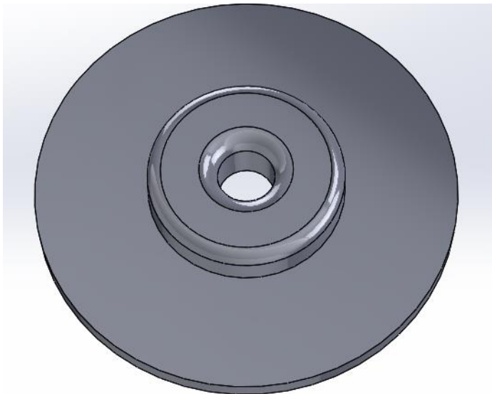
Figure 300: Rivet modified with hole in it to allow activating chemical to flow through and activate cyanoacrylate.
