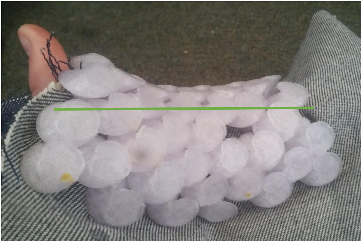
Figure 222: Sympathetic cylindrical deformation of paradoxical-gear-based array with .012" clearances in compression along the axis shown in green (plus a small amount of bending).
