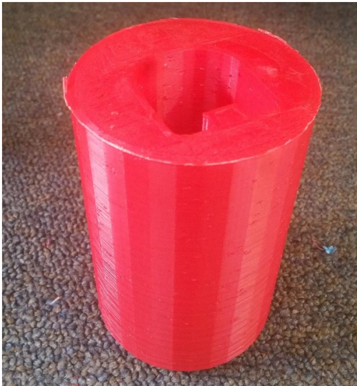
Figure 304: This part slid over the main arm of the “leg” (hence the oddly-shaped T-slot through the cylindrical axis) to properly contact the “sock”.
