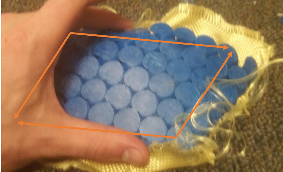
Figure 237: Thanks to the plain weave of the fabric (which gives it high bias compliance) and the low contact area between tooth bases and fabric, the overall structure is quite compliant in shear, up to the point shown.
