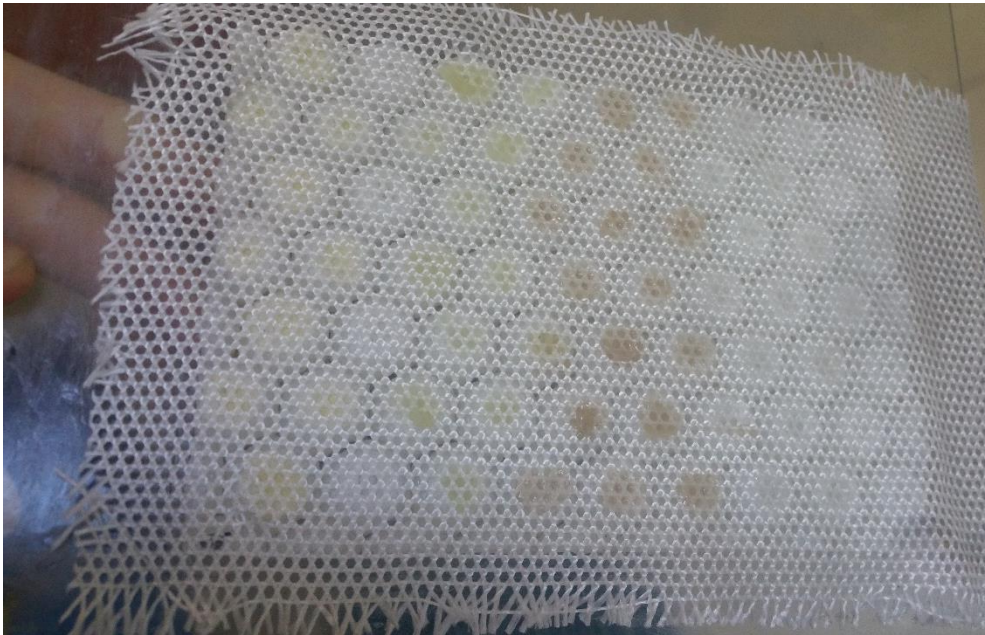
Figure 375: Showing an open weave with epoxy added to the outside of the fabric for improved bonding between the adhesive zone and the fabric.
