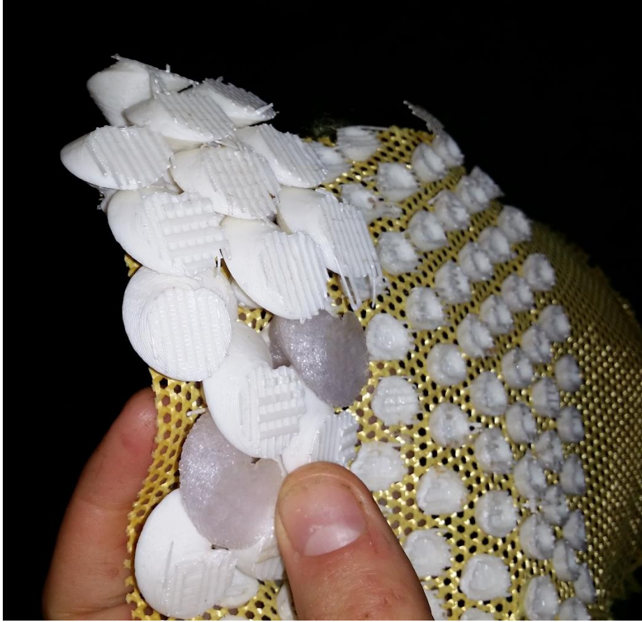
Figure 360: First iteration of flared paradoxical-gear array; note the strange tiling of base parts and corresponding (undesirable) initial synclastic curvature of the array. The array also had very little initial freedom.
