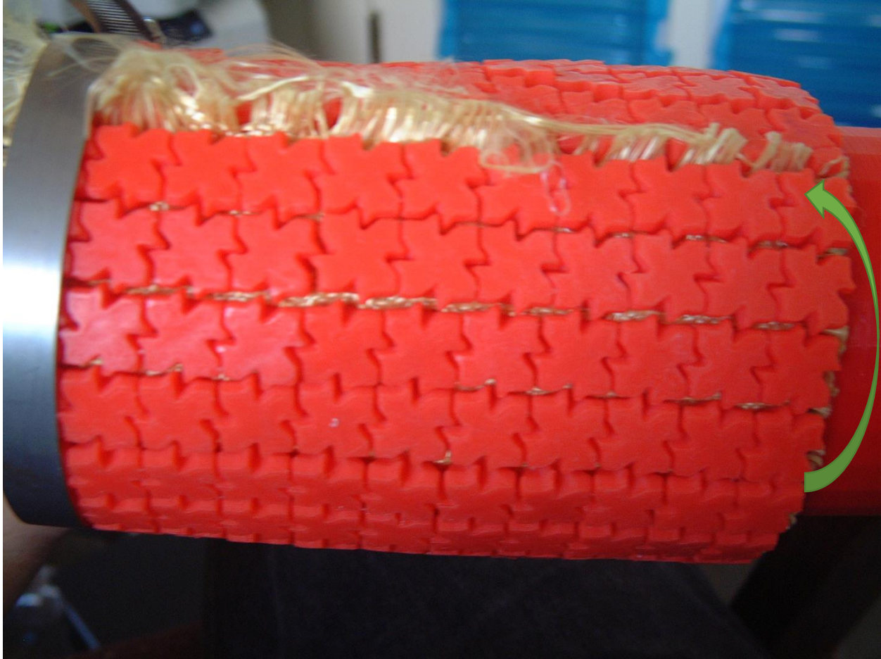
Figure 312: Side view of array mounted on test fixture; the direction of “leg” rotation is shown with the green arrow. (This is the same view but opposite direction of leg rotation from the previous figure).
