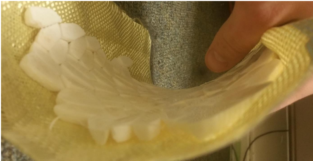
Figure 270: Post-lockup curvature of the P15 pentagon array at another angle.
