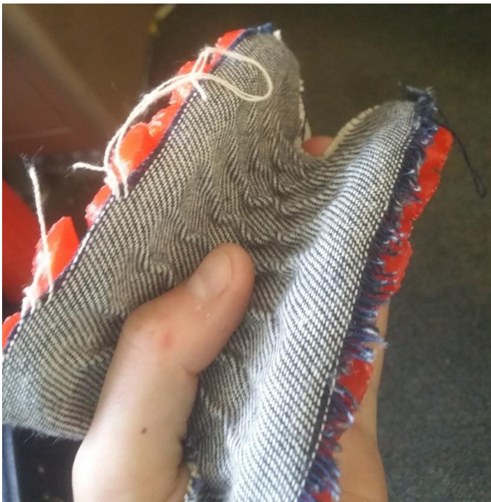
Figure 229: Bottom view of 80%-width-scaled HCP paradoxical-gear array in compression (with coupled cylindrical deformation). Note that this curvature is stronger than that for the unscaled HCP paradoxical-gear array.
