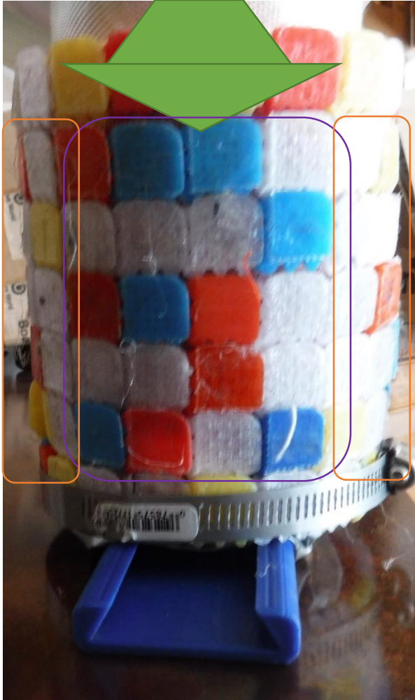
Figure 353: Fabric-backed array of FTASF teeth on test fixture, rotated until lockup, side view. The rotation direction is out of the page, as shown with a green arrow. Shearing of the array occurs in the regions circled in orange (this area saw lockup thanks to the anti-slide features of the teeth), and bending lockup of the array occurs in the region circled in purple.
