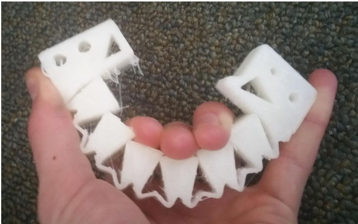
Figure 58: Subjecting the comb to significant bending moment after initial tooth touching brings significant tensile stretching of the backbone, which, thanks both to its wavy geometry and the low bulk stiffness of the elastomer-nylon alloy in which it was
