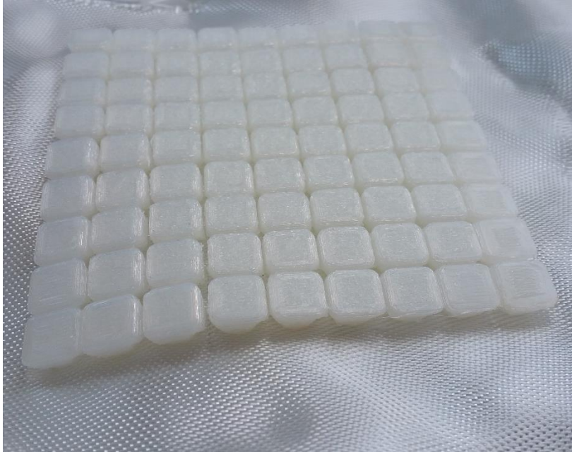
Figure 184: Nylon tooth array on woven ultrafine fiberglass fabric--relaxed.
