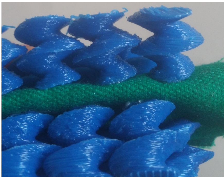
Figure 242: Closeup of several printed, double-rotated teeth showing fairly poor print quality.
