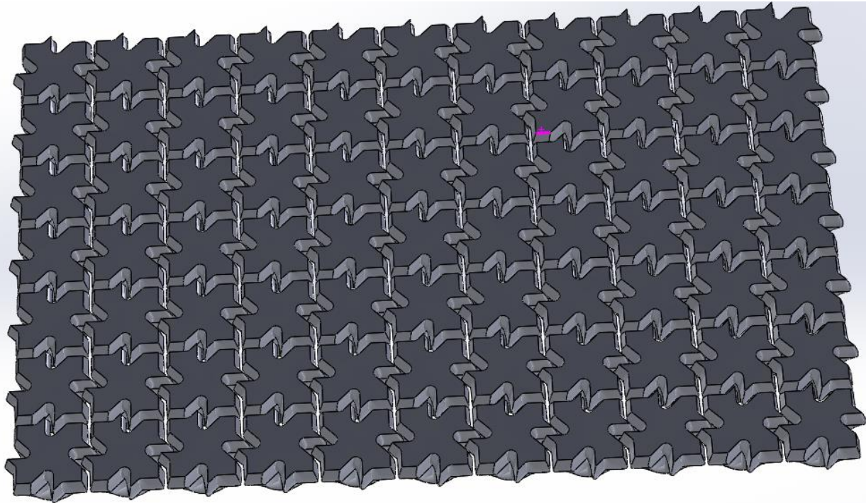
Figure 212: Full array of convex-concave square-like teeth.
