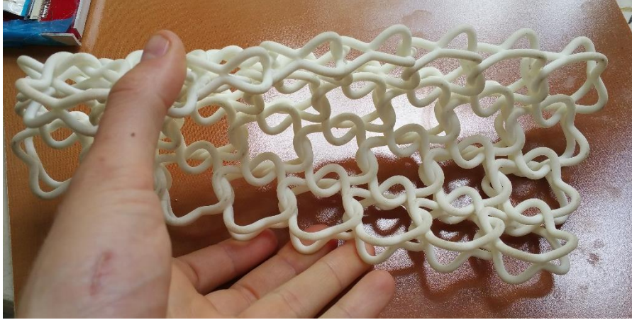
Figure 16: Bending the fabric until resistance ("lock-up") is encountered.
