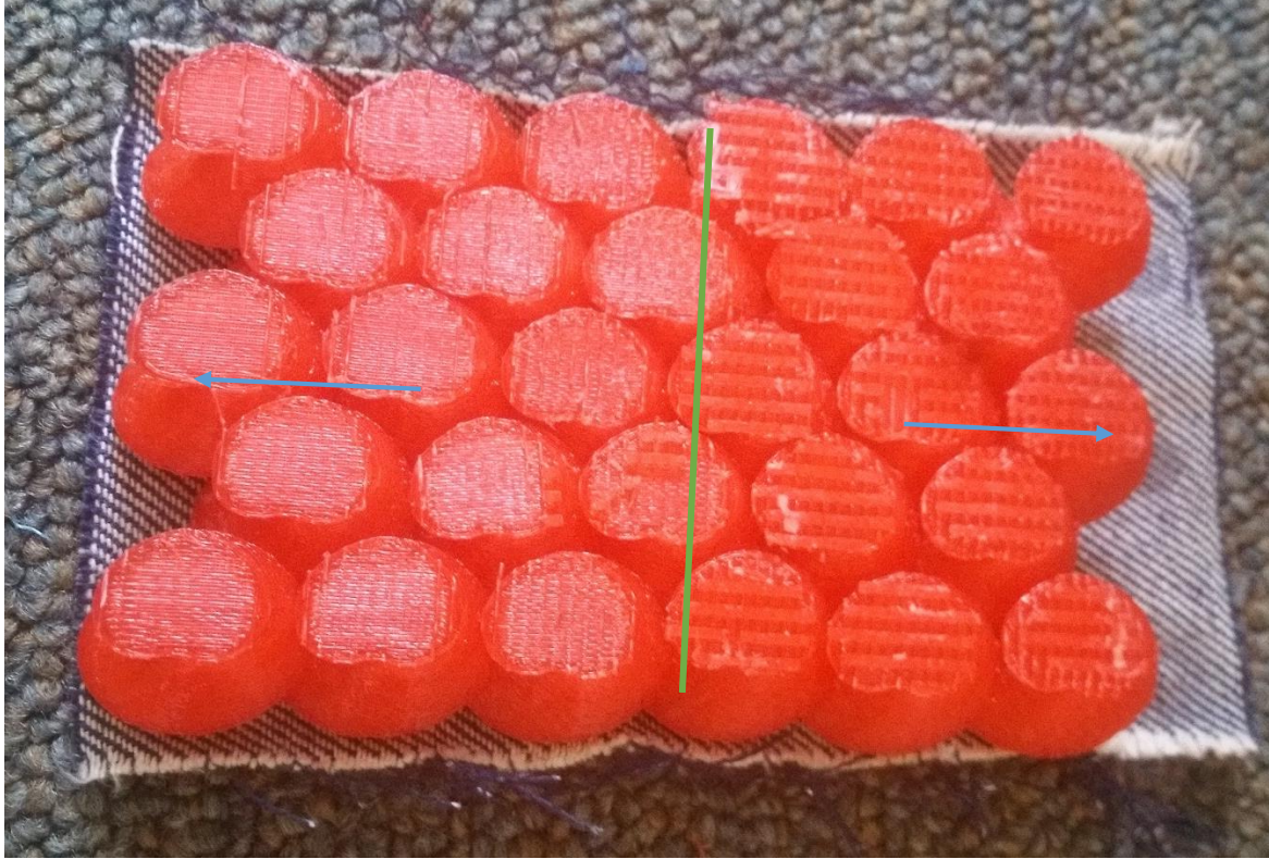
Figure 231: HCP paradoxical-gear tooth array, scaled outwards (along the blue arrows) to 125% of its width. The axis along which compression results in coupled cylindrical deformation is shown in green.
