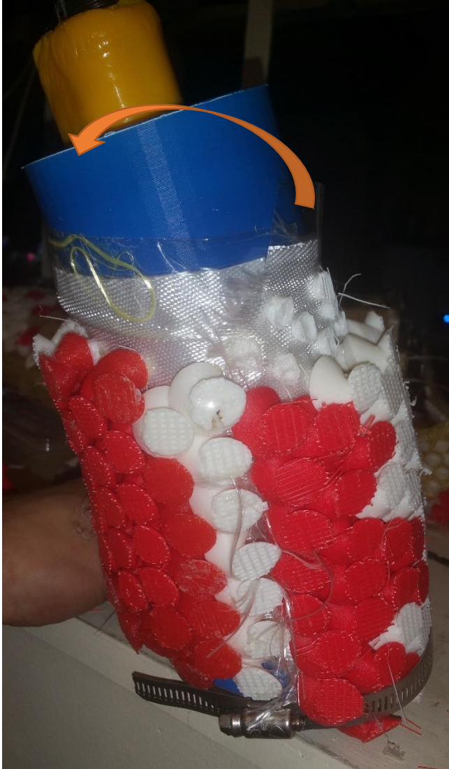
Figure 369: Orthogonal view of test fixture fitted with pre-curved array, bent until lockup. The orange arrow shows the direction of bending.
