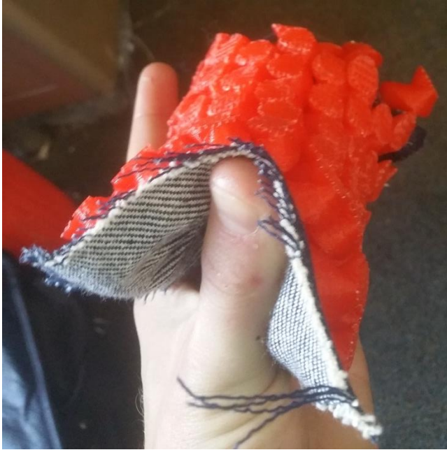
Figure 228: Top view of 80%-width-scaled HCP paradoxical-gear array in compression (with coupled cylindrical deformation). Note that this curvature is stronger than that for the unscaled HCP paradoxical-gear array.
