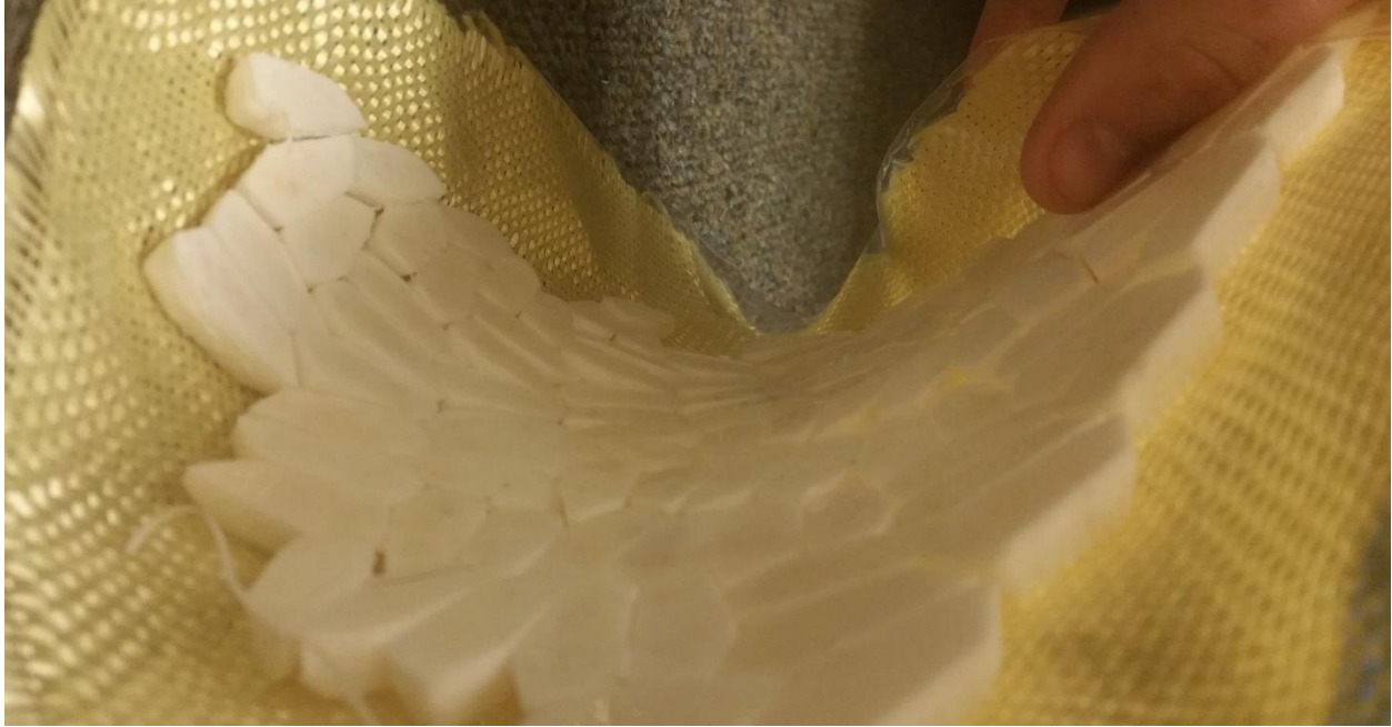
Figure 269: Post-lockup curvature of the P15 pentagon array at another angle.
