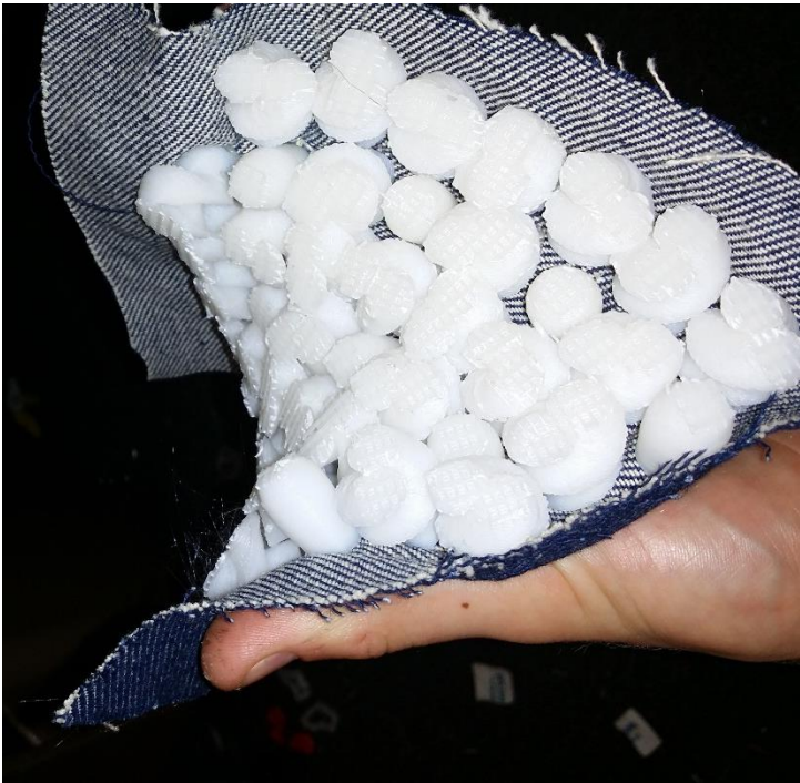
Figure 261: Synthetic saddle-shaped curvature from compressing along a diagonal.
