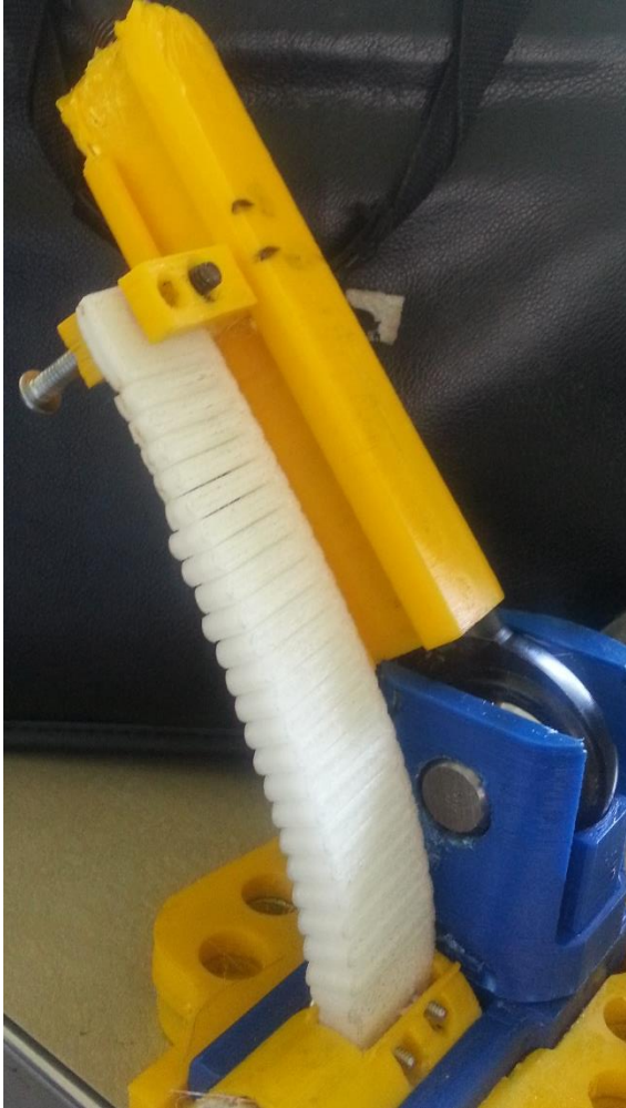
Figure 46: Simulated plantar/dorsiflexion sees greatly-increased bending stiffness throughout the entire range as the comb's backbone is quite thick in this direction. Obviously, this is unsatisfactory.
