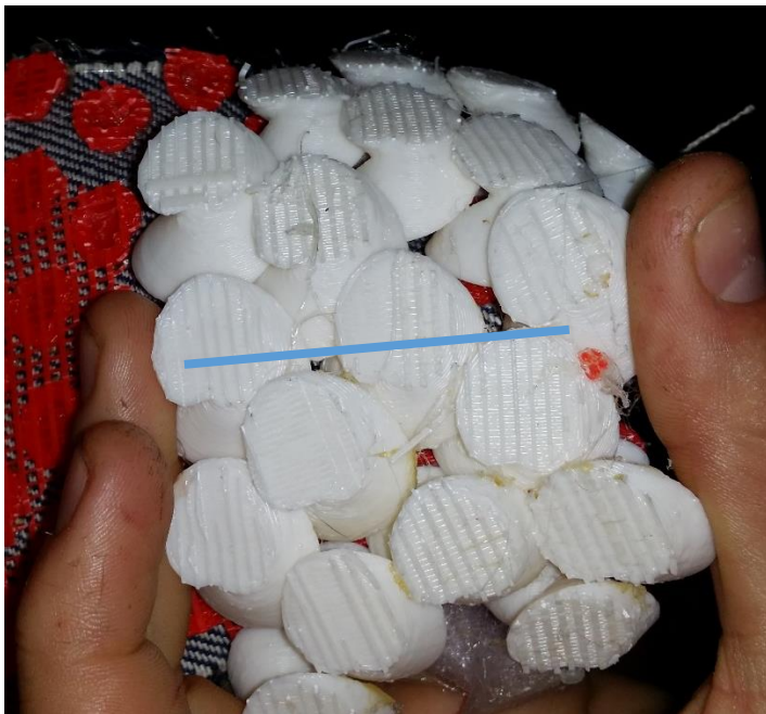
Figure 364: Compressing the array about the axis shown in blue produces sympathetic cylindrical deformation, though this axis is perpendicular to the one expected based on the behavior of planar arrays of unflared teeth.
