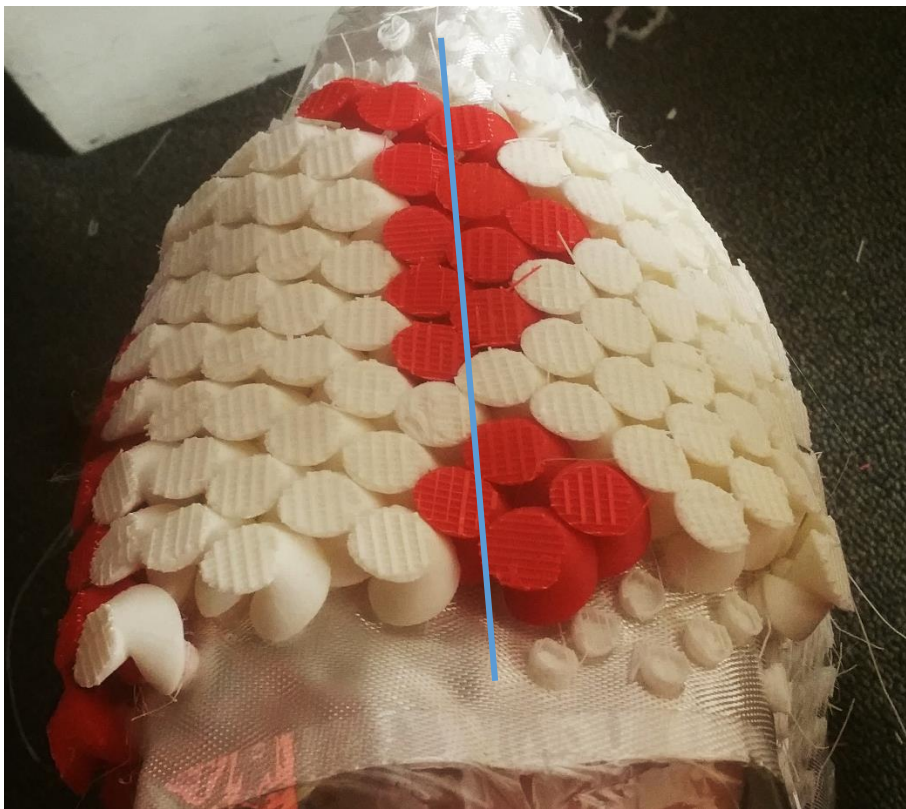
Figure 365: Pre-curved array (of the tooth configuration discussed above) in its neutral, cylindrical shape, with the cylindrical axis shown with a blue line.
