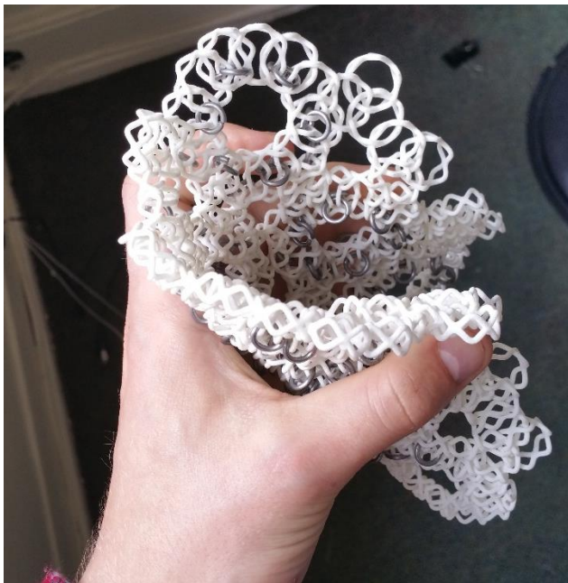
Figure 19: Same chainmail weave as above, bent to the maximum kinematic extent about an axis parallel to the horizontal.
