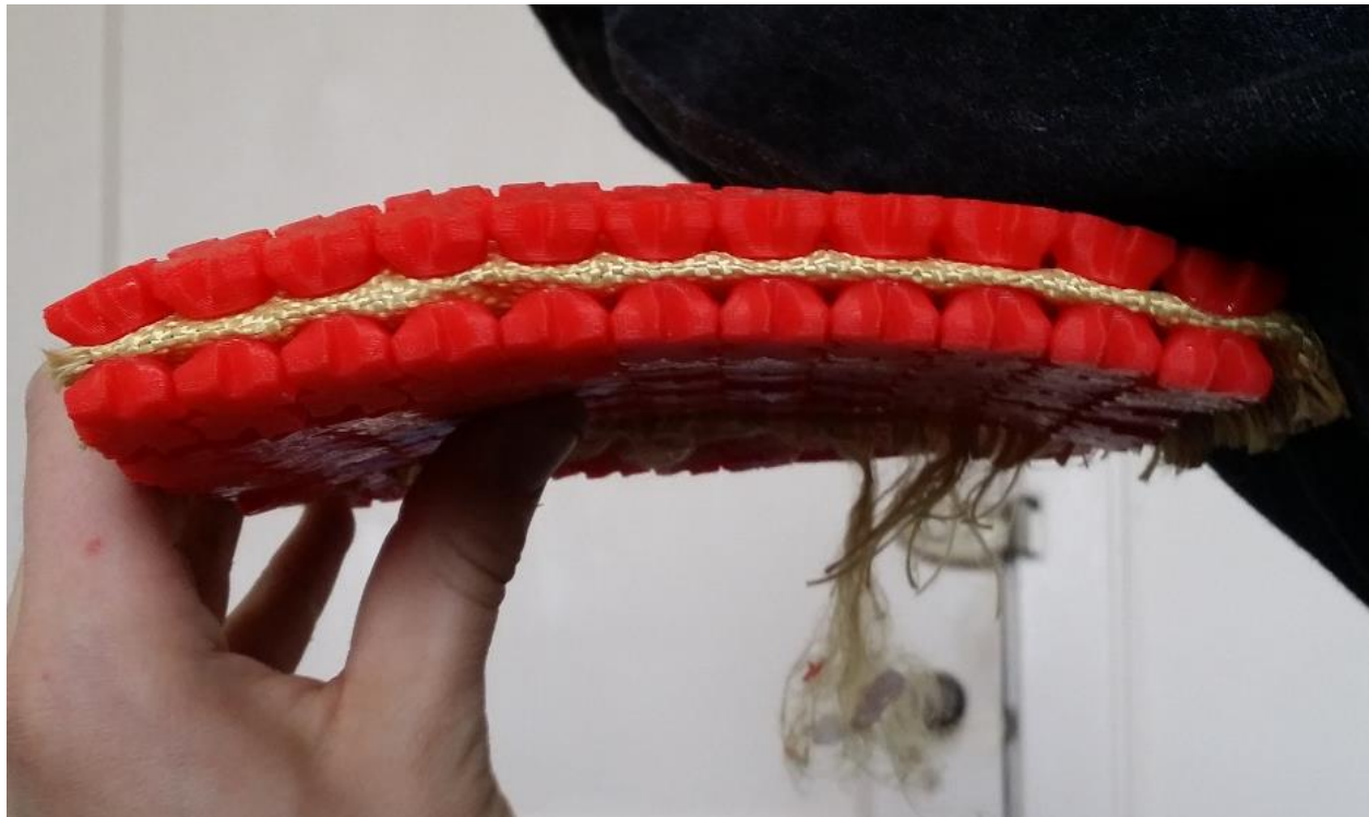
Figure 310: In planar bending, the structure had much more freedom before lockup than it did in cylindrical conformation.
