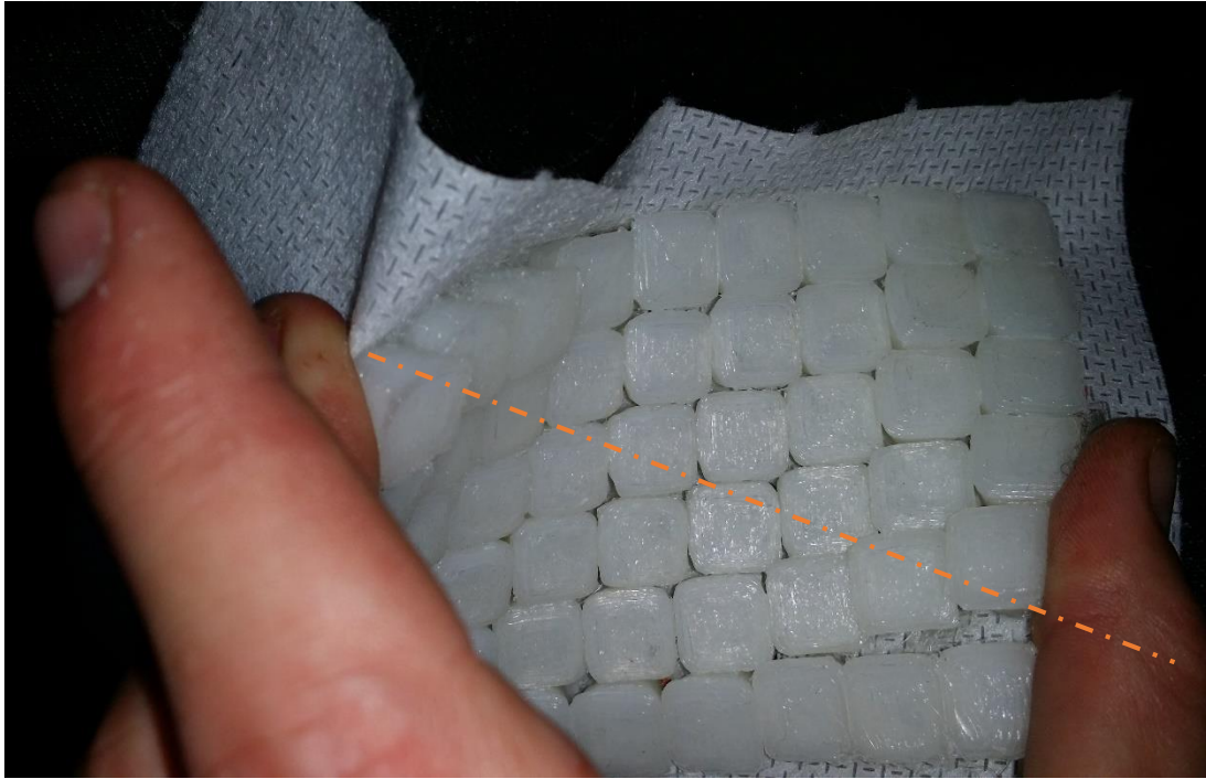
Figure 206: When a square array is bent along an axis not parallel to the contact normals between teeth (i.e. at an angle that is not an integer multiple of 90^\circ for a square array), its teeth see sliding past each other, and much more curvature can be achieved before lockup than could be achieved when the array is bent along an angle that is a multiple of 90^\circ .
