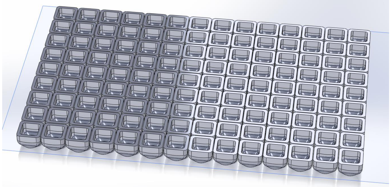
Figure 293: Hollow tooth array to be printed on fabric and then reinforced with metal, composite material, or, at the very least, solid resin.
