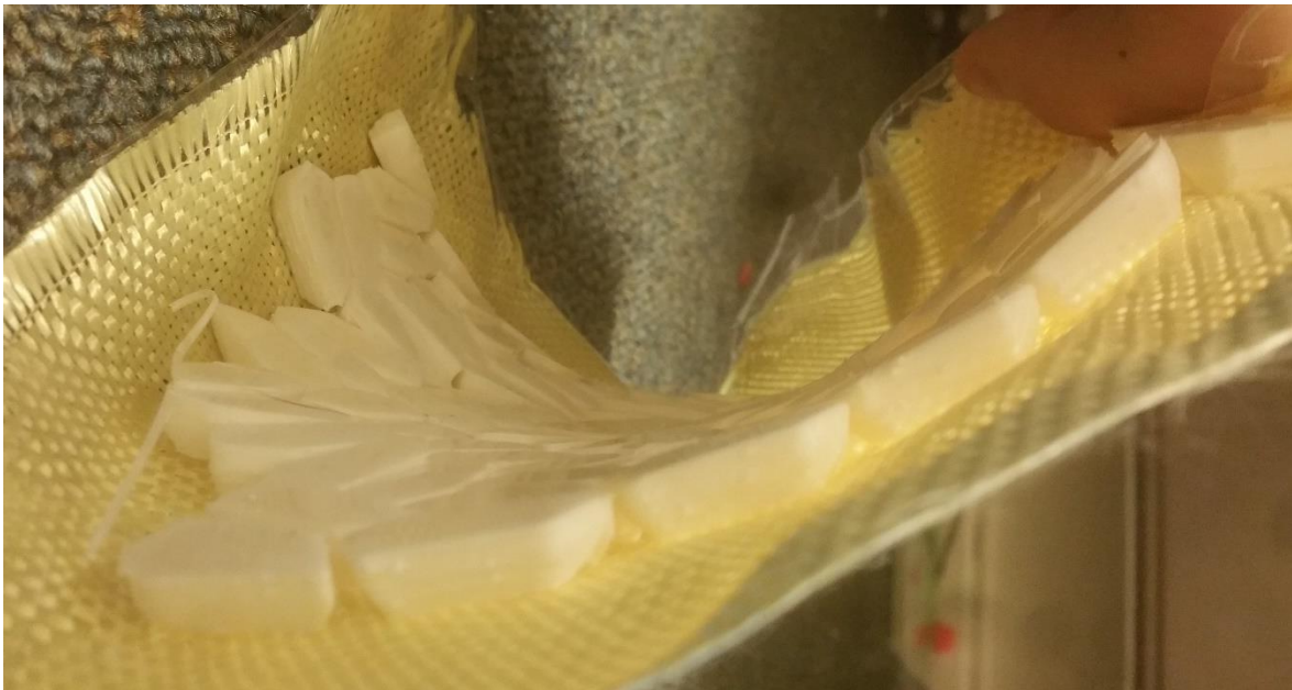
Figure 268: Post-lockup curvature of the P15 pentagon array at another angle.
