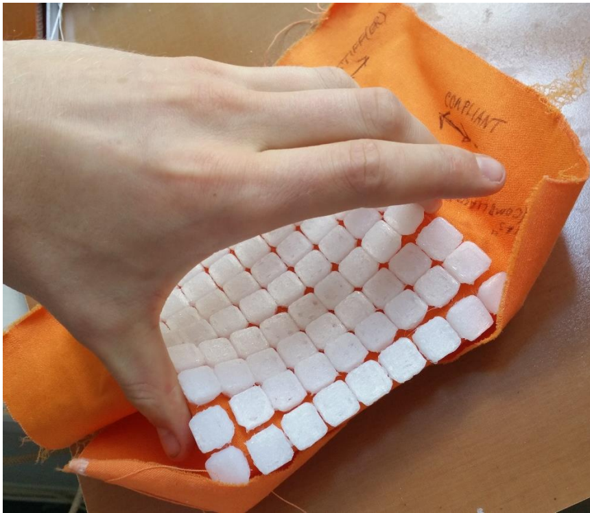
Figure 196: Lockup curvature of the CPE-backbone array when bent along the stiffest direction.
