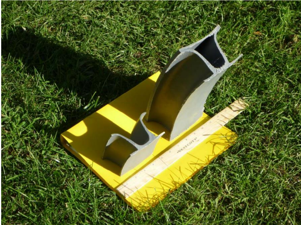
Figure 2-10: Dual-Wall and Triple-Wall Profiles of ADS Pipes (Hoppe 2011)
