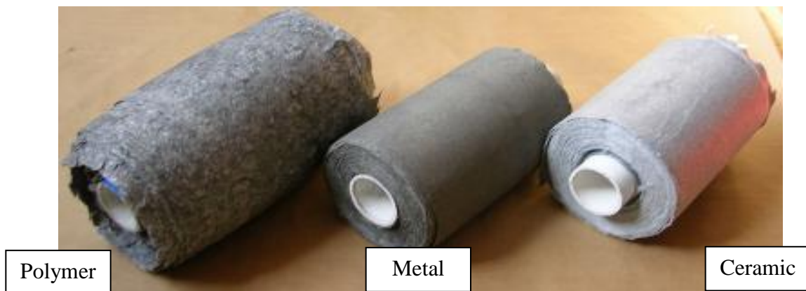
Figure 0-12 Microfibrinous media (polymer, metal and ceramic)
