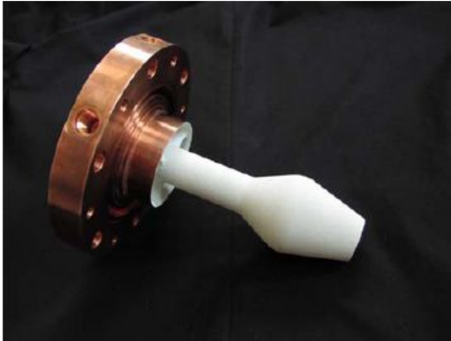
Figure 3.8: Center Body used in the Experimental Analysis (source: Anderson[21] et al. (2003)).
