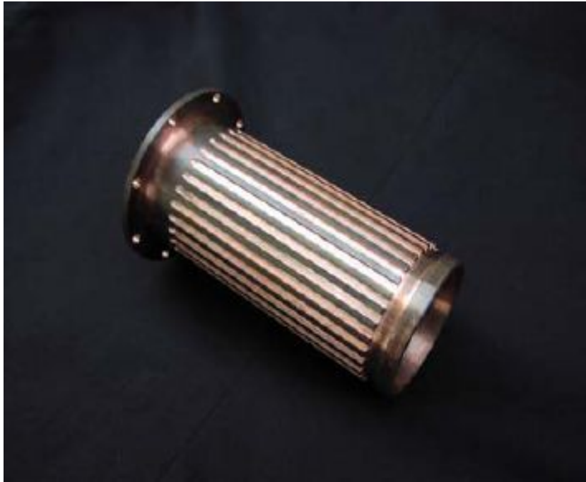
Figure 2.7: Undeformed OFHC Copper Chamber Liner (source: Anderson [21] (2003)).
