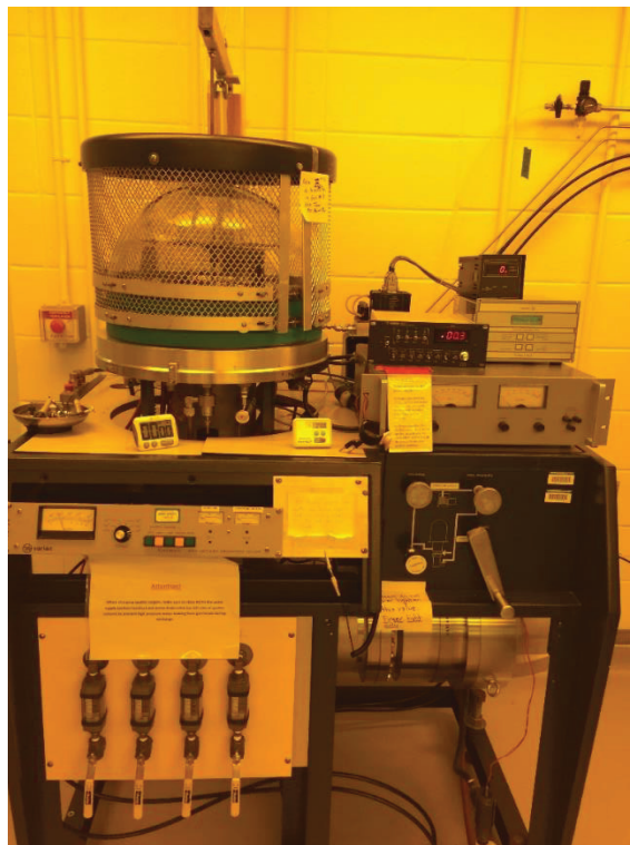
Figure 4.4-9: DC Magnetron sputtering system for the metallic thin film.
